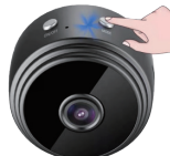
Press and hold the MODE button to reset the device
