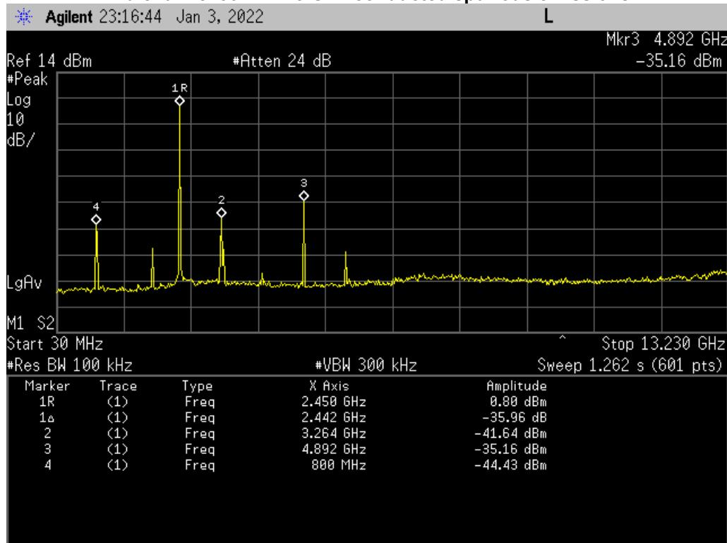
**High channel 30MHz-13 GHz conducted spurious emissions**
