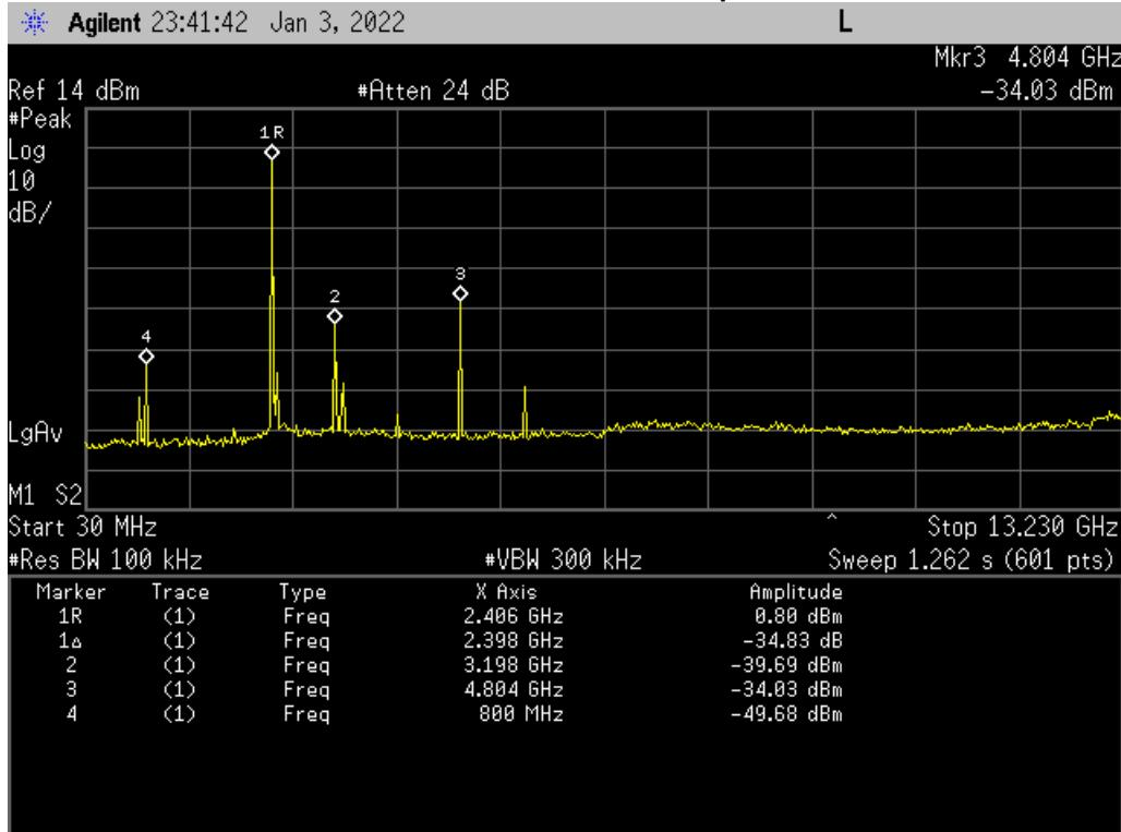
**Mid channel 30MHz-13 GHz conducted spurious emissions**
