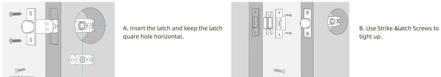
A. Insert the latch and keep the latch square hole horizontal.
