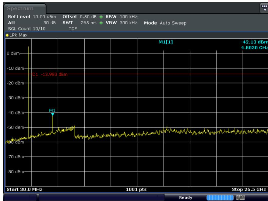
**B.1. Middle Ch. (2 440 MHz) Spurious emissions**
