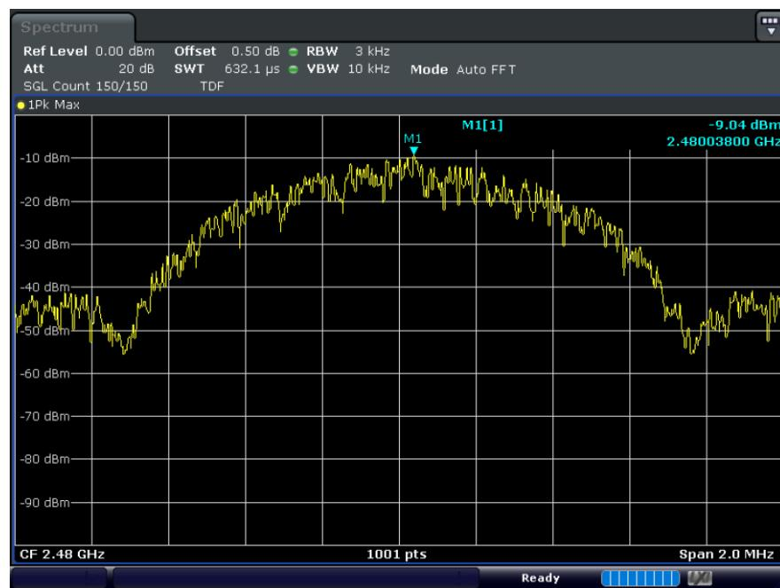
**Test mode : Bluetooth LE (2 Mbps)****A. Lowest Ch. (2.402 MHz)**
