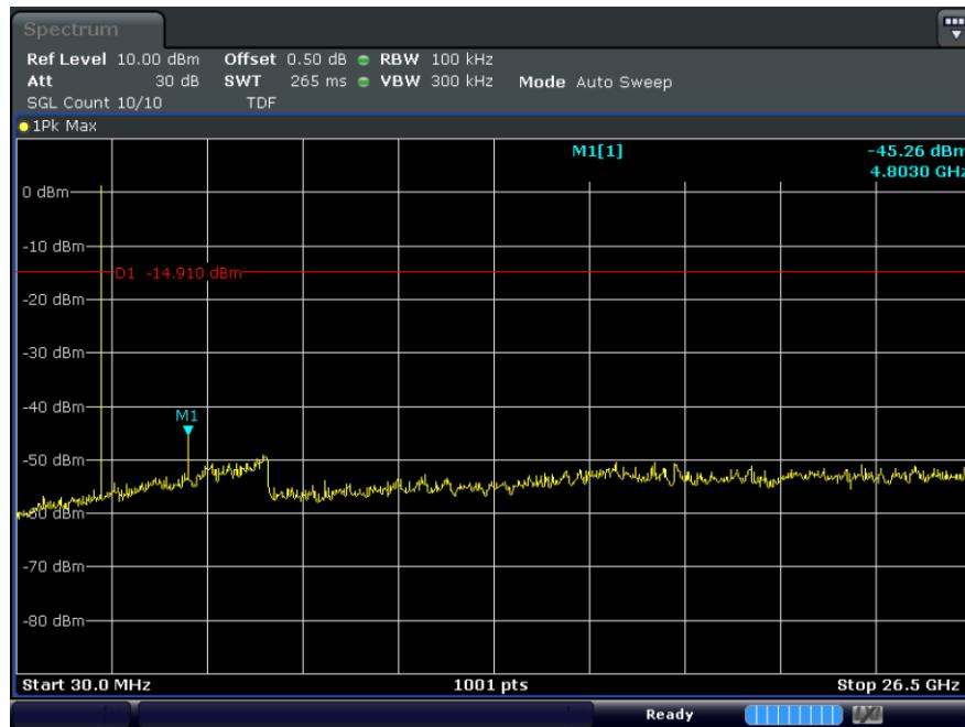
**B.1. Middle Ch. (2 440 MHz) Spurious emissions**
