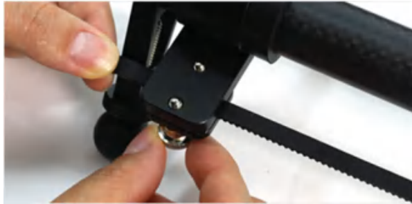
1 Insert the belt and tighten with two knobs.
