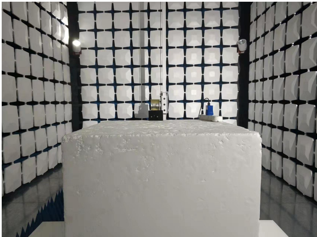
Above 1GHz for radiated emission test setup
