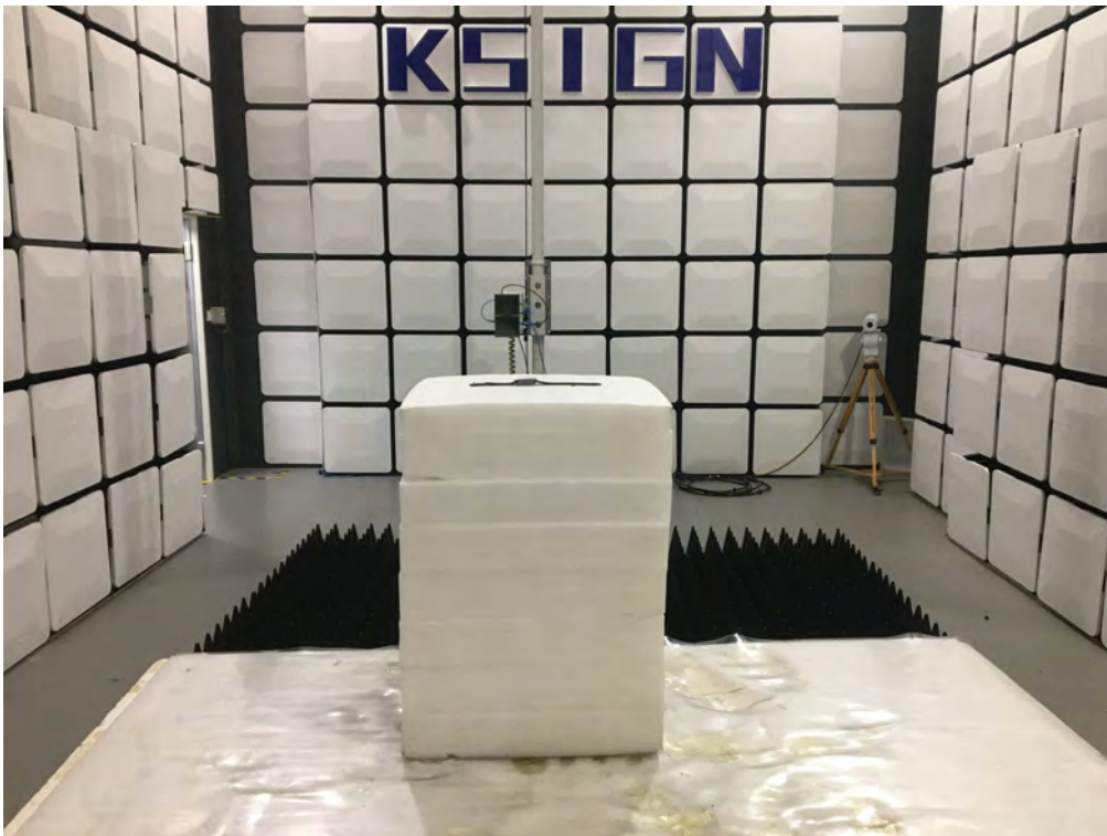
Radiated Measurement (Above 1GHz)
