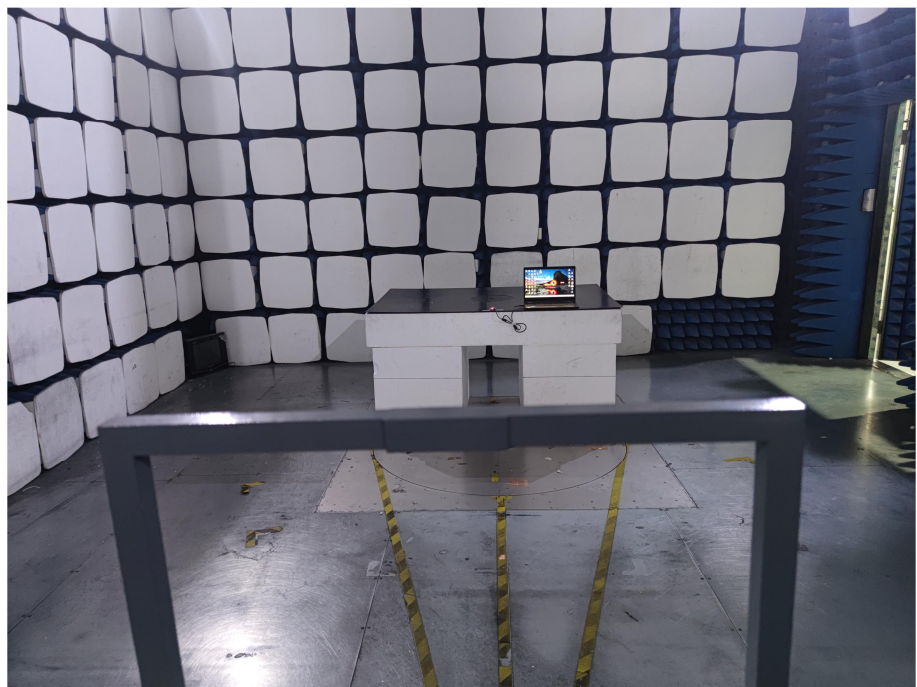
Radiation Emission Test Setup (Below 30MHz)
