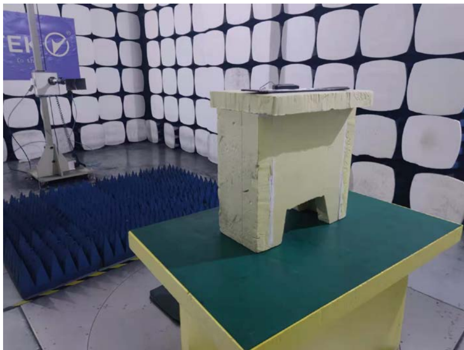
Spurious Emission Test Setup (Above 1GHz)
