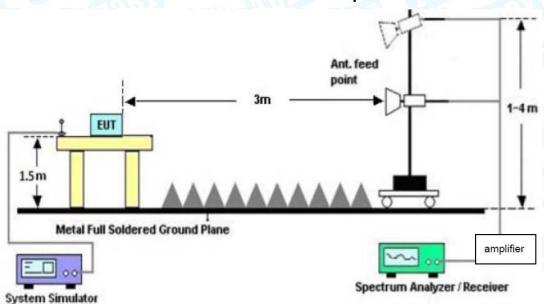
**Above 1GHz Test Setup**
