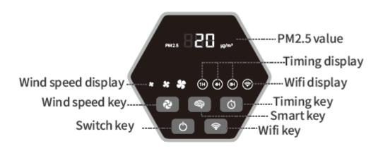
**Wind speed key:** in the power on state, short press the wind speed key, the panel wind speed LED light is on, the intelligent LED light is off, the buzzer rings, the wind speed gear changes by pressing "1-2-3" cycle, in the intelligent mode, press thewind speed key to exit the intelligent mode, and the wind speed is in the next gear of the wind speed in the intelligent mode.
