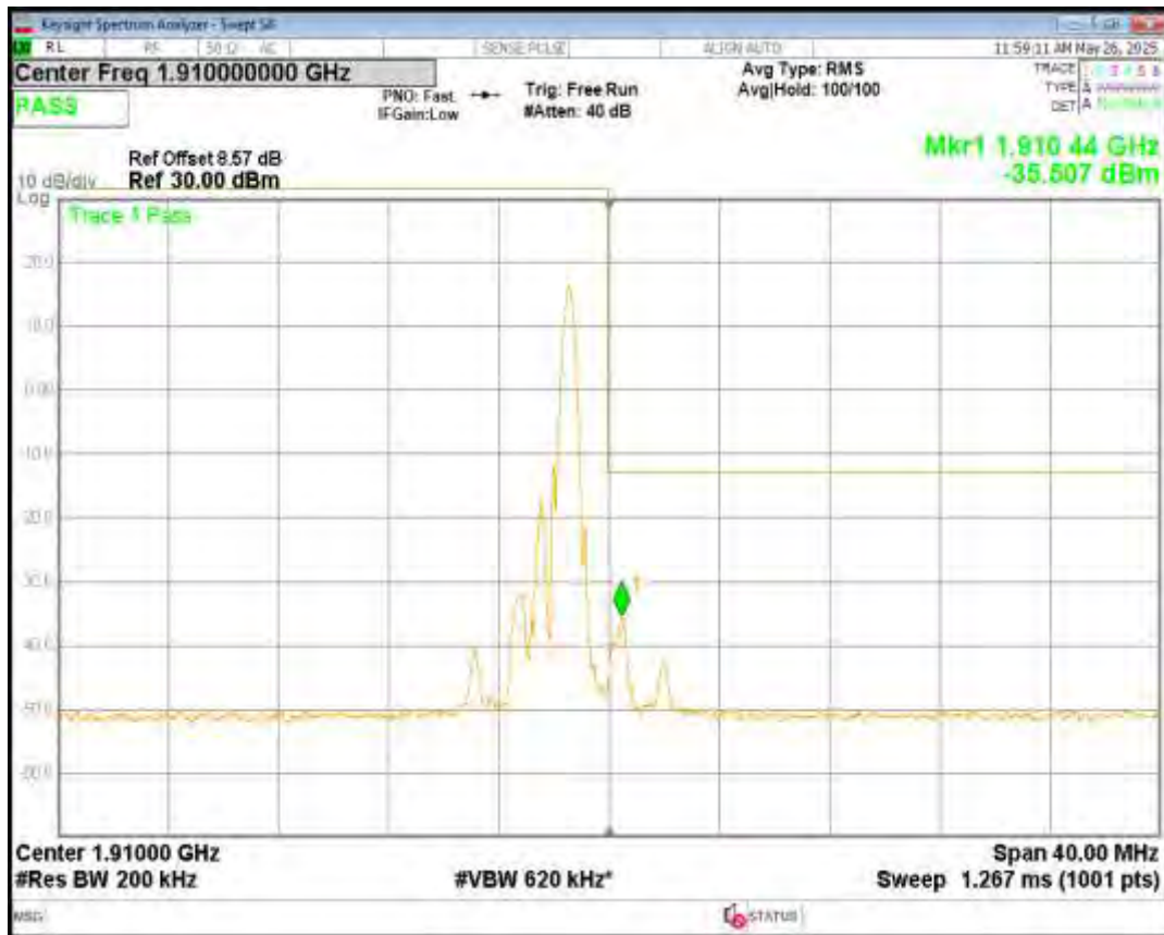
Band2 16QAM BW=20MHz Channel=19100 RB Size=5 Position=#Max NB Index=15
