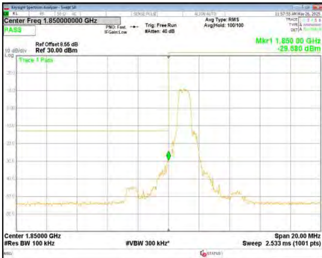
Band2 QPSK BW=10MHz Channel=19150 RB Size=1 Position=#Max NB Index=7
