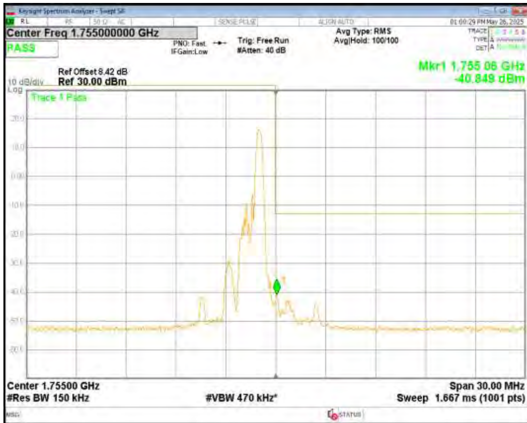
Band4 QPSK BW=15MHz Channel=20325 RB Size=6 Position=#Max NB Index=11
