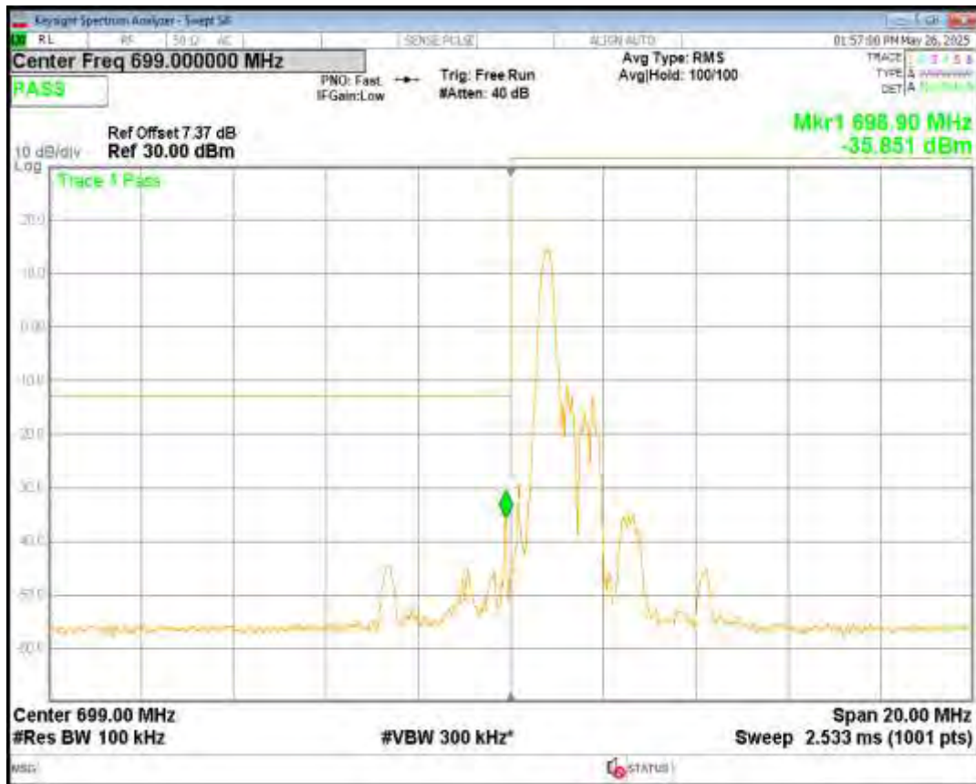
Band12 QPSK BW=10MHz Channel=23060 RB Size=4 Position=#0 NB Index=0
