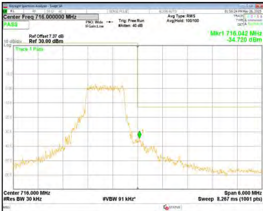
Band12 16QAM BW=5MHz Channel=23035 RB Size=1 Position=#0 NB Index=0
