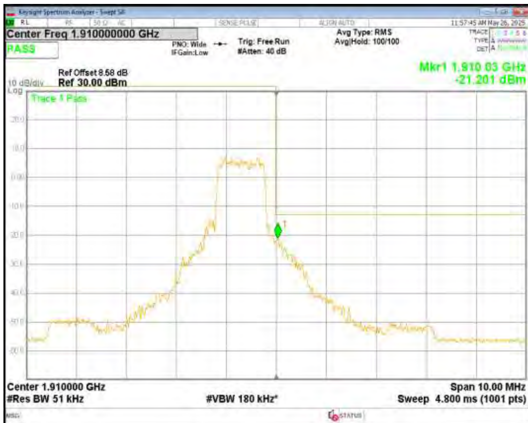
Band2 QPSK BW=1.4MHz Channel=18607 RB Size=1 Position=#0 NB Index=0
