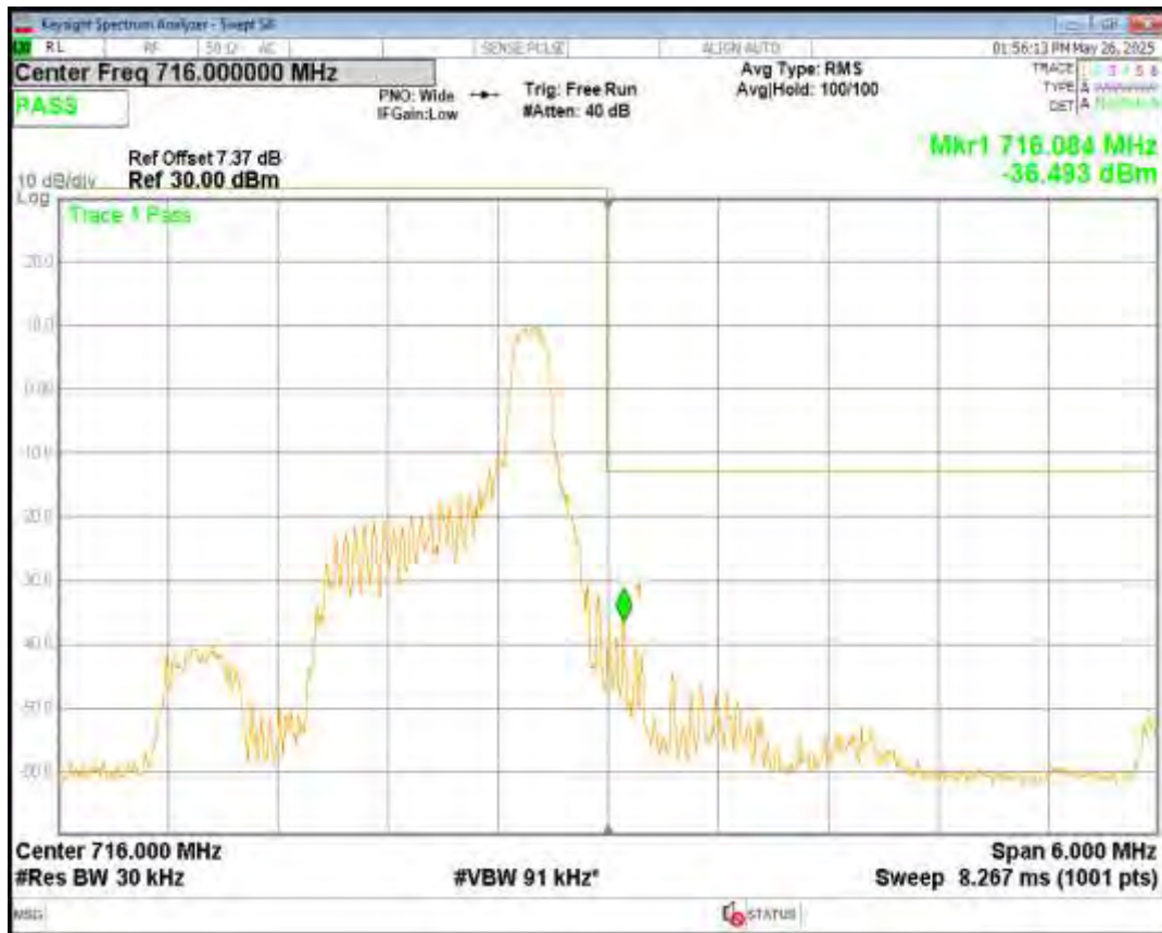
Band12 QPSK BW=3MHz Channel=23165 RB Size=6 Position=#Max NB Index=1
