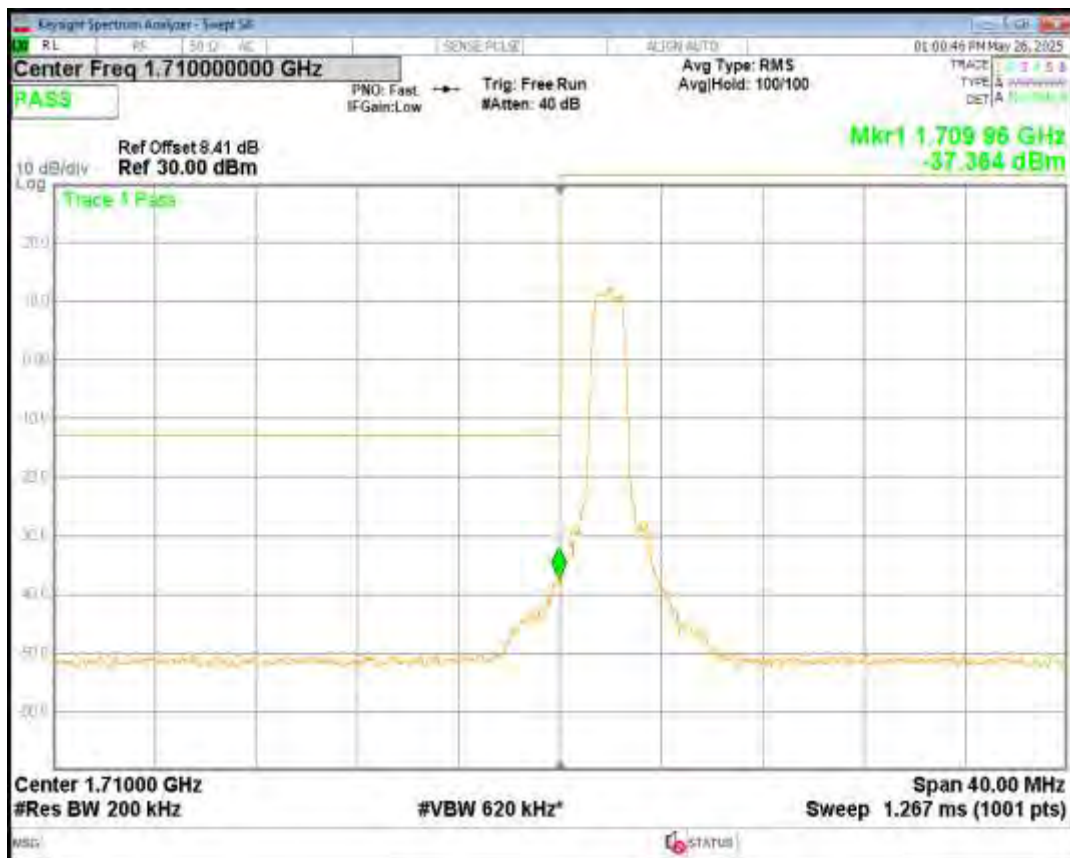
Band4 QPSK BW=20MHz Channel=20300 RB Size=1 Position=#Max NB Index=15
