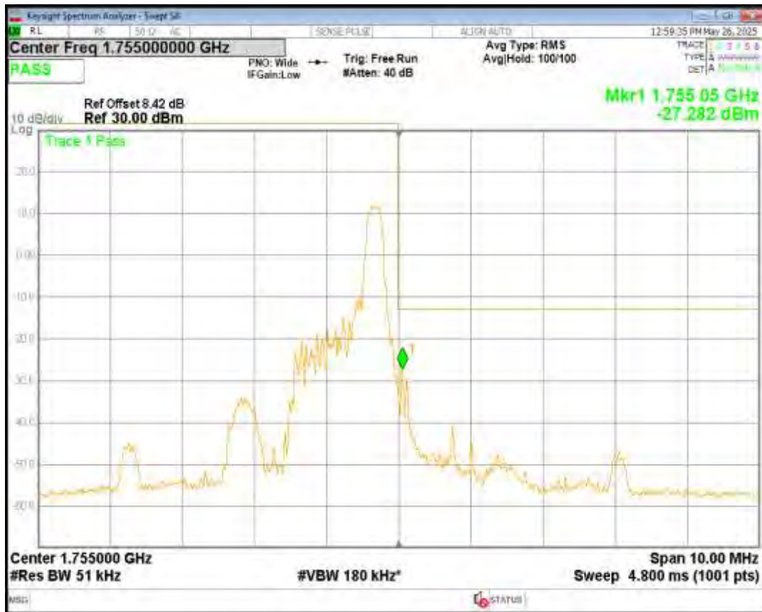
Band4 16QAM BW=5MHz Channel=20375 RB Size=5 Position=#Max NB Index=3
