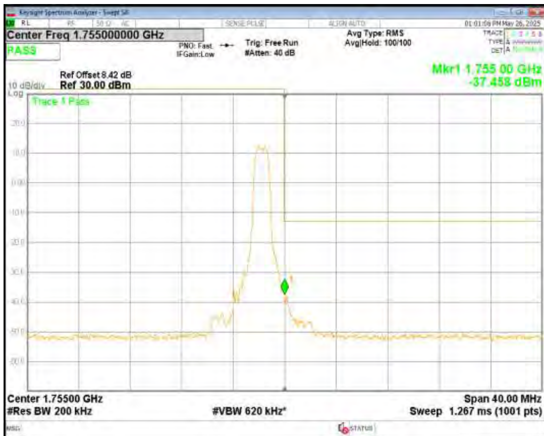
Band4 16QAM BW=3MHz Channel=19965 RB Size=1 Position=#0 NB Index=0
