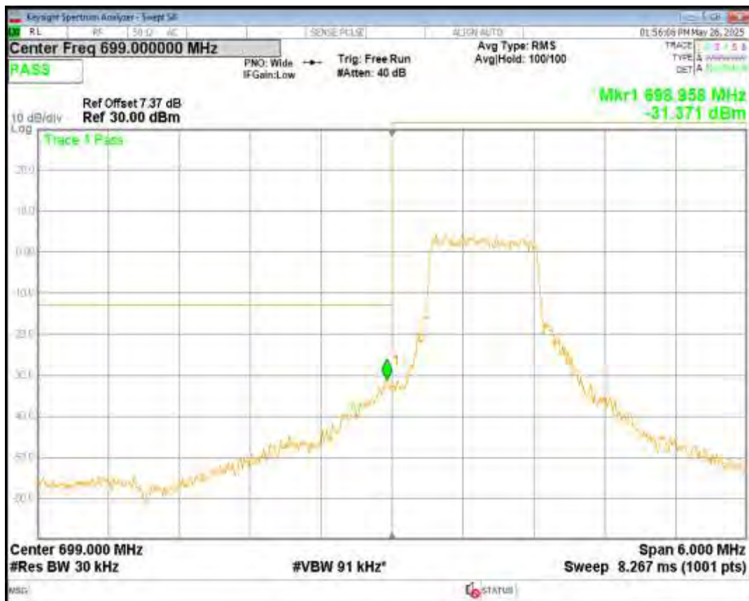
Band12 16QAM BW=3MHz Channel=23165 RB Size=1 Position=#Max NB Index=1
