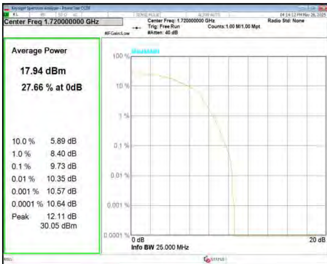
Band4 16QAM BW=20MHz Channel=20175 RB Size=5 Position=#0 NB Index=0
