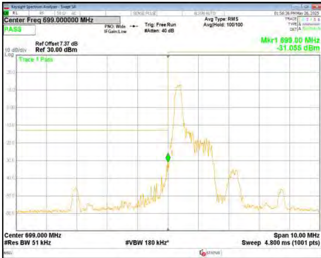
Band12 16QAM BW=5MHz Channel=23035 RB Size=5 Position=#0 NB Index=0
