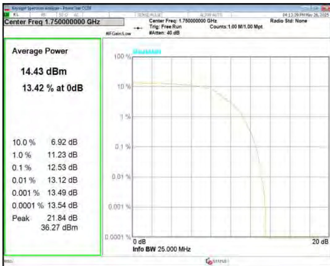
Band4 QPSK BW=15MHz Channel=20025 RB Size=6 Position=#0 NB Index=0
