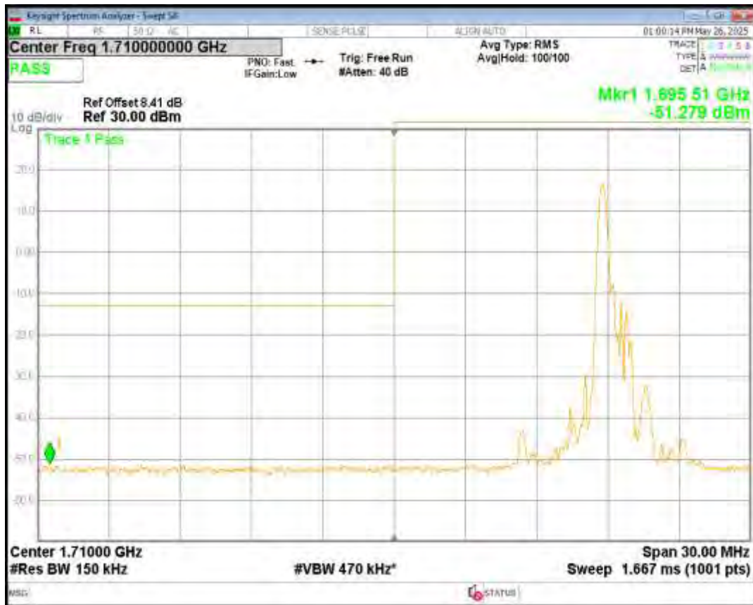
Band4 QPSK BW=15MHz Channel=20025 RB Size=6 Position=#0 NB Index=7
