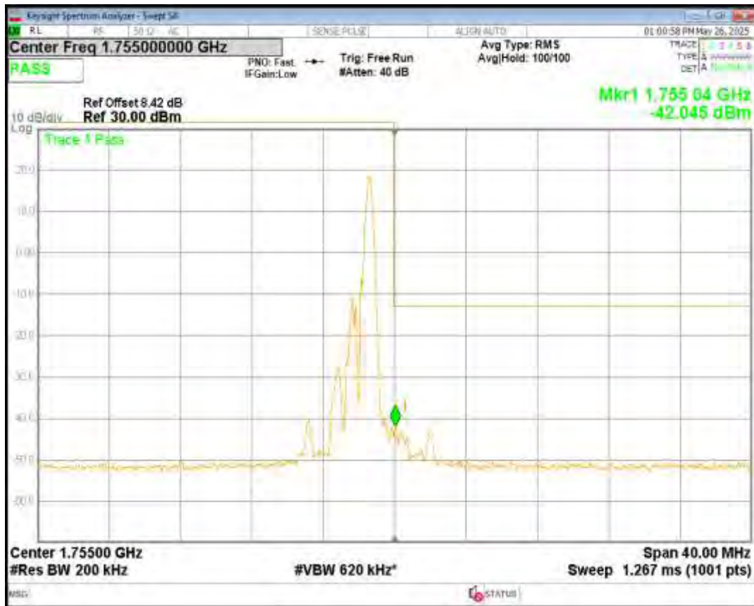
Band4 QPSK BW=20MHz Channel=20300 RB Size=6 Position=#Max NB Index=15
