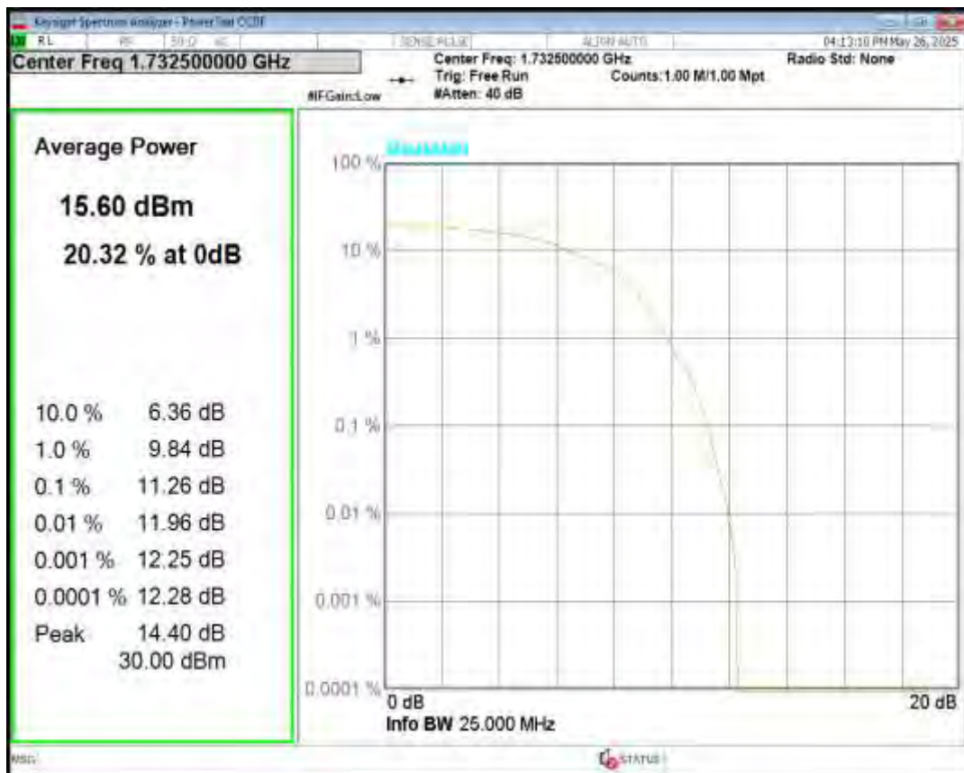
Band4 16QAM BW=5MHz Channel=20375 RB Size=5 Position=#0 NB Index=0
