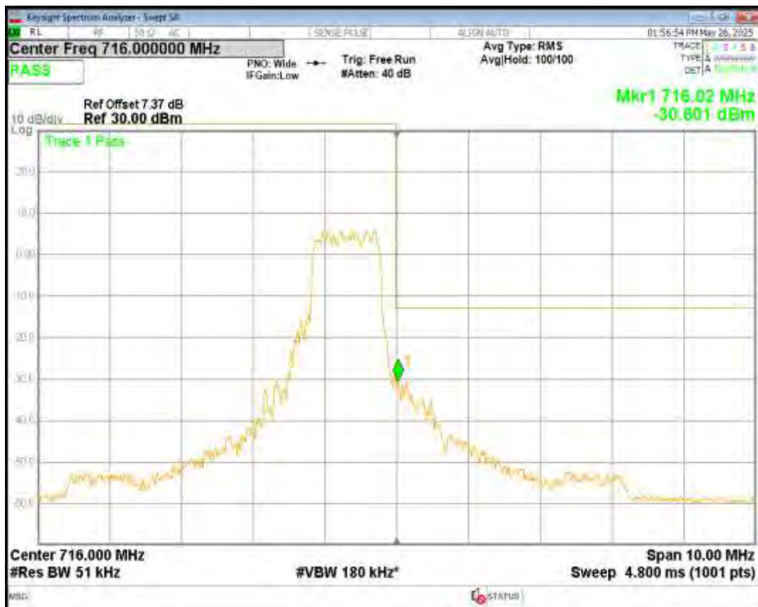
Band12 QPSK BW=1.4MHz Channel=23017 RB Size=1 Position=#0 NB Index=0
