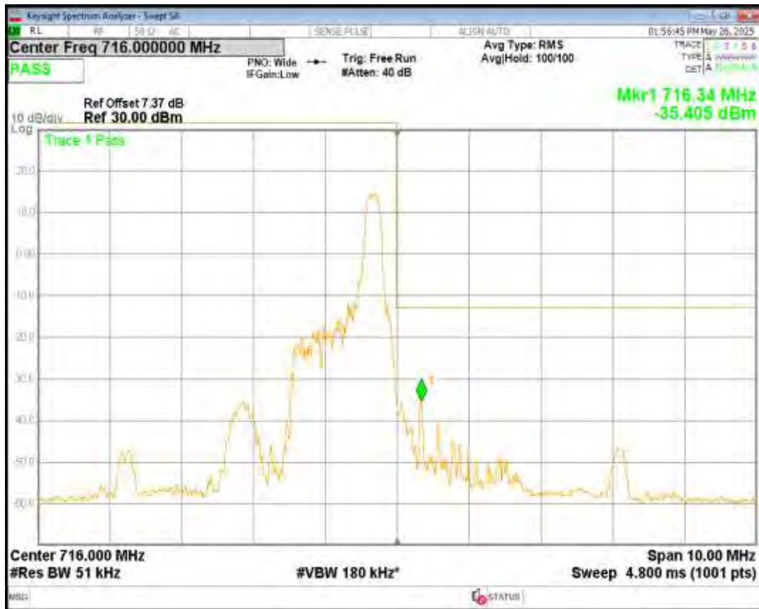
Band12 QPSK BW=5MHz Channel=23155 RB Size=6 Position=#Max NB Index=3
