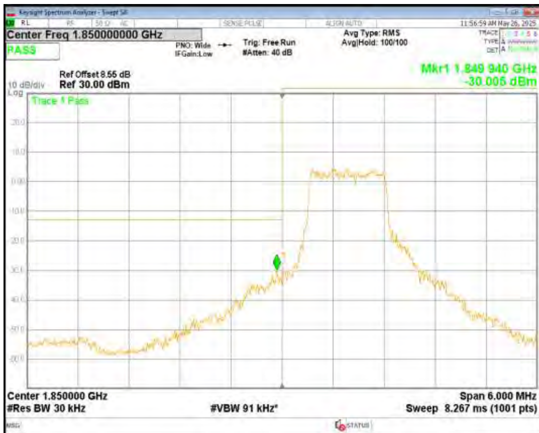
Band2 16QAM BW=3MHz Channel=19185 RB Size=1 Position=#Max NB Index=1
