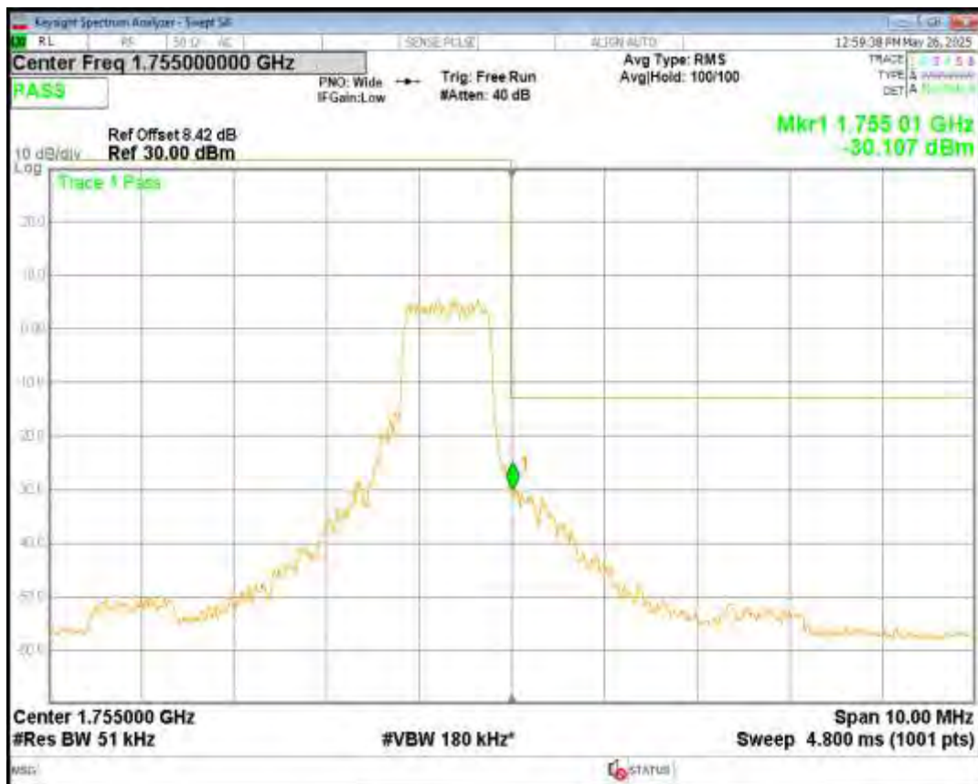
Band4 QPSK BW=1.4MHz Channel=19957 RB Size=1 Position=#0 NB Index=0
