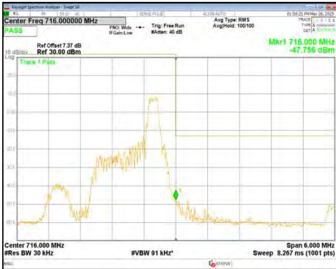
Band12 16QAM BW=3MHz Channel=23165 RB Size=5 Position=#Max NB Index=1
