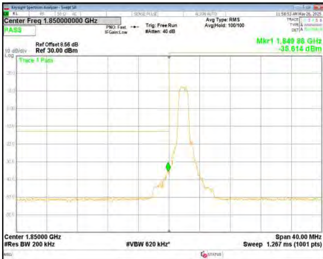
Band2 QPSK BW=20MHz Channel=19100 RB Size=1 Position=#Max NB Index=15
