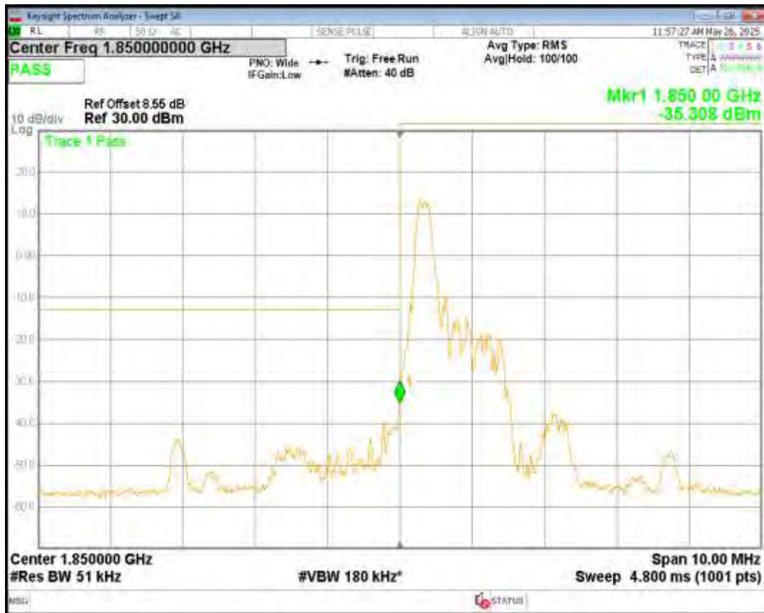
Band2 16QAM BW=5MHz Channel=18625 RB Size=5 Position=#0 NB Index=0
