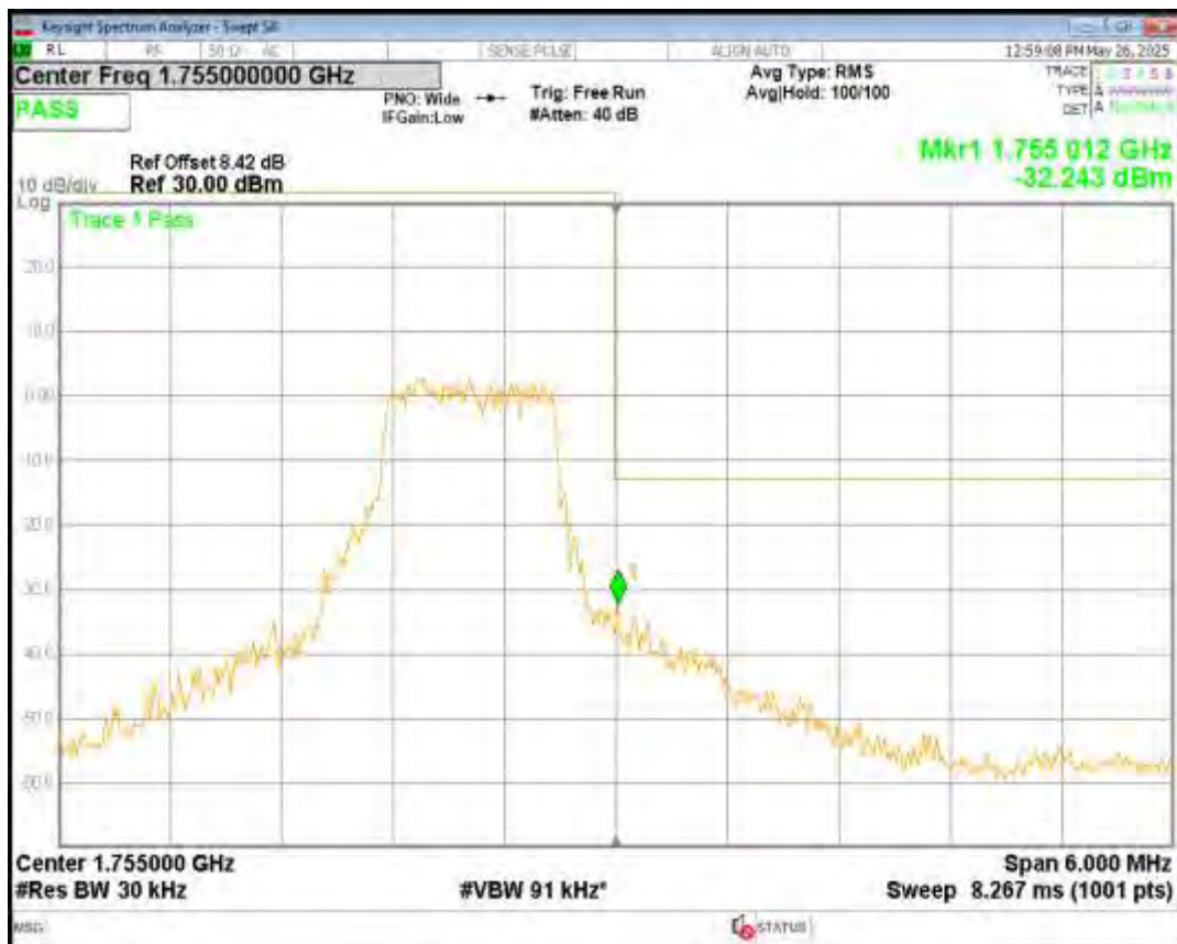
Band4 16QAM BW=5MHz Channel=19975 RB Size=1 Position=#0 NB Index=0
