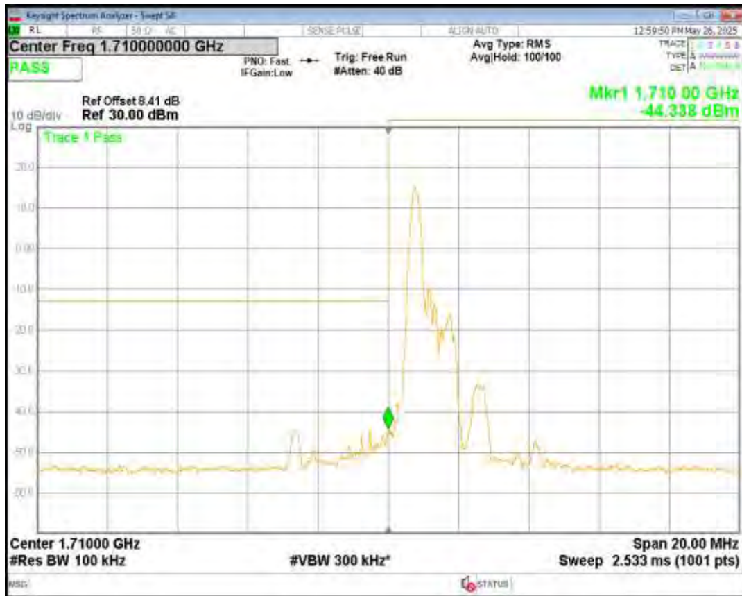
Band4 16QAM BW=10MHz Channel=20000 RB Size=4 Position=#0 NB Index=0
