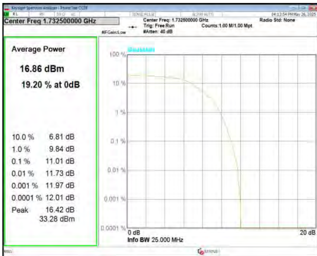
Band4 QPSK BW=15MHz Channel=20325 RB Size=6 Position=#0 NB Index=0
