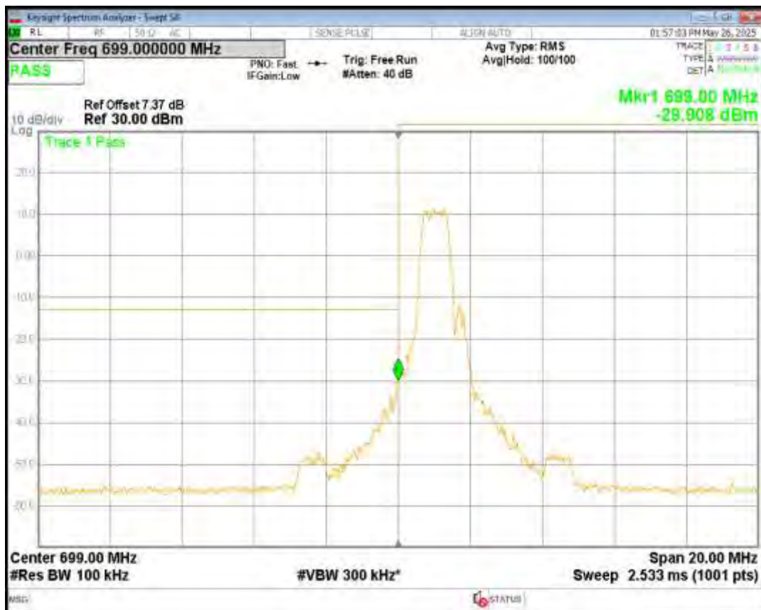
Band12 QPSK BW=10MHz Channel=23130 RB Size=1 Position=#Max NB Index=7
