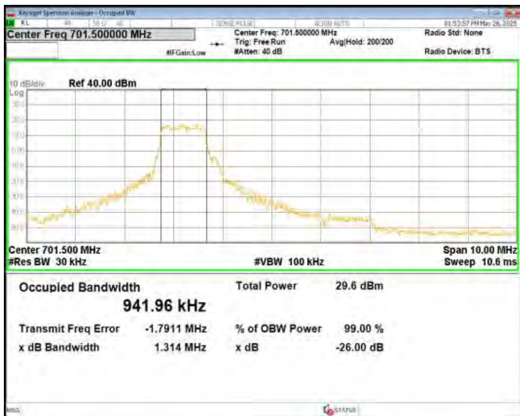
Band12 16QAM BW=5MHz Channel=23095 RB Size=5 Position=#0 NB Index=0
