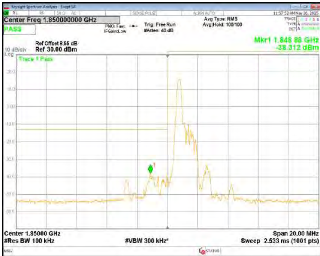
Band2 QPSK BW=10MHz Channel=18650 RB Size=4 Position=#0 NB Index=0
