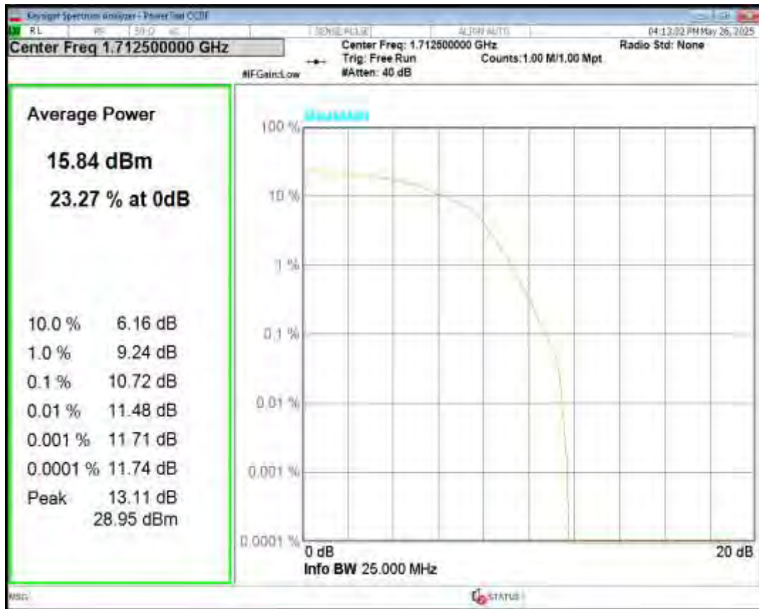
Band4 16QAM BW=5MHz Channel=20175 RB Size=5 Position=#0 NB Index=0
