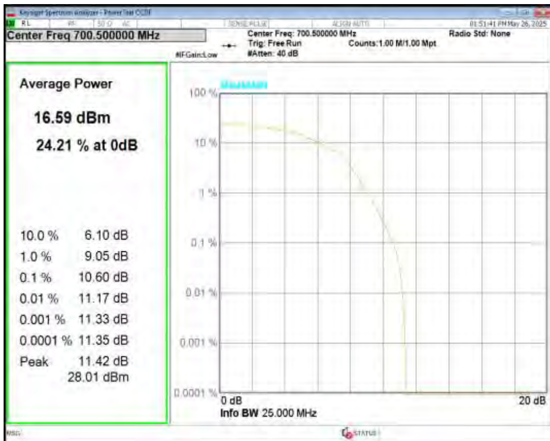
Band12 16QAM BW=3MHz Channel=23095 RB Size=5 Position=#0 NB Index=0
