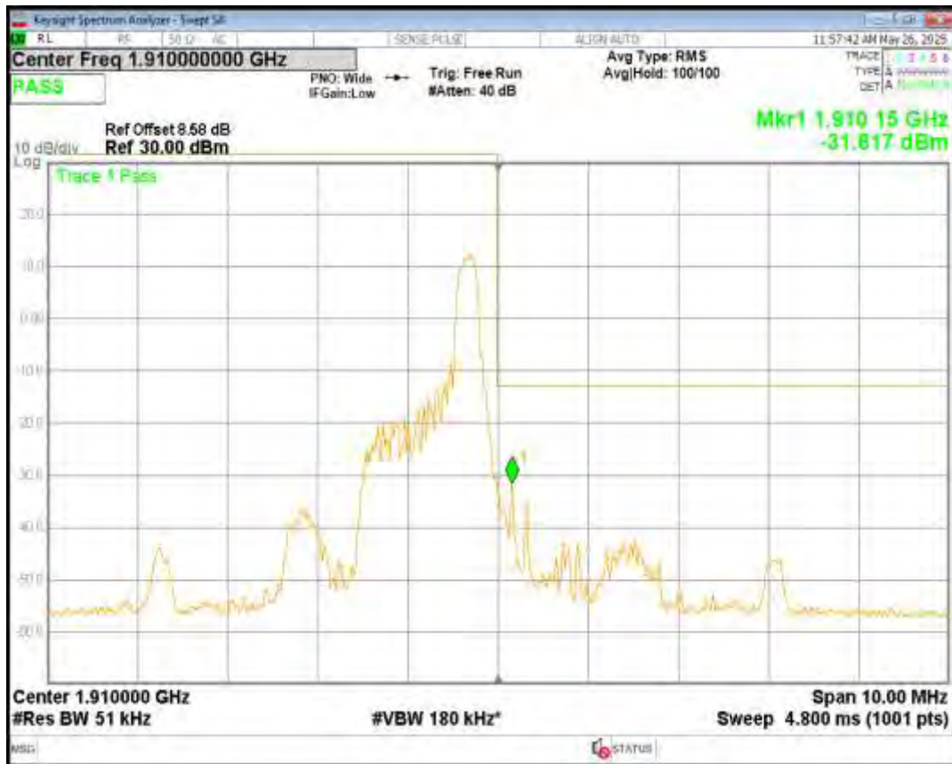
Band2 16QAM BW=5MHz Channel=19175 RB Size=5 Position=#Max NB Index=3
