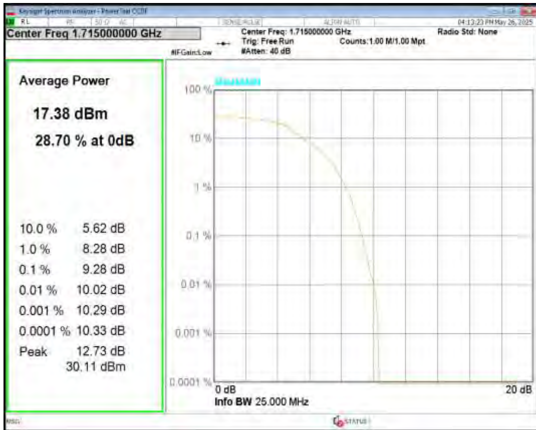
Band4 QPSK BW=10MHz Channel=20175 RB Size=6 Position=#0 NB Index=0
