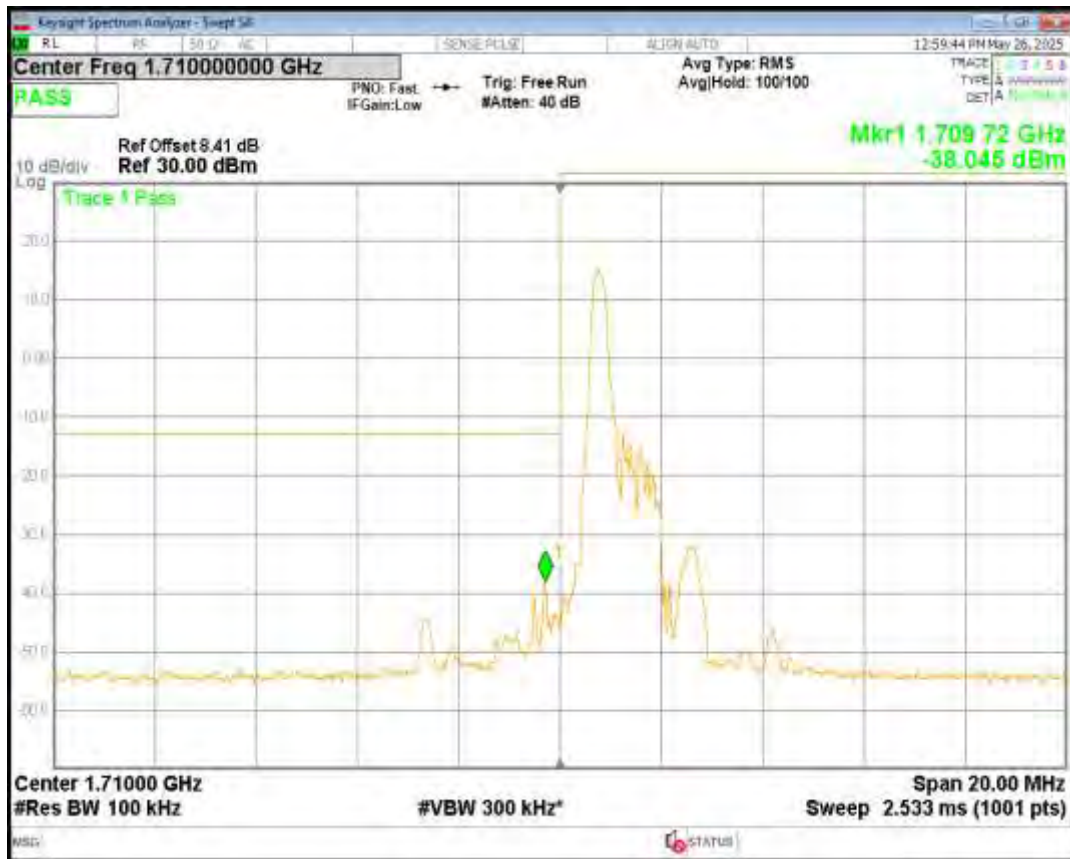
Band4 QPSK BW=10MHz Channel=20000 RB Size=4 Position=#0 NB Index=0
