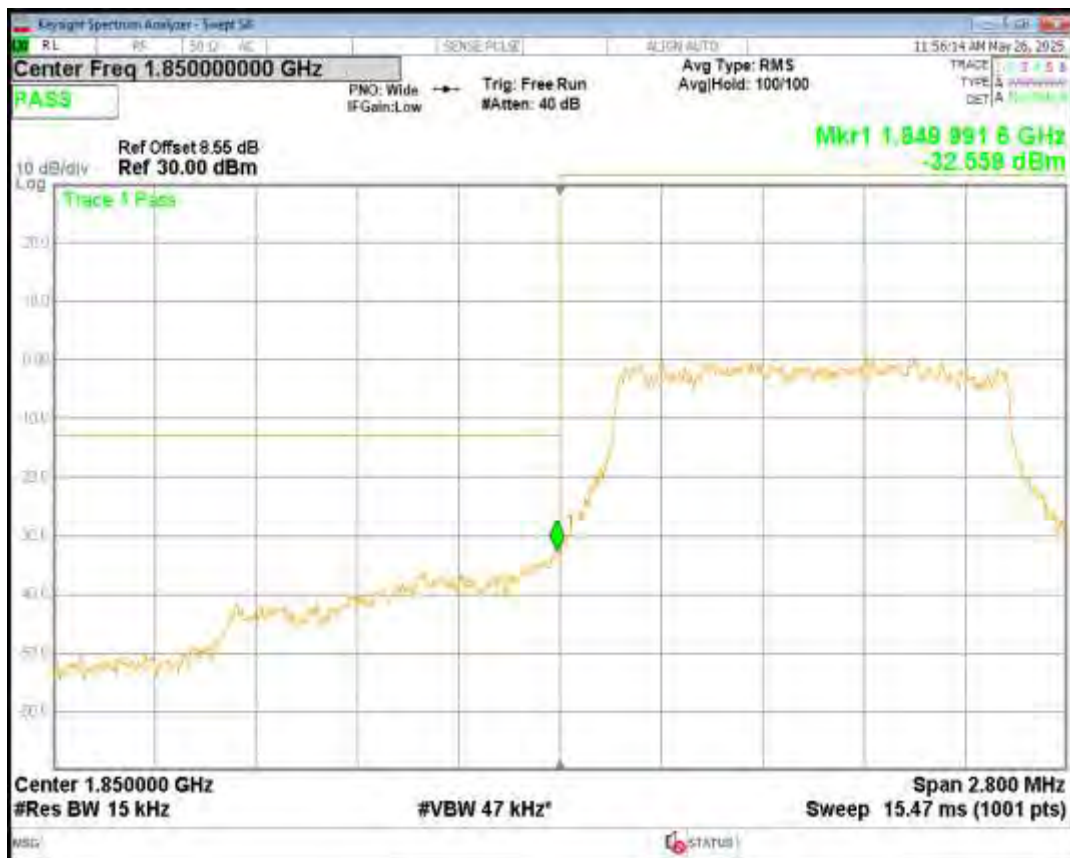
Band2 QPSK BW=1.4MHz Channel=19193 RB Size=1 Position=#Max NB Index=0
