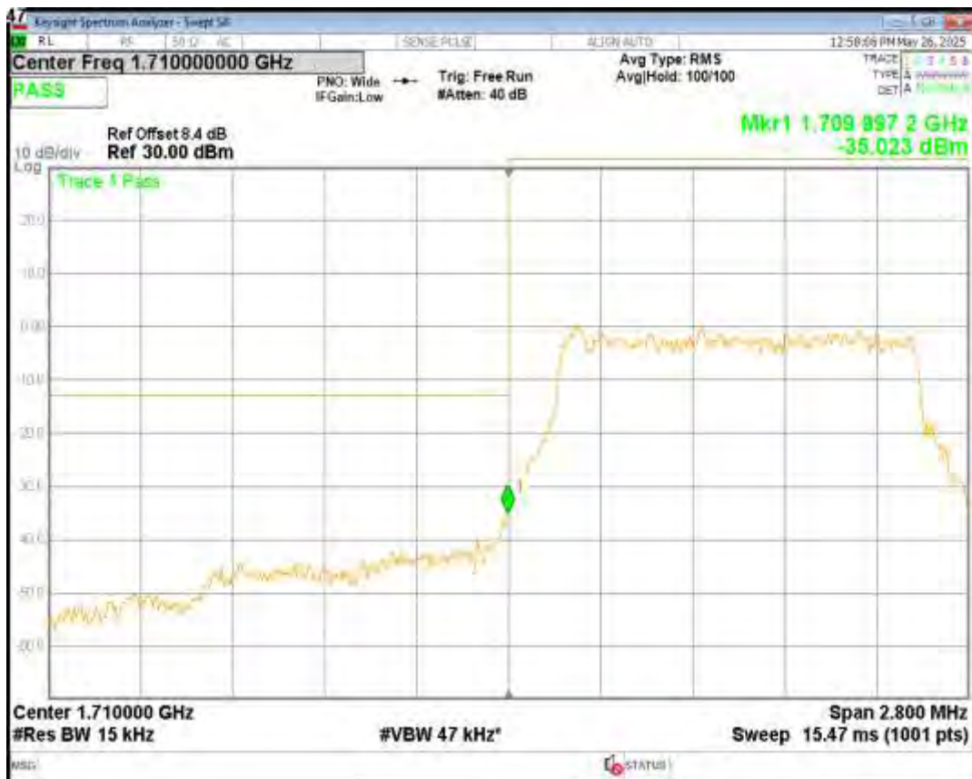
Band4 QPSK BW=1.4MHz Channel=20393 RB Size=1 Position=#Max NB Index=0
