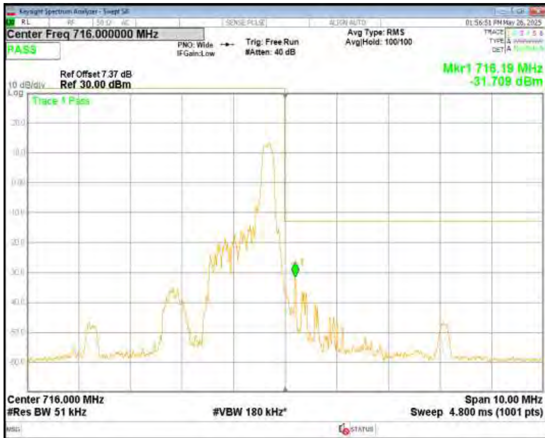
Band12 16QAM BW=5MHz Channel=23155 RB Size=5 Position=#Max NB Index=3
