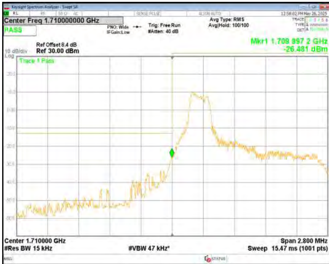
Band4 QPSK BW=1.4MHz Channel=19957 RB Size=6 Position=#0 NB Index=0
