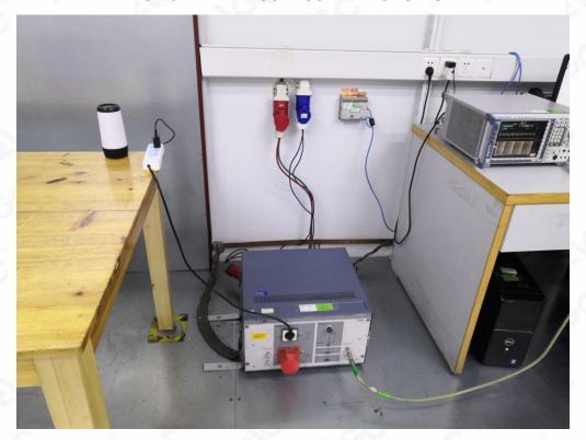
RF CONDUCTED TEST SETUP
