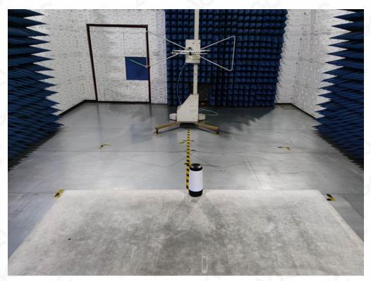
RADIATED EMISSION TEST SETUP ABOVE 1GHz
