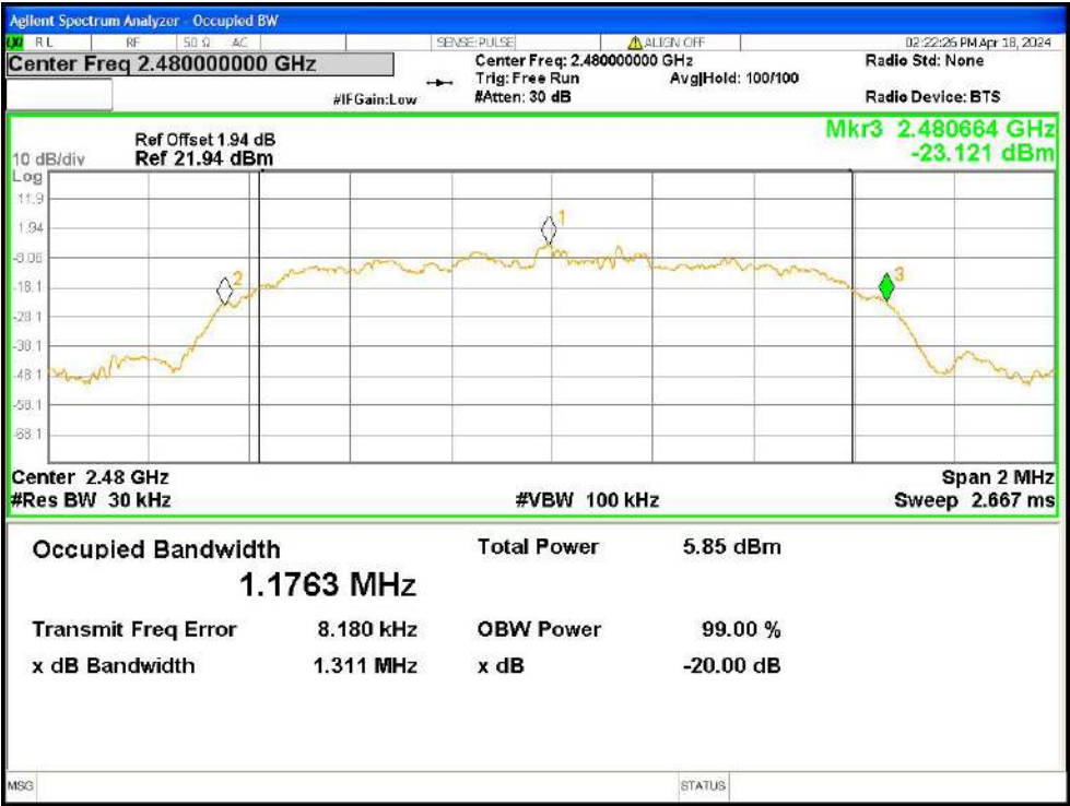
-20dB Bandwidth NVNT 2-DH5 2480MHz Ant1
