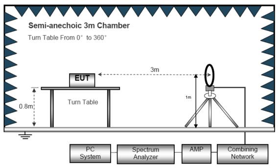
(B) Radiated Emission Test-Up Frequency 30MHz~1GHz
