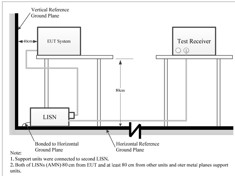
The setup of EUT is according with per ANSI C63.10-2020 measurement procedure. The specification used was with the FCC Part 15.207, RSS-Gen limits.
