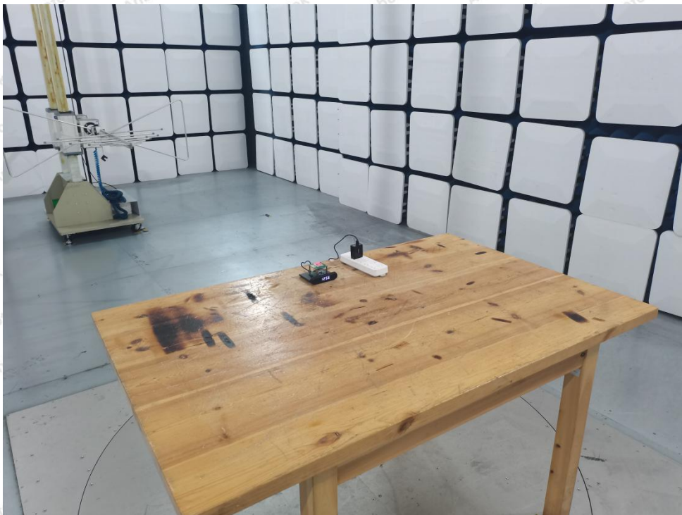
Photo of Radiation Emission Test
