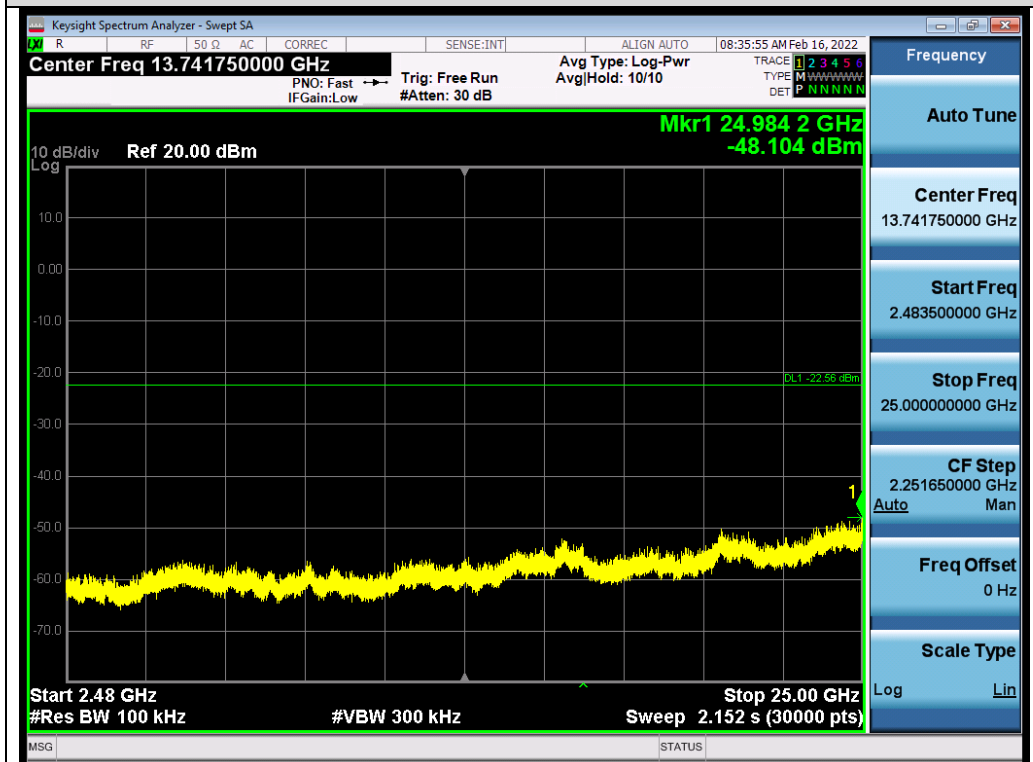
Test_Graph_802.11g_ANT1_2412_6Mbps_Higher Band Emissions
