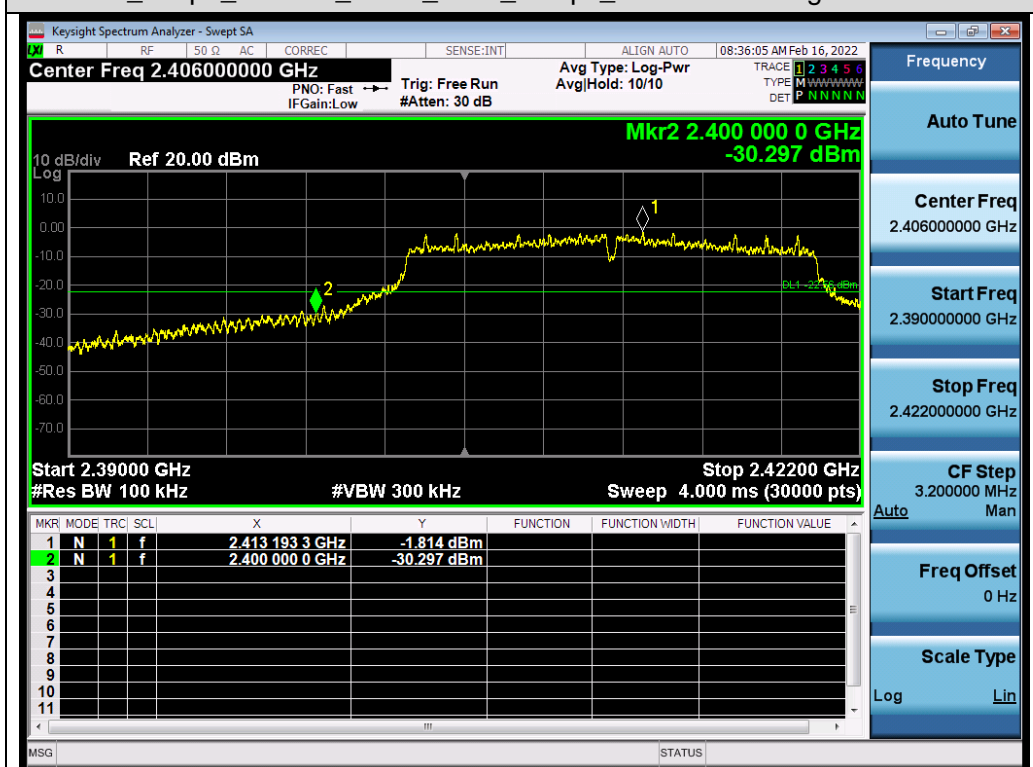
Test_Graph_802.11g_ANT1_2412_6Mbps_Lower Band Edge Emissions
