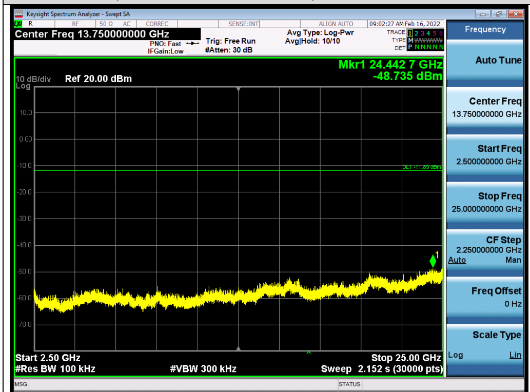
Test_Graph_802.11b_ANT1_2462_1Mbps_Higher Band Emissions
