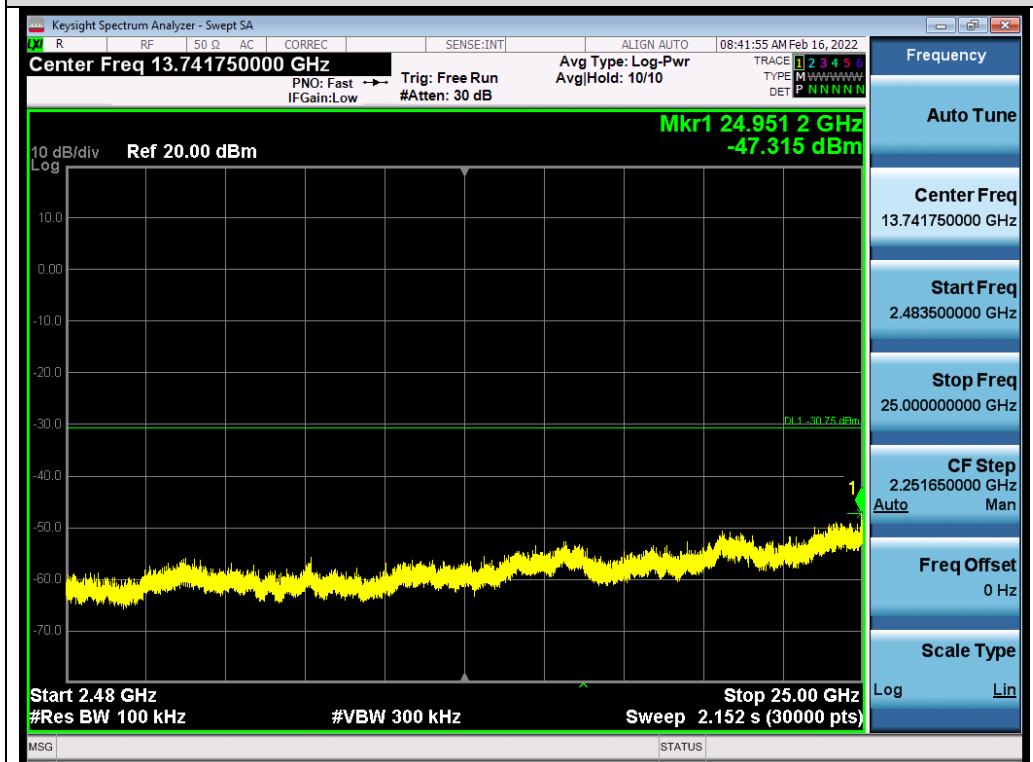
Test_Graph_802.11g_ANT1_2437_6Mbps_Higher Band Emissions
