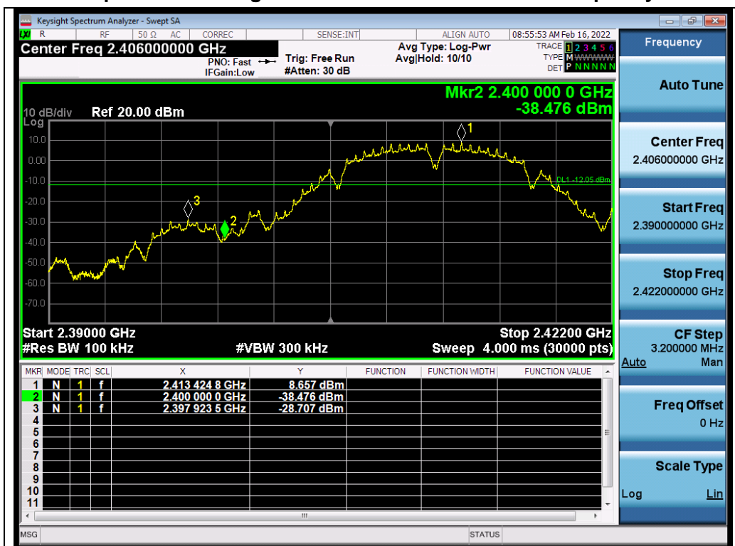
Test_Graph_802.11b_ANT1_2412_1Mbps_Lower Band Edge Emissions
