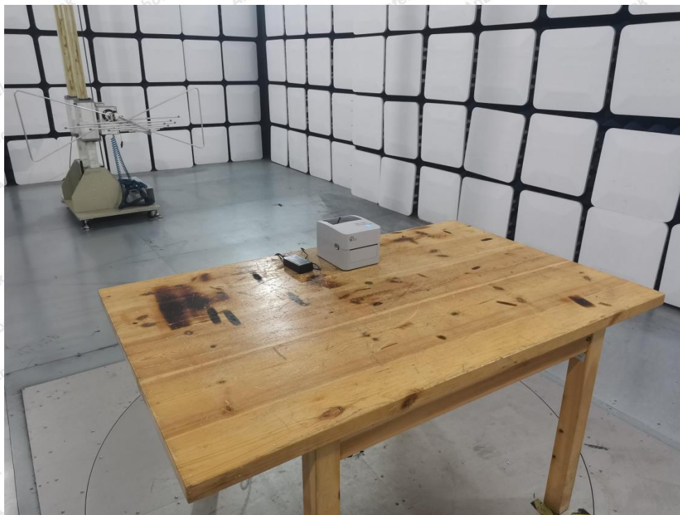
Photo of Radiation Emission Test
