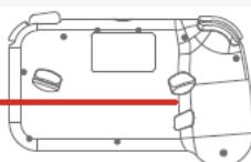
If any abnormal situations occur with the gaming touchpad, you can press the [RESET] button on the back of the gaming touchpad to restore it to its initial state.
