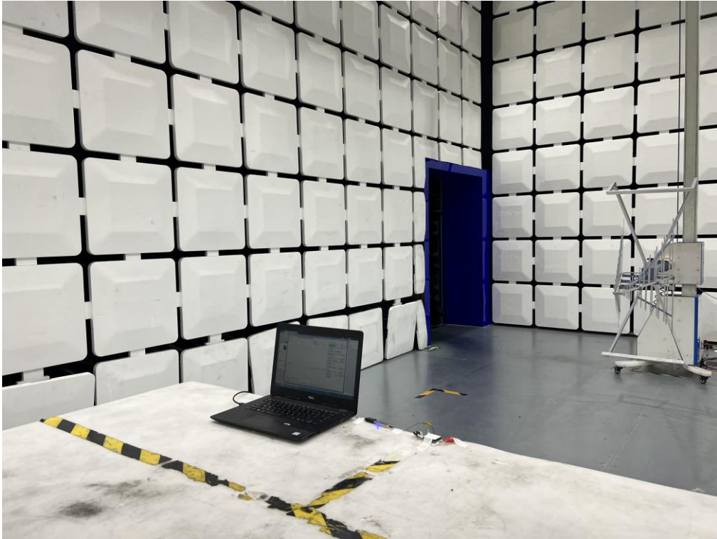
Description: Radiated Emission Test Setup for 30MHz ~ 1GHz
