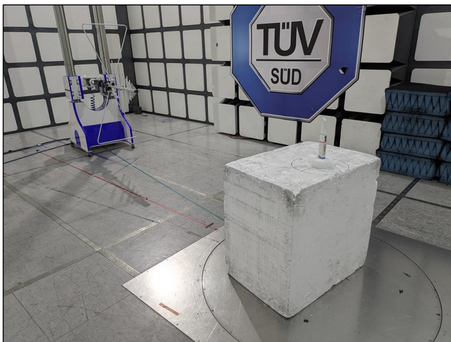
Figure 164 - Test setup - 30 MHz to 1 GHz
