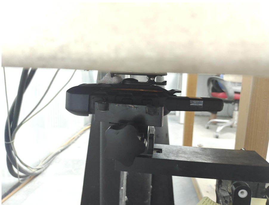
Body Back With Headset Setup Photo (0mm)
