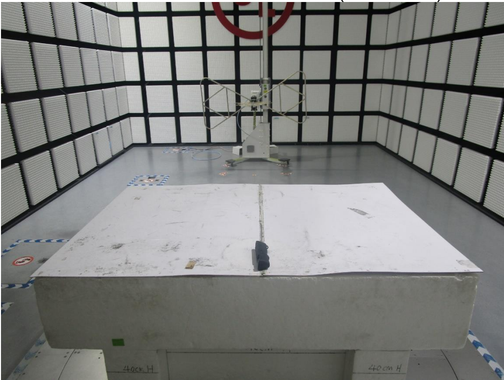
RADIATED RF MEASUREMENT SETUP (30MHz~1GHz)
