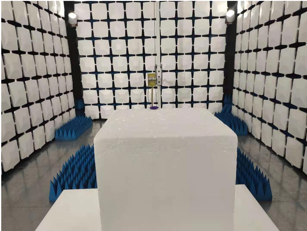
Below 1GHz for radiated emission test setup
