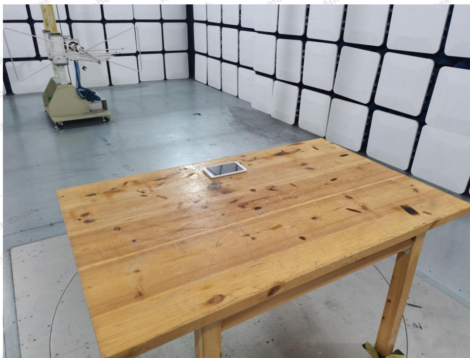
Photo of Radiation Emission Test
