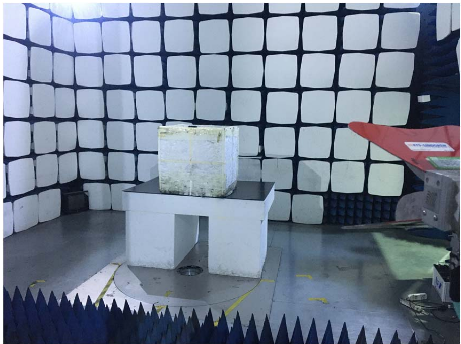
Radiation Emission Test Setup (1GHz to 18GHz)
