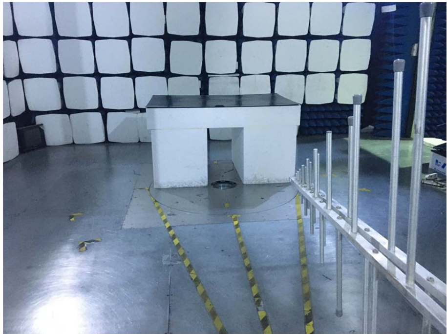
Radiation Emission Test Setup (30MHz to 1GHz)
