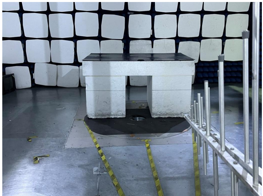
Radiation Emission Test Setup (30MHz to 1GHz)
