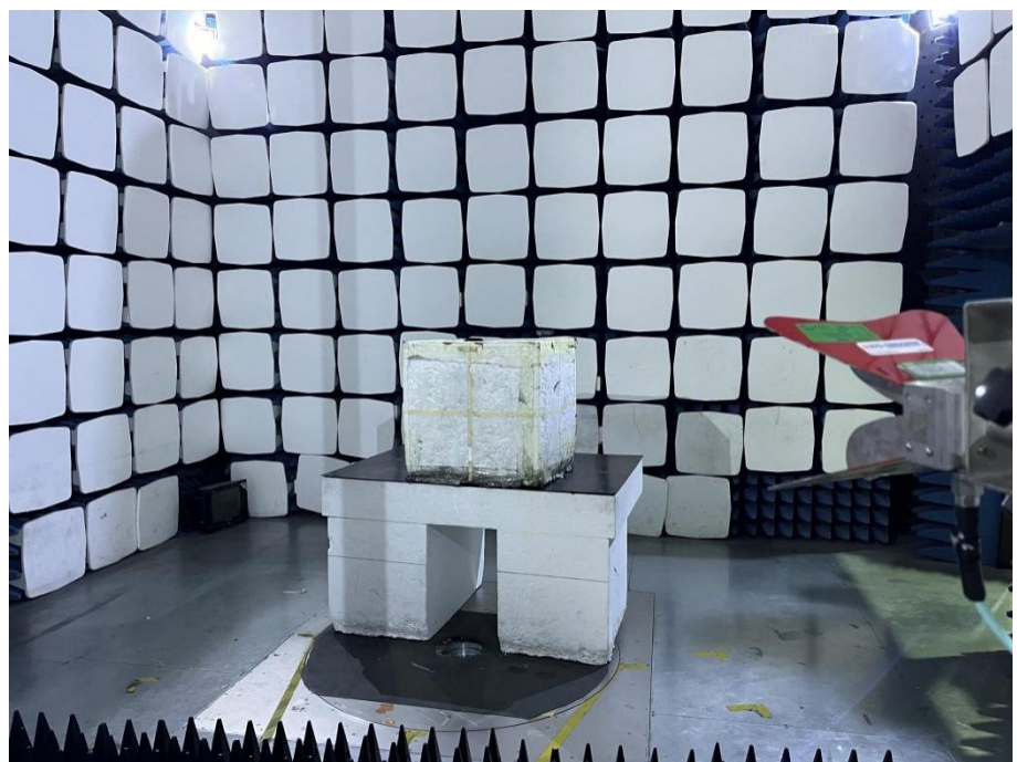
Radiation Emission Test Setup (1GHz to 18GHz)
