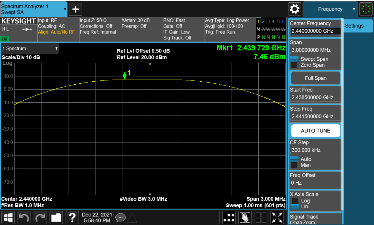
Figure 2: Peak Output Power, 2440MHz
