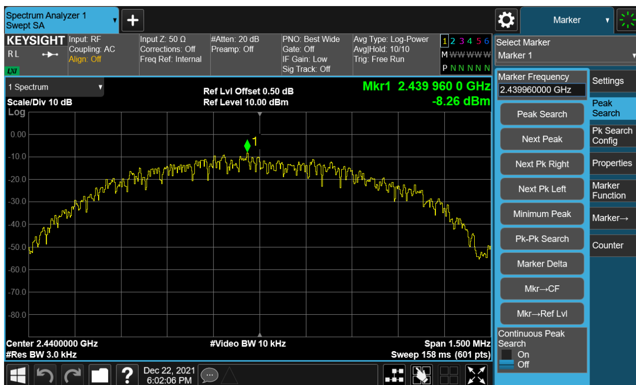
Figure 8: Power Spectral Density, 2440MHz
