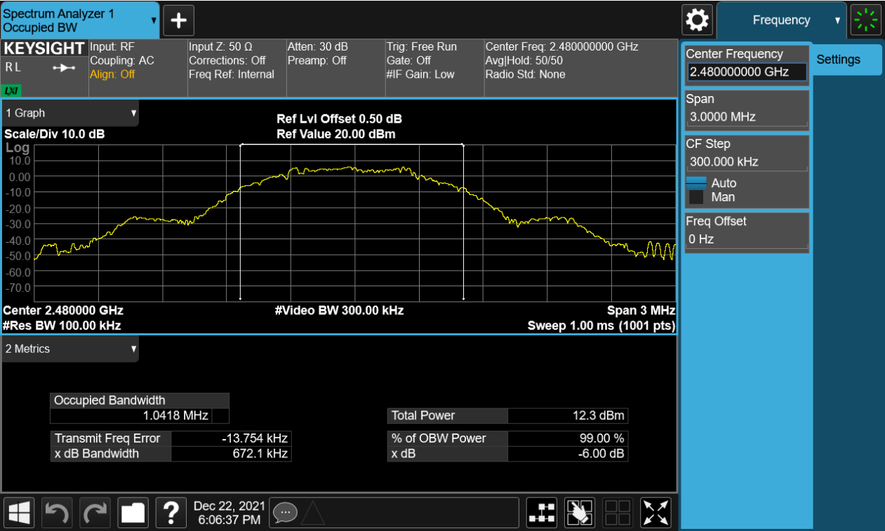
Figure 6: 6dB Bandwidth, 2480MHz
