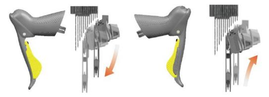
Press the right hand to get bigger button and the small button at the same time, and move the rear dial in the direction of the small tooth. Press the hand change button once, the indicator flashes blue, and then returns to solid on.
