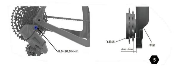
A 5mm Allen wrench is used to attach the transmission to the frame hook, and the appropriate chain is used to alternately pass through the two guide wheels of the transmission. The transmission performance is best when the distance between the inner plane of the chainstay and the outer side of the flywheel minimum gear is maintained at 4-6mm.
