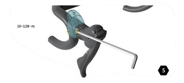
Flip open the rubber sleeve from the top end, loosen the set screws with a 5mm Allen wrench, and then thread the clamp ring through the handlebar. Attach the handset to the handlebar and tighten the fixing bolts.
