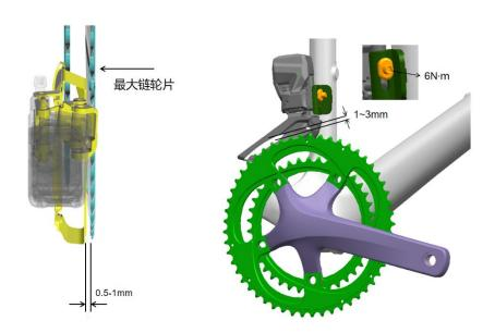
Use a 5mm Allen wrench to attach the front derailleur to the lugs and tighten the
