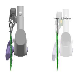
Use the right-hand variable to make fine adjustments until the front derailleur inner guide fits snugly against the chain of the largest chain. If there is no chain as a reference, adjust the distance between the inner guide plate of the front dilleur and the maximum chain wheel to 3.5~5mm.
