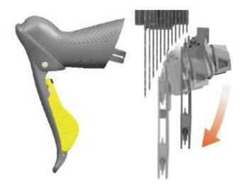
1. Press the button on your right hand to increase the gear, and the transmission shifts to the large gear. Each time the indicator flashes, long press to continuously upshift.
