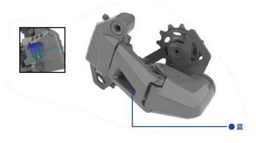
1. Enter pairing: Open the rear dial dust cover, connect the magnetic connector of the charging cable connected to the power supply to the magnetic connector of the rear dial, and the indicator flashes blue to enter pairing mode.
