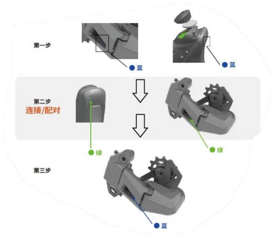
2. Front dial pairing: Open the front dial dust cover, connect the magnetic connector of the charging cable connected to the power supply with the magnetic connector of the front dial, and the indicator flashes blue to enter the pairing mode. After successfully pairing with the rear dial, the rear and front dial indicators will light up green for 1 second, while the blue indicator will continue to flash after the rear dial.
