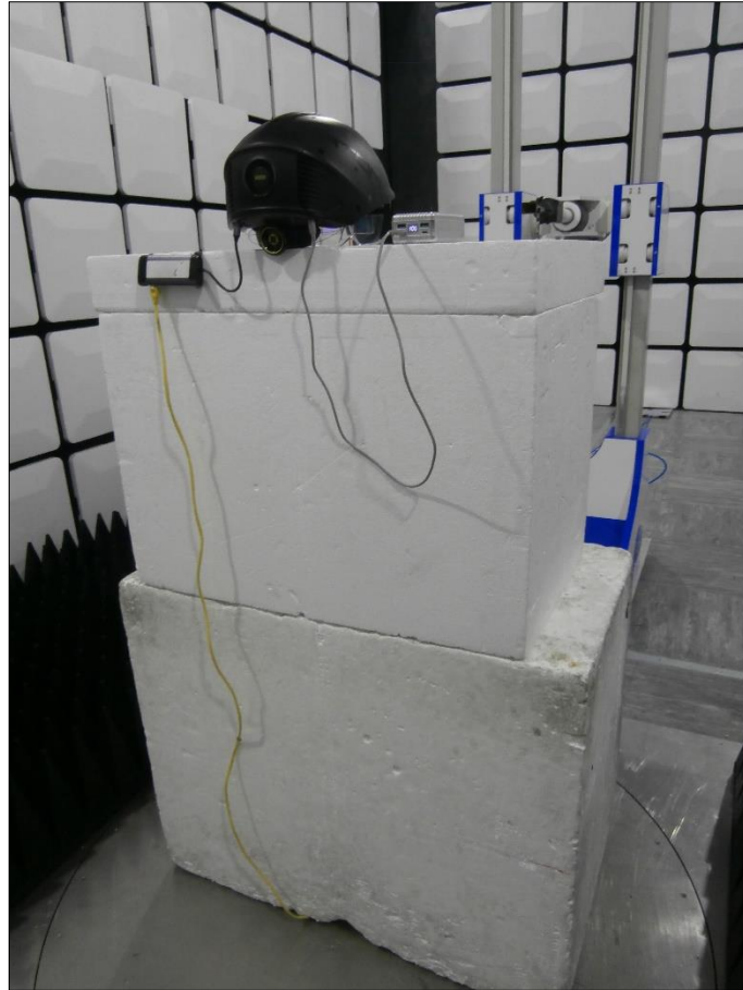
Figure 7 - Test Setup - 18 GHz to 25 GHz - X Orientation
