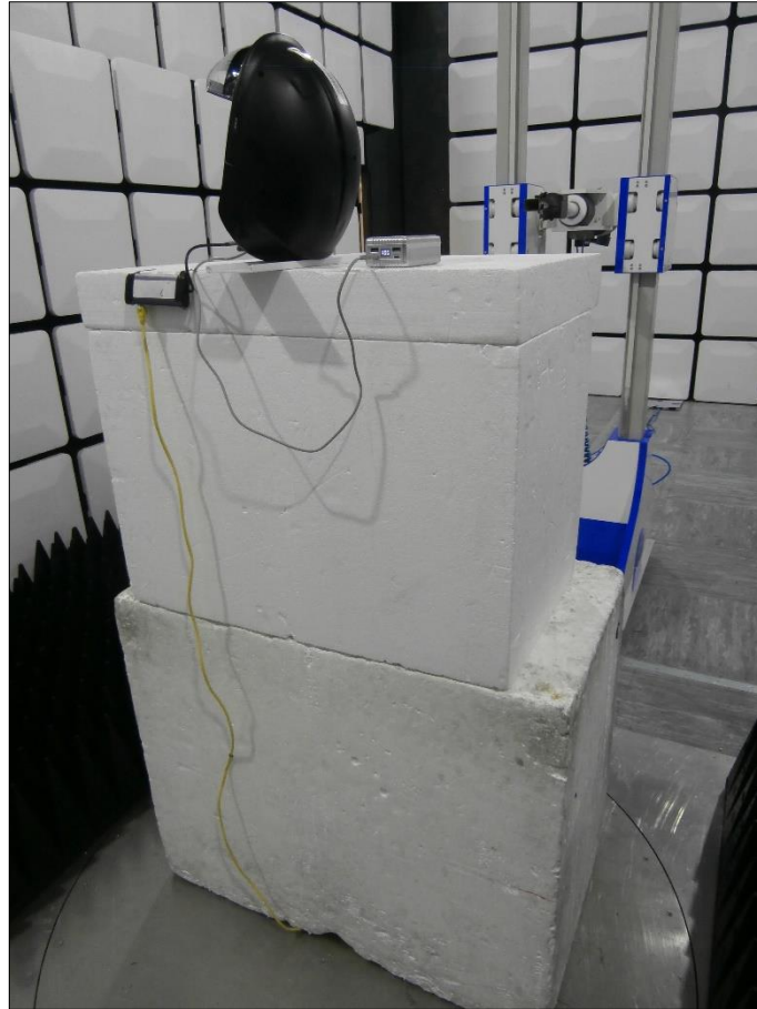
Figure 8 - Test Setup - 18 GHz to 25 GHz - Y Orientation
