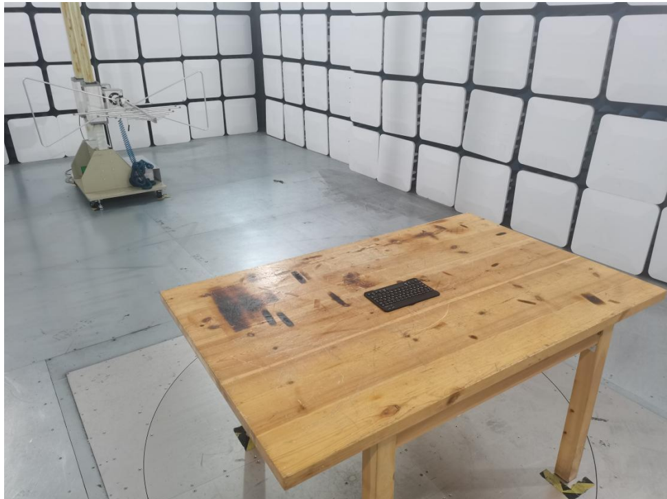
Photo of Radiation Emission Test
