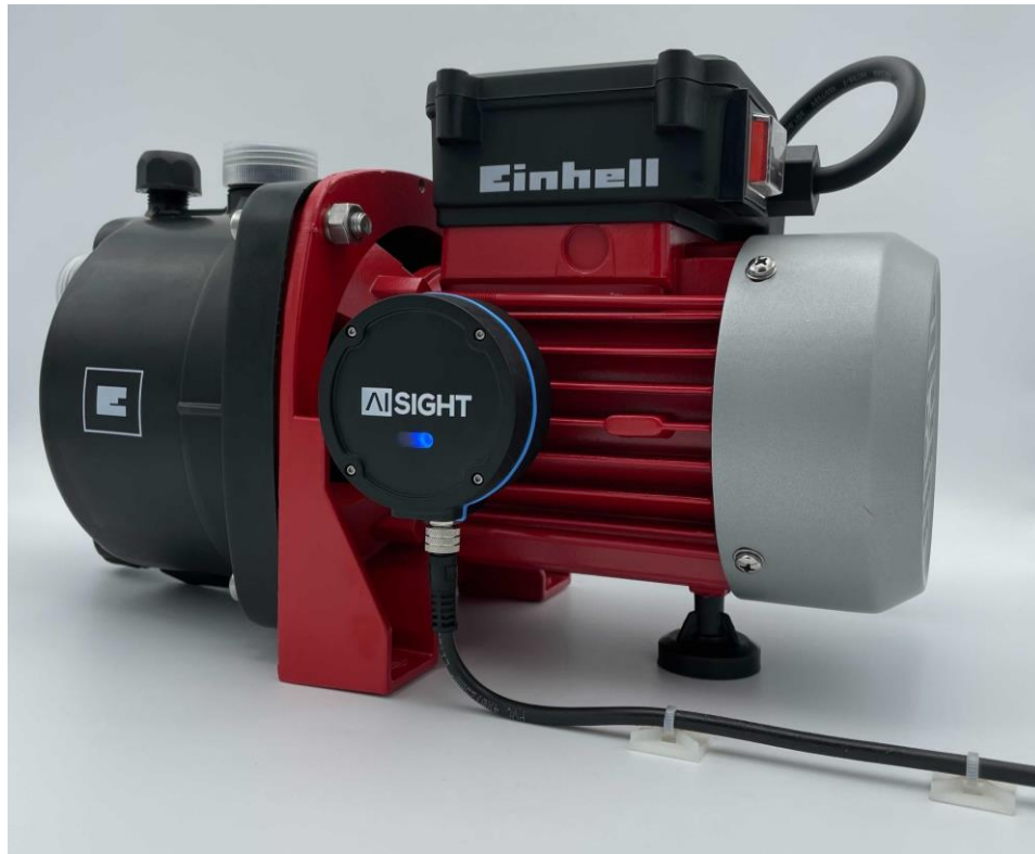
Figure 4.5. Sensor node connected to power and ready to be provisioned
