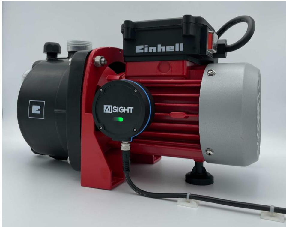
Figure 4.9. Sensor node provisioned and connected to the Wi-Fi
