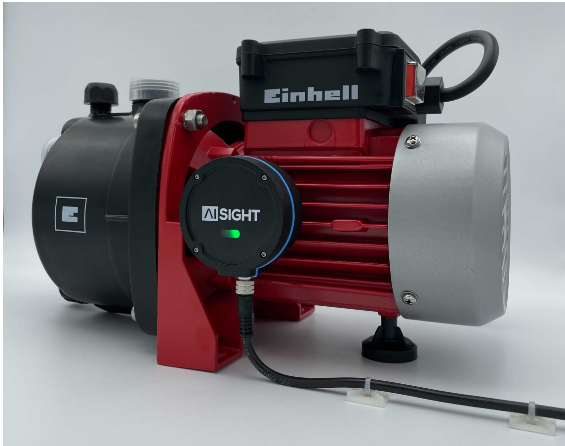
Figure 5.10 - Sensor node provisioned and connected to the Wi-Fi
