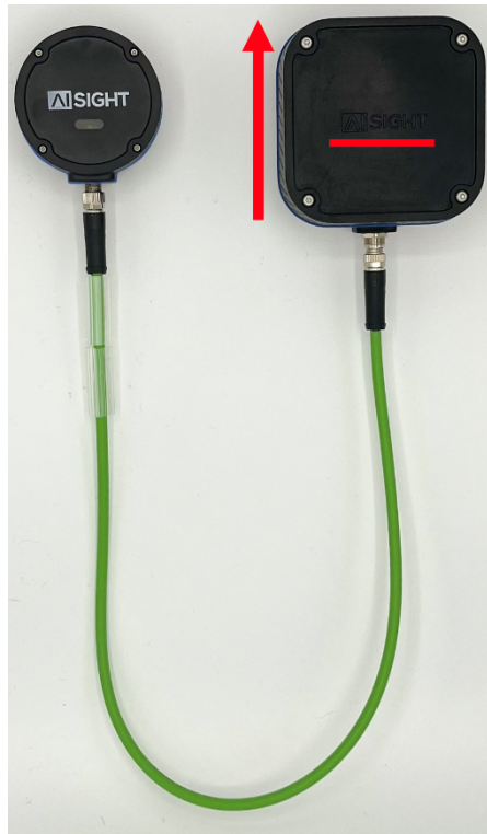
Figure 5.5 - The BP must be aligned so the text reads left to right with the cable extended towards the floor, or as close as possible
