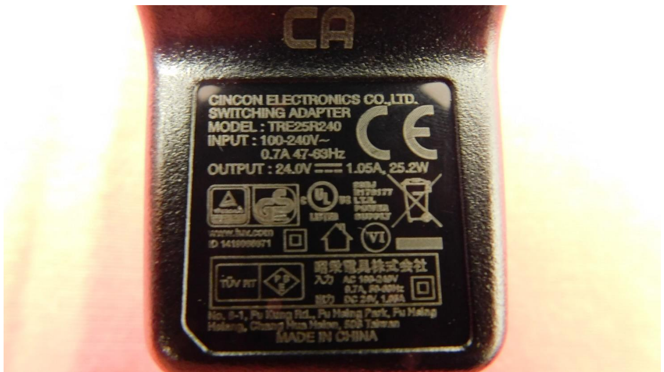
Picture 9: Name plate of power supply
