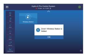
Press and release the button quickly on the TWS-1 to pair the TWS-1 to the main controller. A "pairing successful" message will appear on the HCS-2 display when successful.
