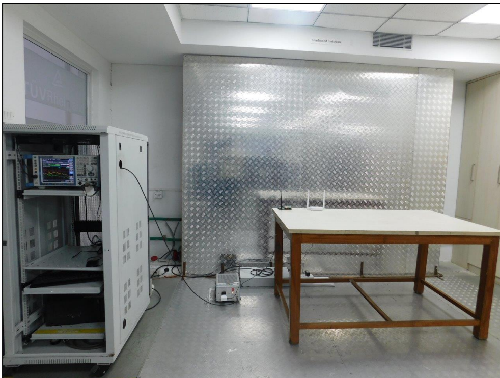
Tset Setup of Conducted Emission on AC Power lines
