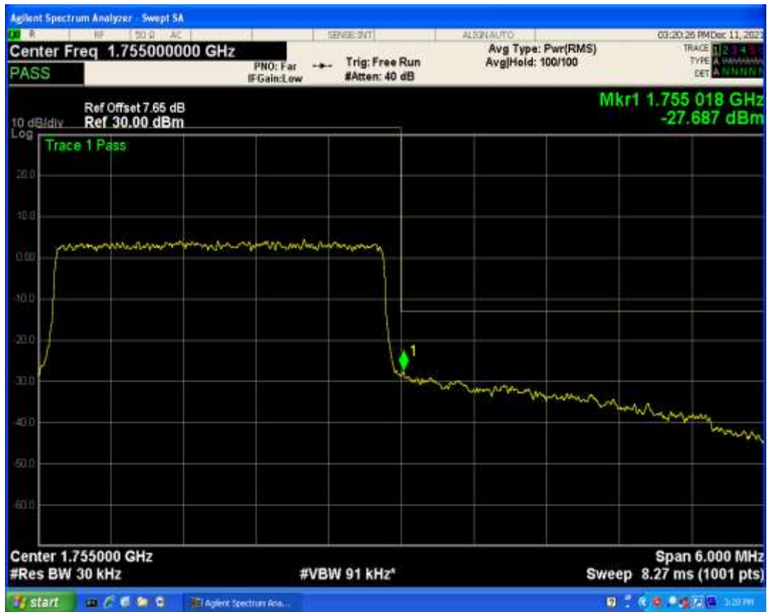
Band4 QPSK BW=5MHz Channel=19975 RB Size=1 Position=#Max
