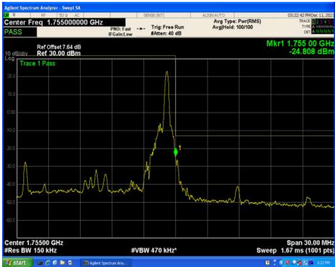
Band4 QPSK BW=15MHz Channel=20325 RB Size=75 Position=#0
