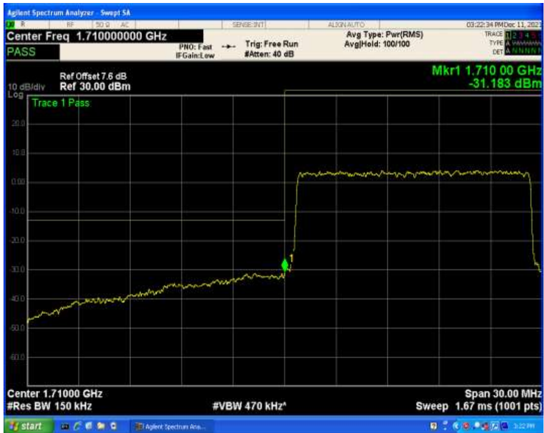
Band4 QPSK BW=15MHz Channel=20325 RB Size=1 Position=#0
