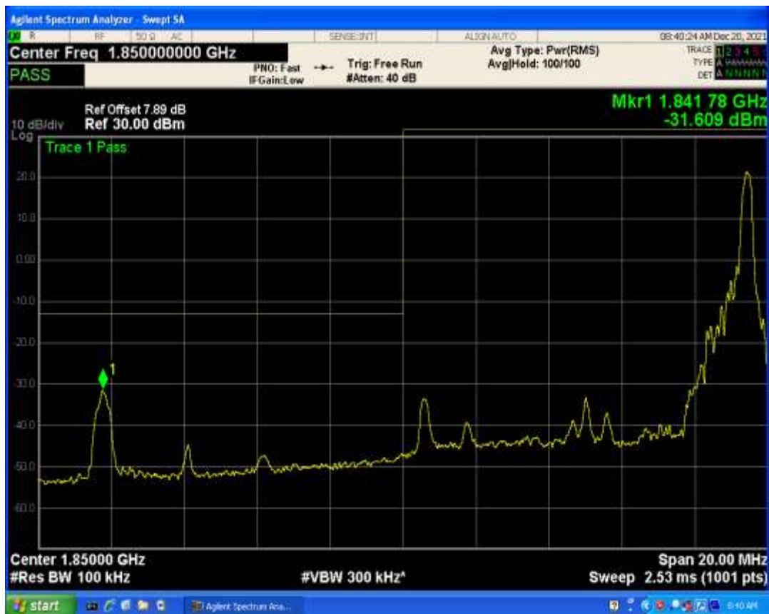
Band2 QPSK BW=10MHz Channel=19150 RB Size=1 Position=#0
