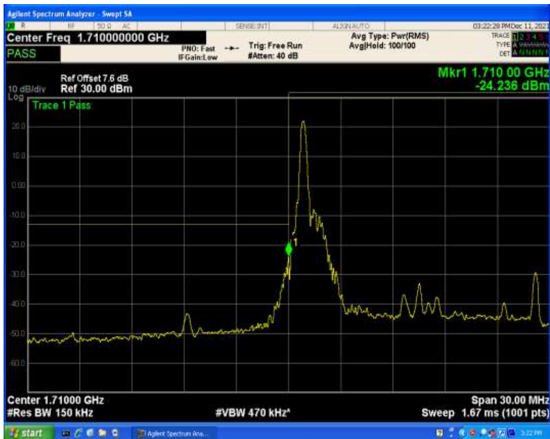
Band4 QAM16 BW=15MHz Channel=20025 RB Size=75 Position=#0
