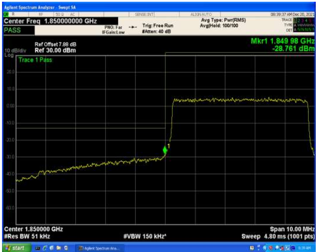
Band2 QPSK BW=5MHz Channel=19175 RB Size=1 Position=#0
