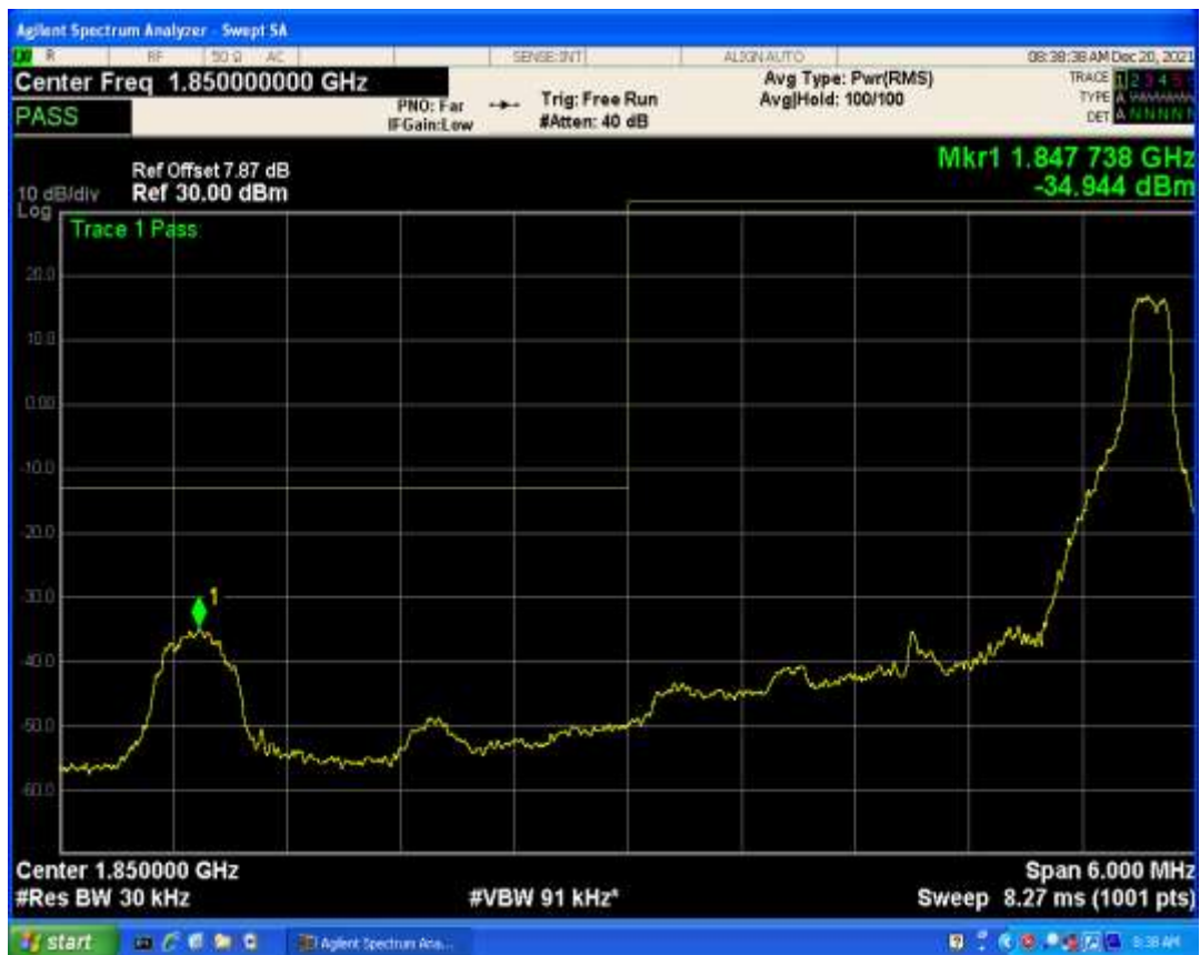
Band2 QPSK BW=3MHz Channel=19185 RB Size=1 Position=#0
