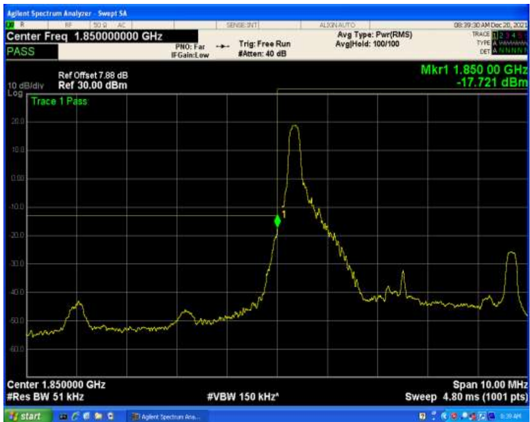
Band2 QPSK BW=5MHz Channel=18625 RB Size=25 Position=#0
