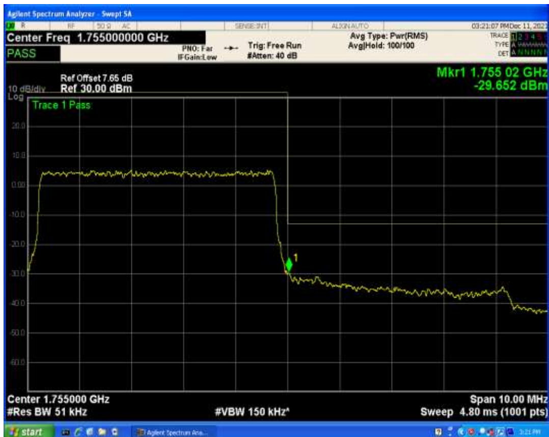
Band4 QAM16 BW=5MHz Channel=20375 RB Size=1 Position=#0
