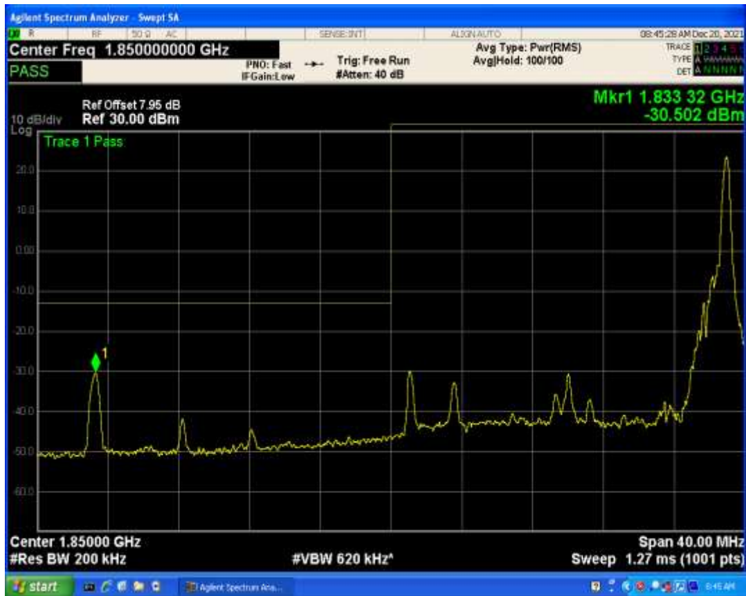
Band2 QAM16 BW=20MHz Channel=18700 RB Size=1 Position=#0
