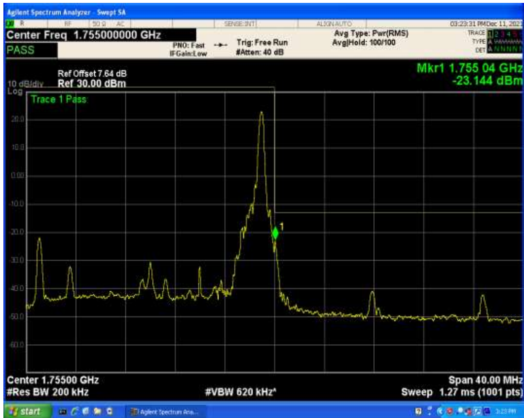
Band4 QPSK BW=20MHz Channel=20300 RB Size=100 Position=#0
