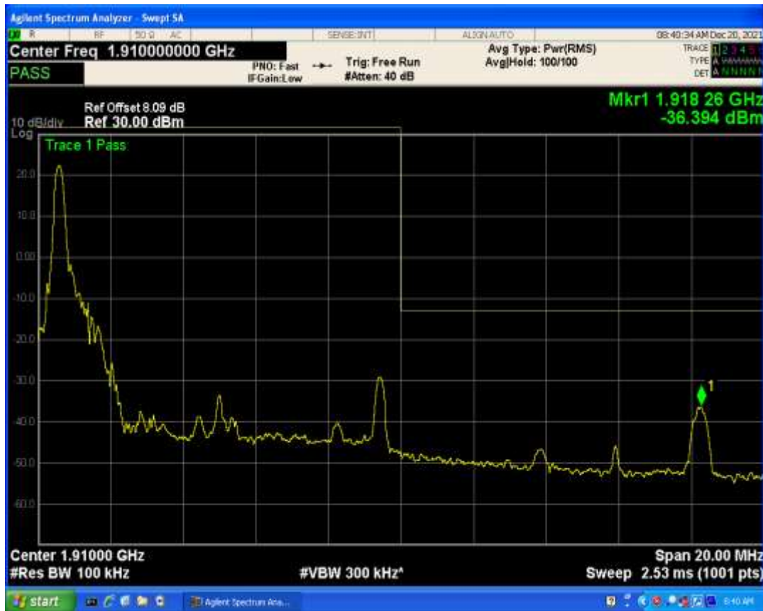
Band2 QAM16 BW=10MHz Channel=18650 RB Size=50 Position=#0
