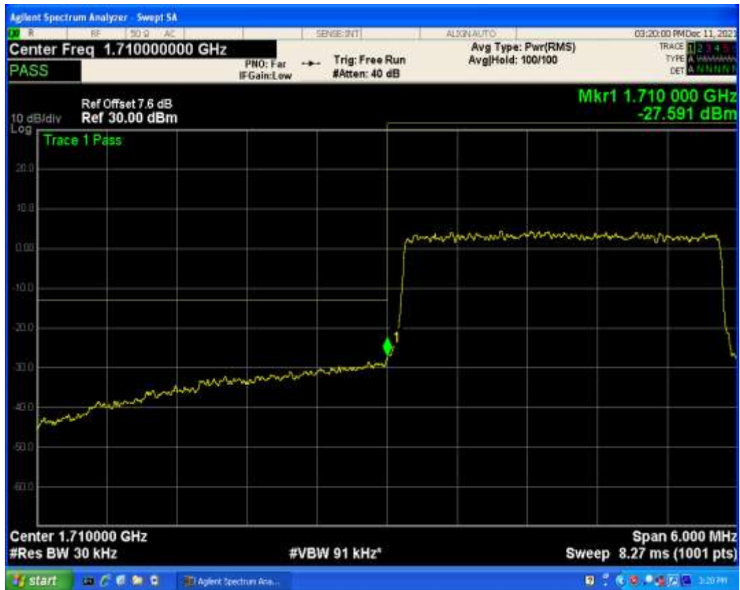
Band4 QPSK BW=3MHz Channel=20385 RB Size=1 Position=#0
