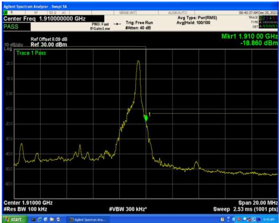
Band2 QPSK BW=10MHz Channel=19150 RB Size=50 Position=#0
