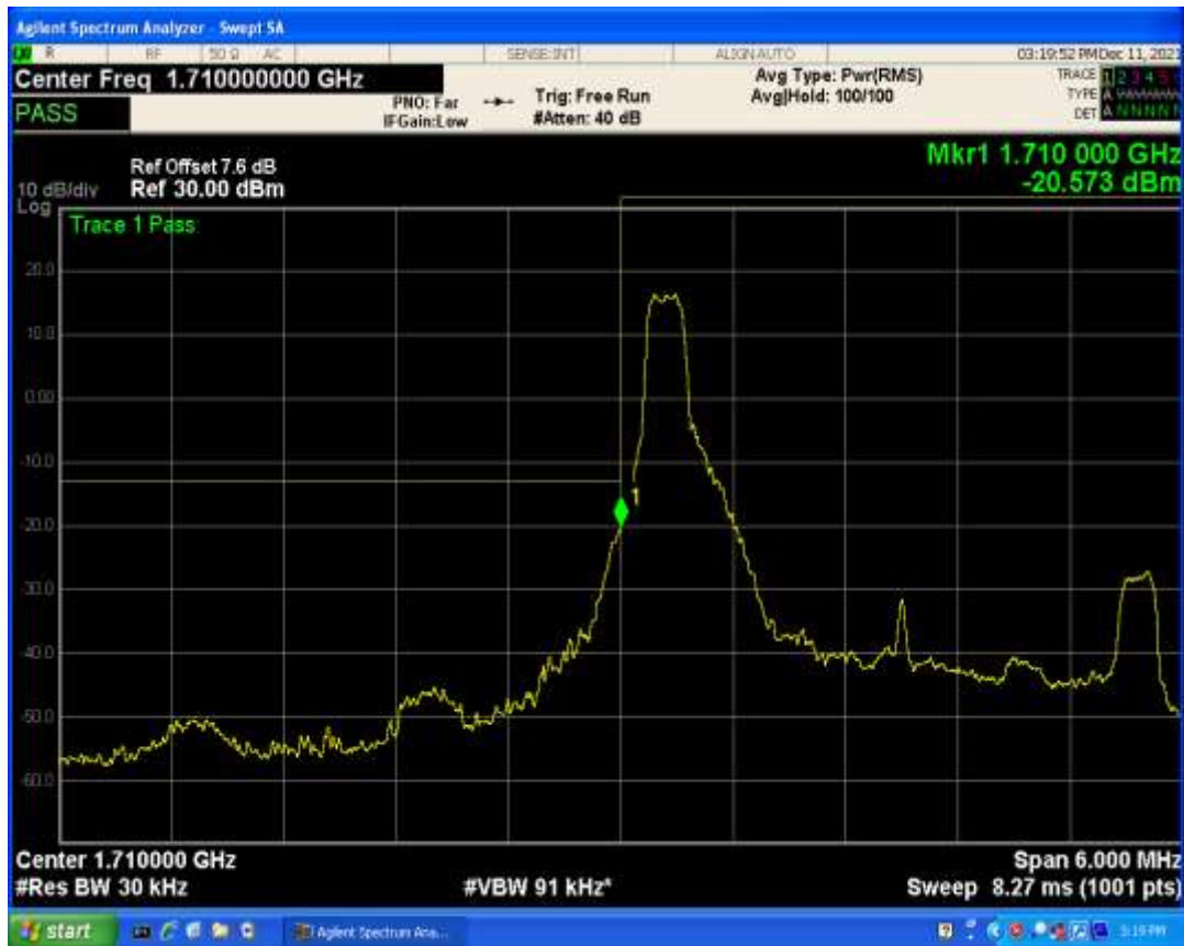
Band4 QAM16 BW=3MHz Channel=19965 RB Size=1 Position=#Max
