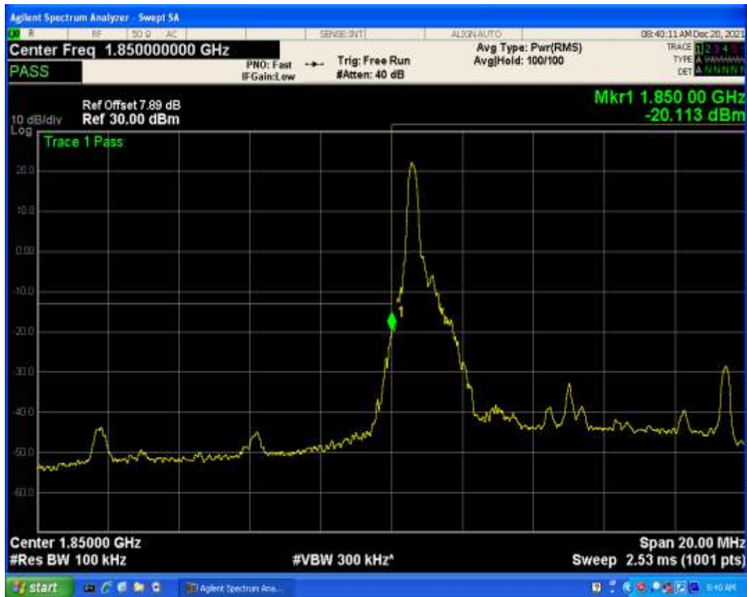
Band2 QAM16 BW=5MHz Channel=19175 RB Size=25 Position=#0
