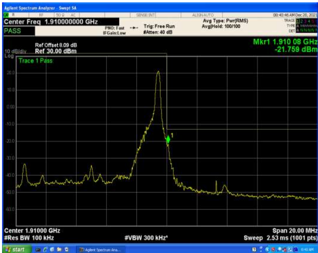
Band2 QPSK BW=15MHz Channel=18675 RB Size=1 Position=#0
