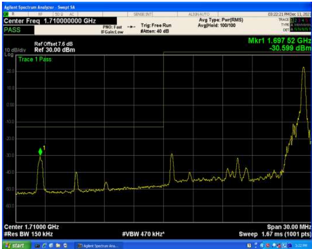
Band4 QPSK BW=15MHz Channel=20025 RB Size=75 Position=#0
