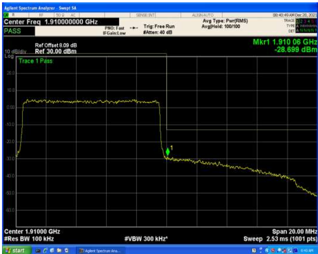
Band2 QPSK BW=15MHz Channel=18675 RB Size=1 Position=#Max
