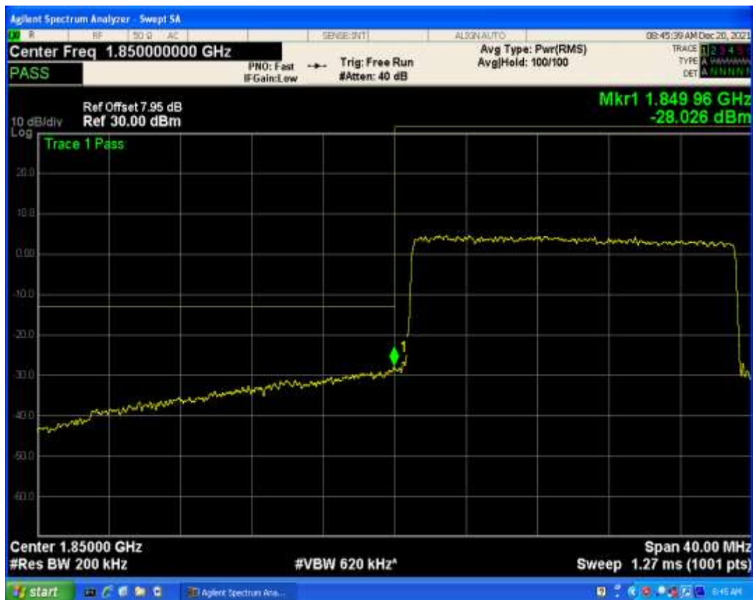
Band2 QPSK BW=20MHz Channel=19100 RB Size=1 Position=#Max
