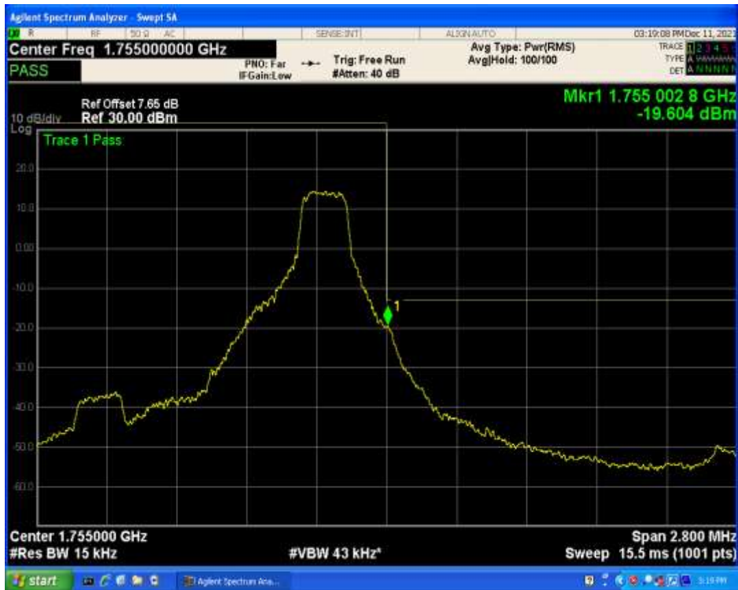
Band4 QPSK BW=1.4MHz Channel=20393 RB Size=6 Position=#0
