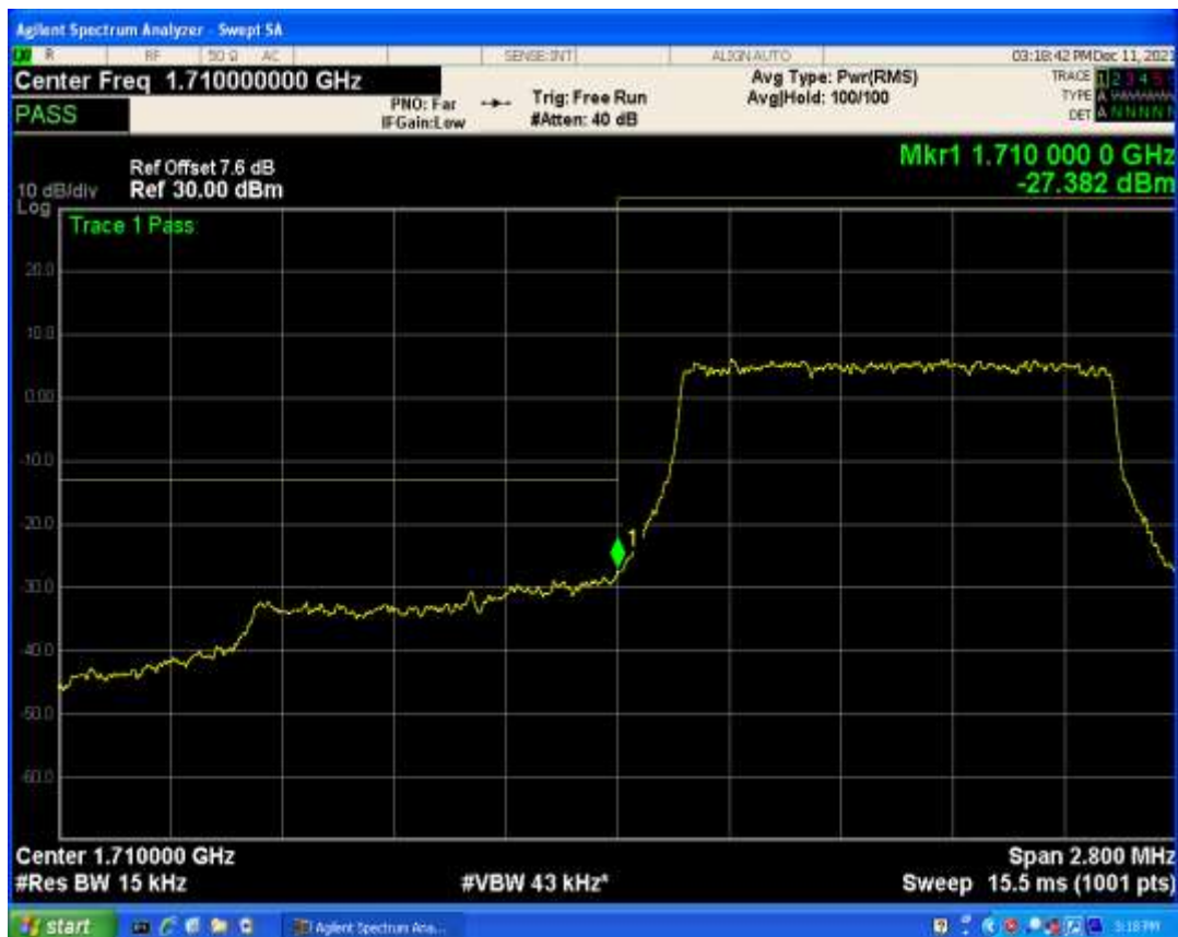
Band4 QAM16 BW=1.4MHz Channel=19957 RB Size=1 Position=#0
