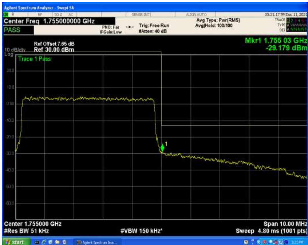
Band4 QPSK BW=10MHz Channel=20000 RB Size=1 Position=#Max
