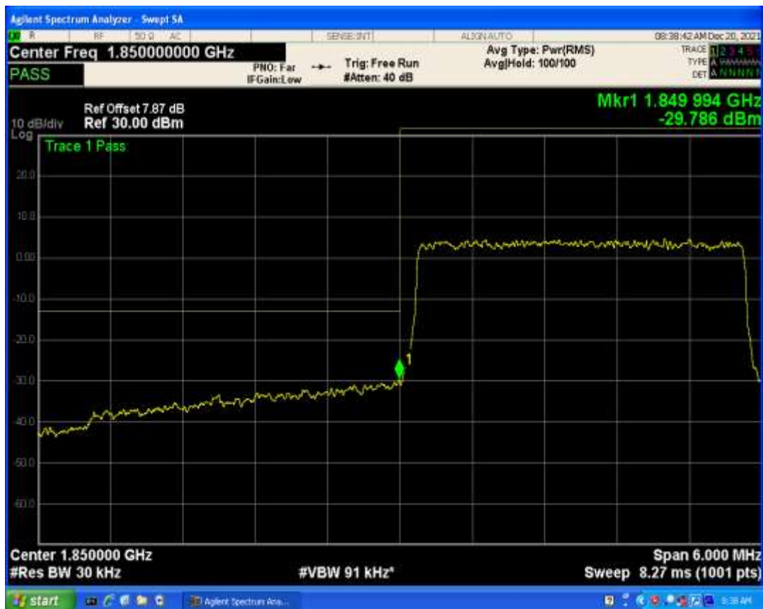
Band2 QPSK BW=3MHz Channel=19185 RB Size=1 Position=#Max
