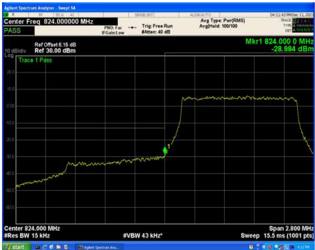
Band5 QAM16 BW=1.4MHz Channel=20407 RB Size=1 Position=#0
