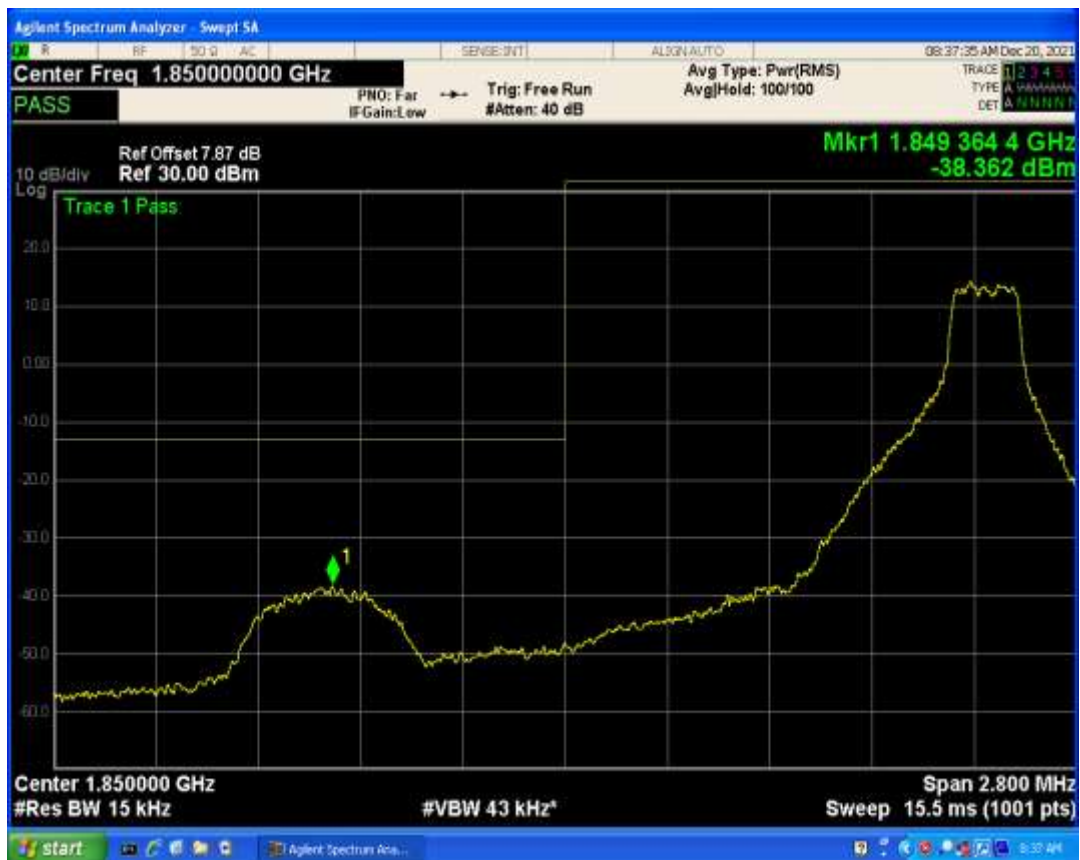
Band2 QPSK BW=1.4MHz Channel=19193 RB Size=1 Position=#0
