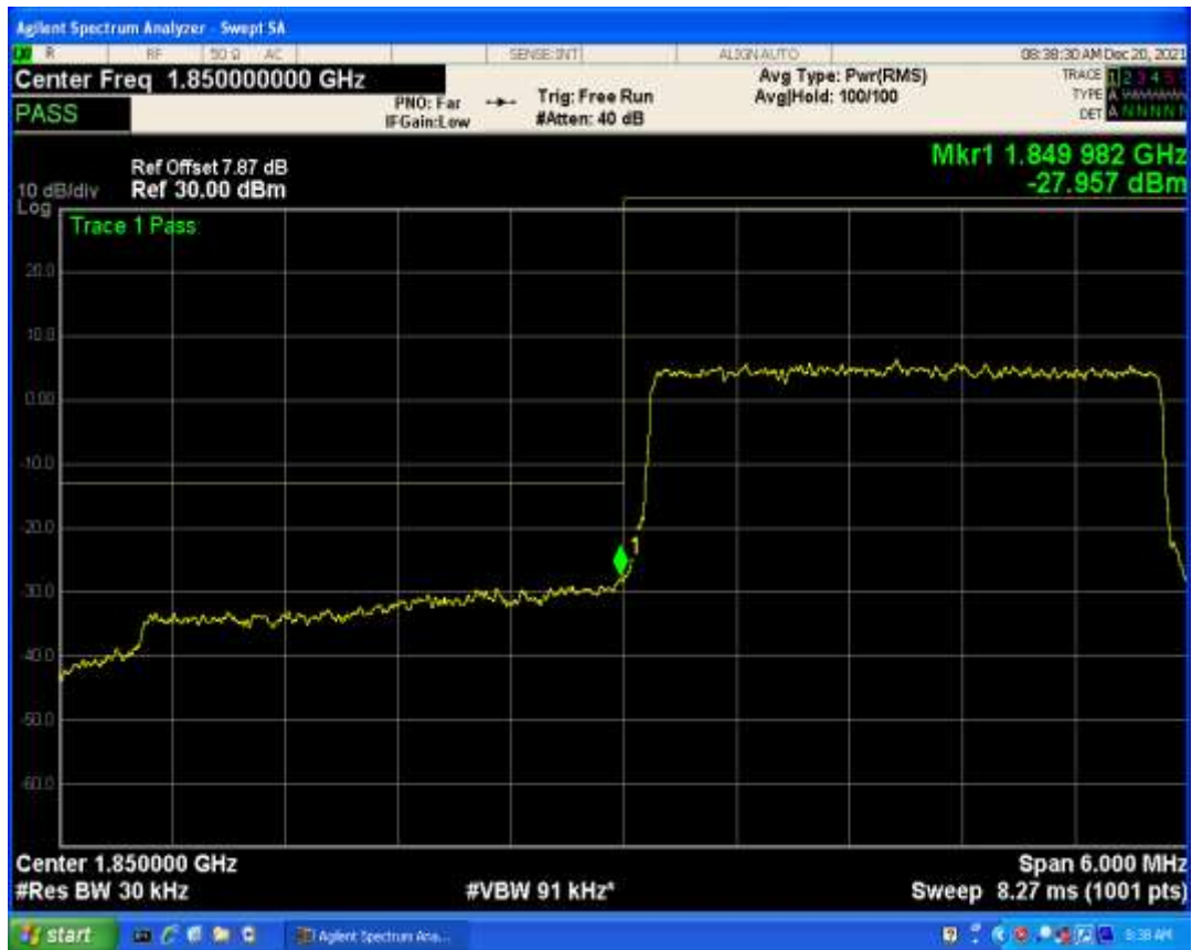
Band2 QAM16 BW=3MHz Channel=18615 RB Size=1 Position=#Max
