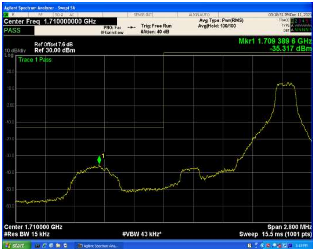
Band4 QAM16 BW=1.4MHz Channel=19957 RB Size=6 Position=#0
