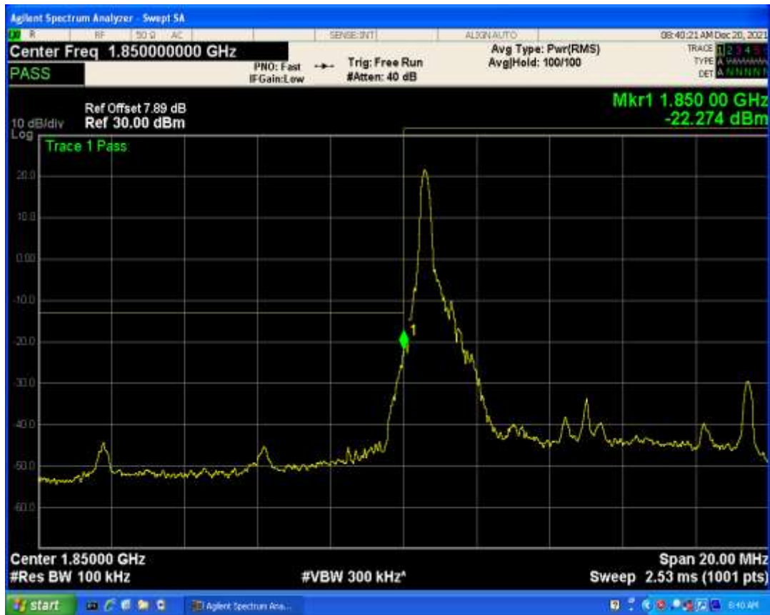
Band2 QAM16 BW=10MHz Channel=18650 RB Size=1 Position=#Max
