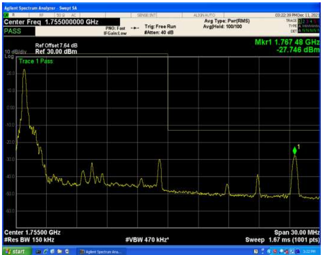
Band4 QPSK BW=15MHz Channel=20325 RB Size=1 Position=#Max
