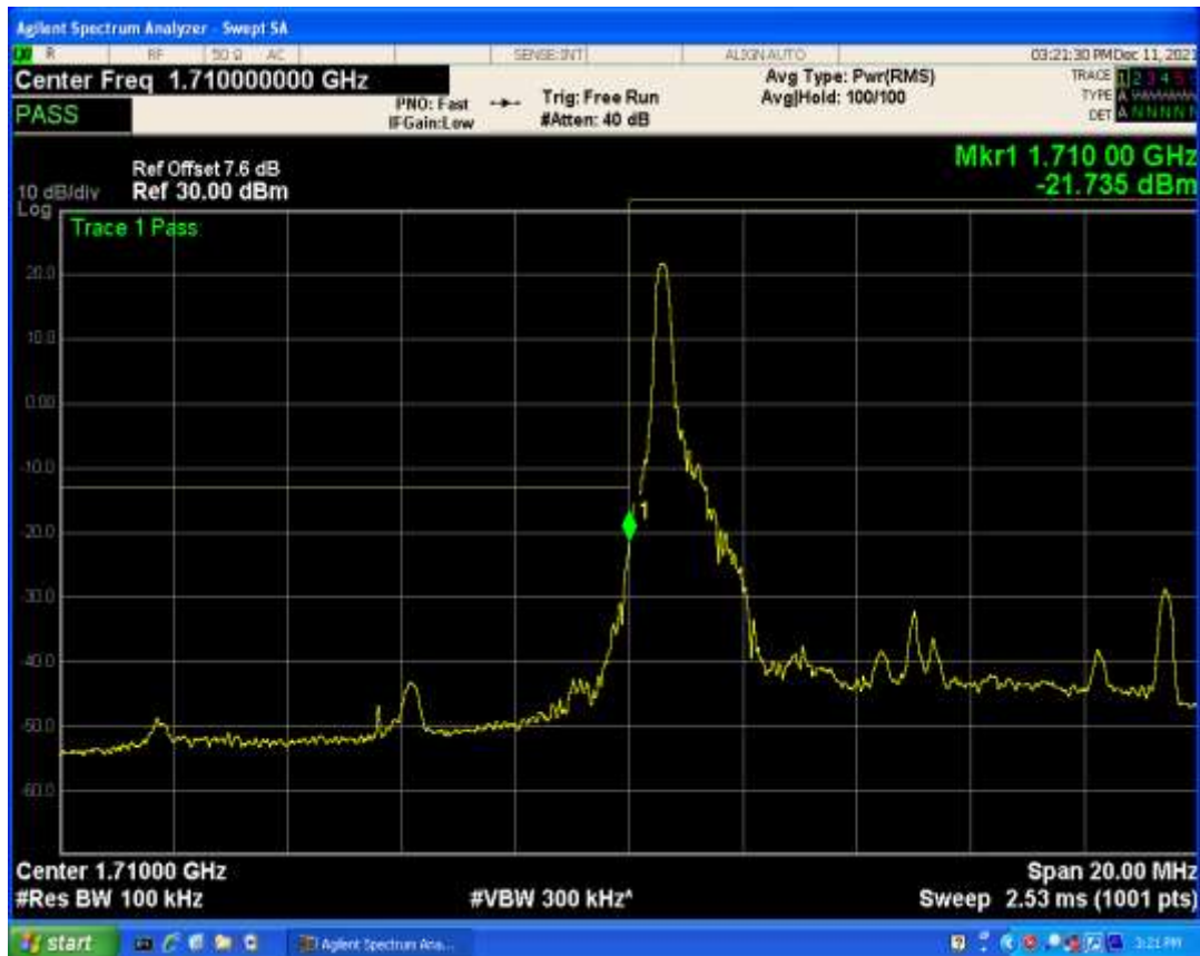
Band4 QAM16 BW=5MHz Channel=20375 RB Size=25 Position=#0
