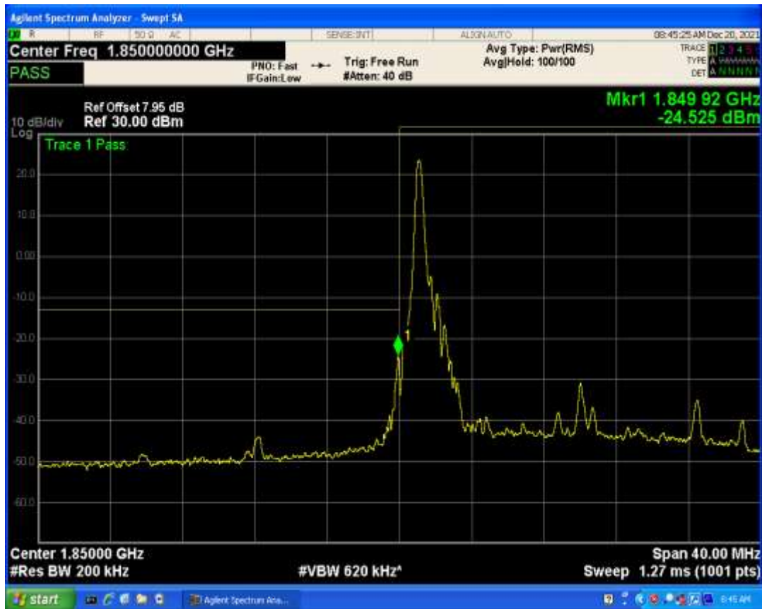
Band2 QAM16 BW=15MHz Channel=19125 RB Size=75 Position=#0
