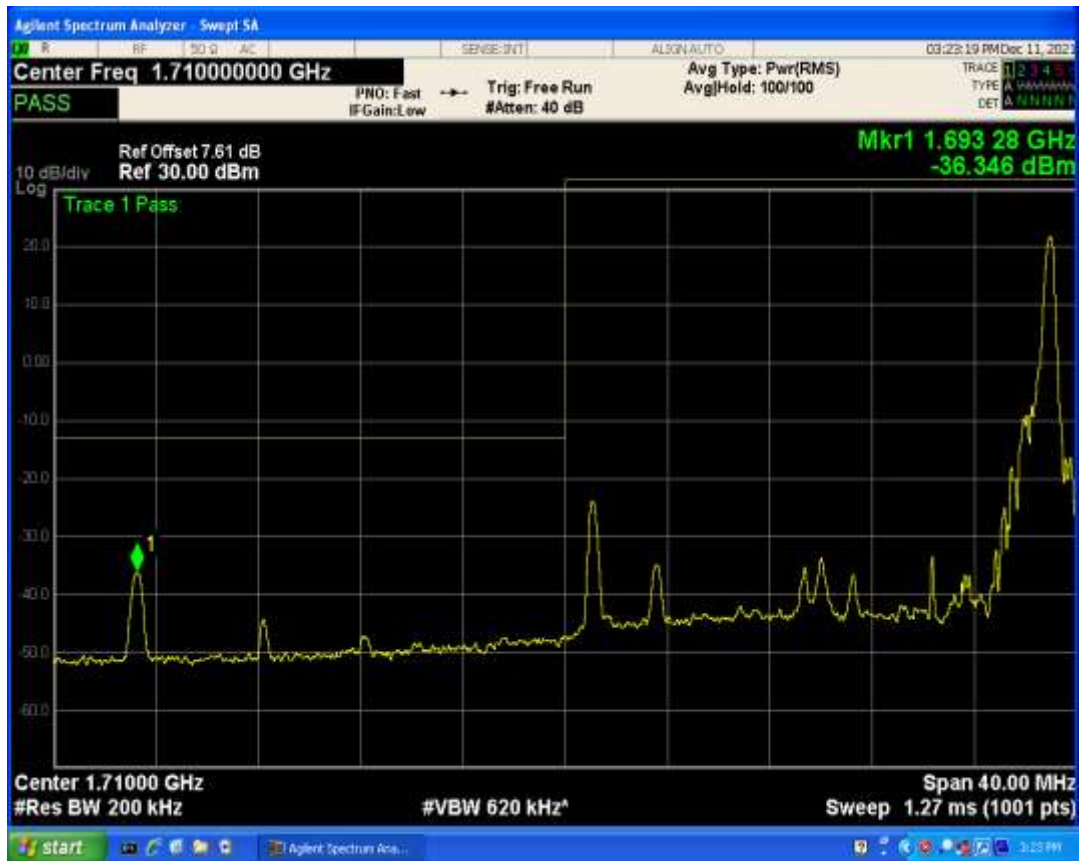
Band4 QAM16 BW=20MHz Channel=20050 RB Size=1 Position=#0
