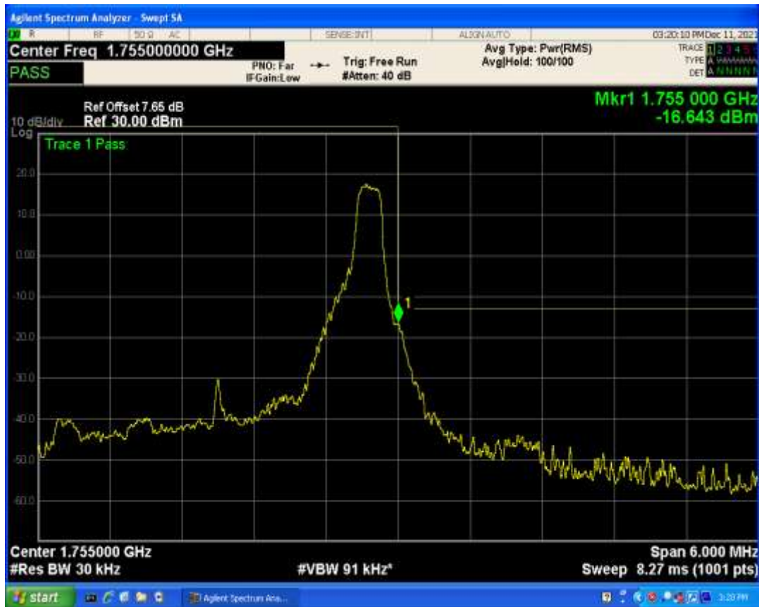
Band4 QPSK BW=3MHz Channel=20385 RB Size=15 Position=#0
