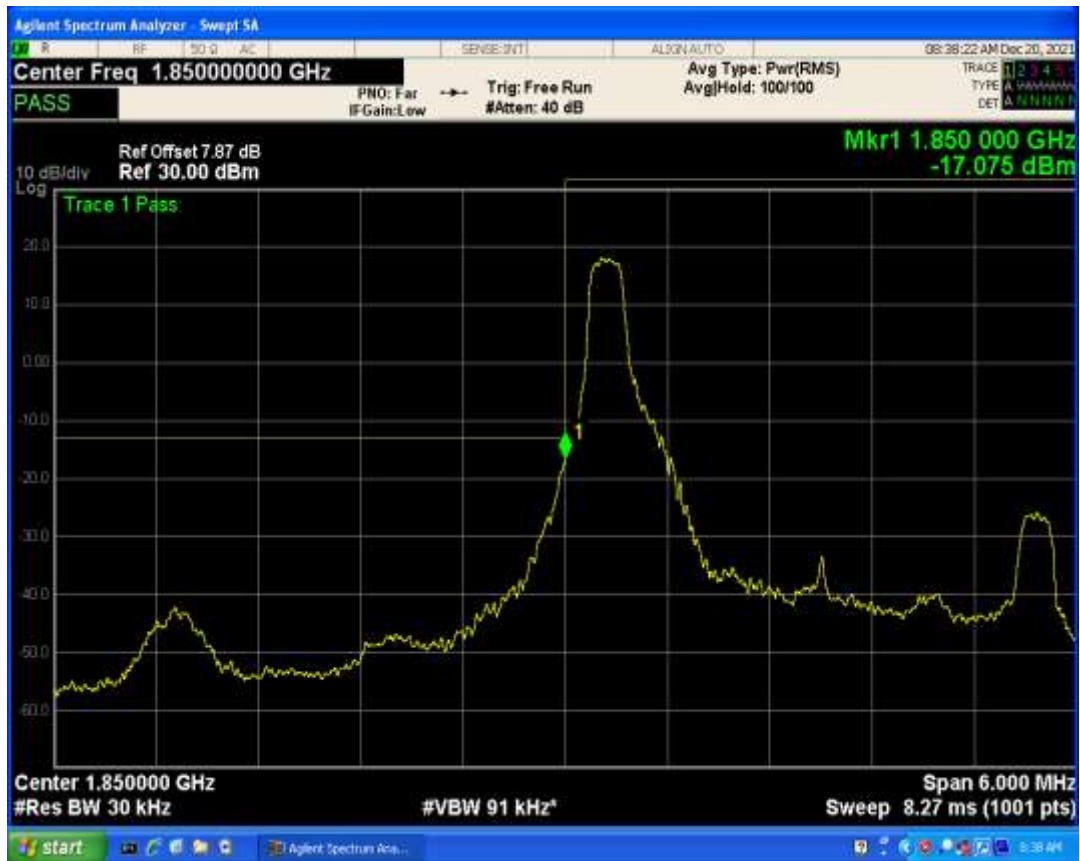
Band2 QAM16 BW=1.4MHz Channel=19193 RB Size=6 Position=#0
