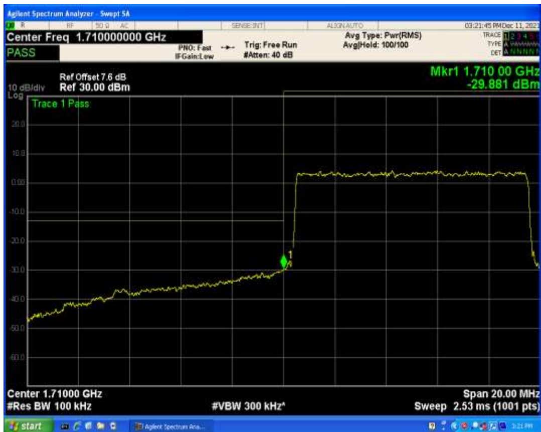
Band4 QPSK BW=10MHz Channel=20350 RB Size=1 Position=#Max
