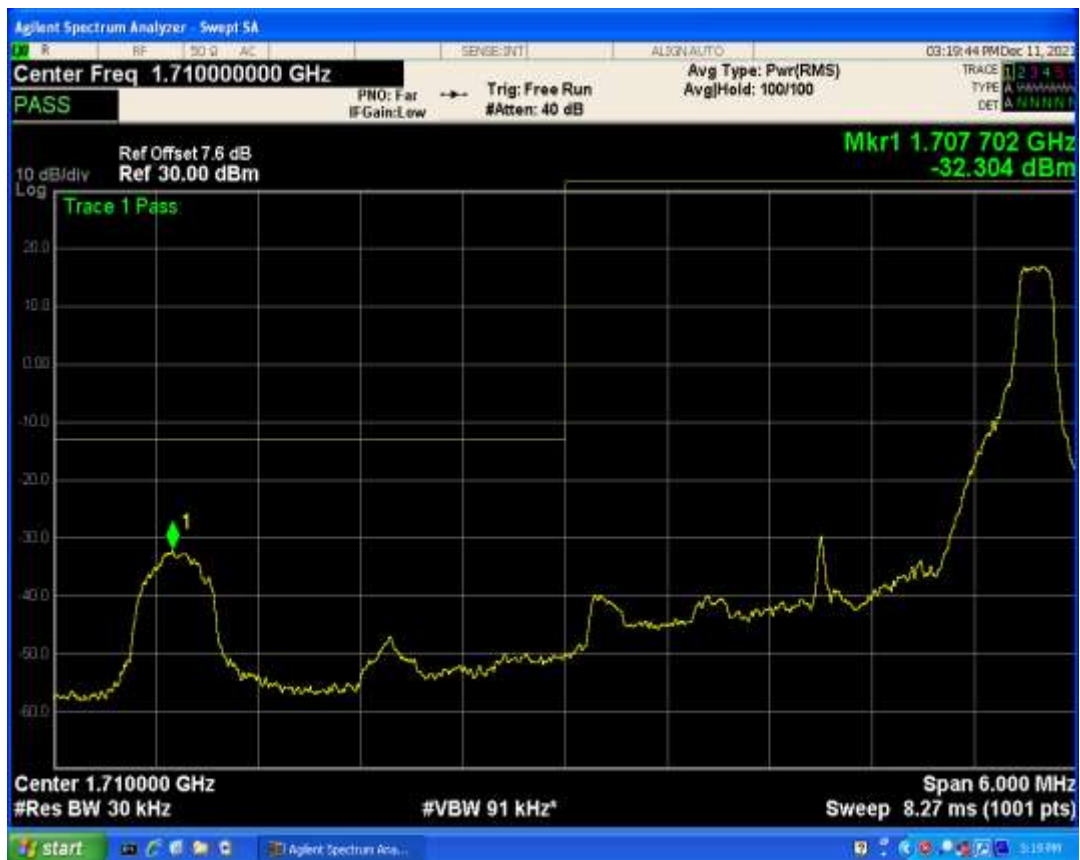
Band4 QPSK BW=3MHz Channel=19965 RB Size=1 Position=#0
