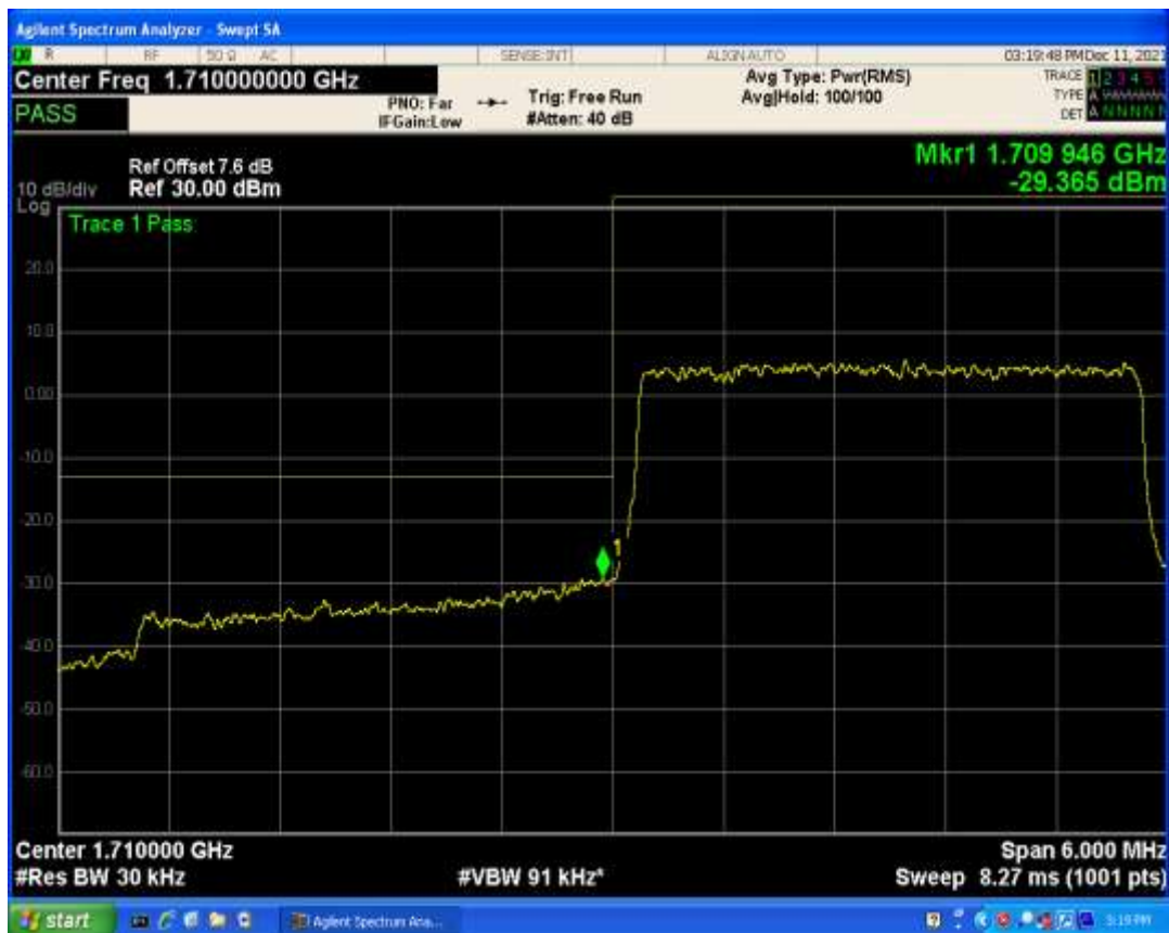
Band4 QAM16 BW=3MHz Channel=19965 RB Size=1 Position=#0
