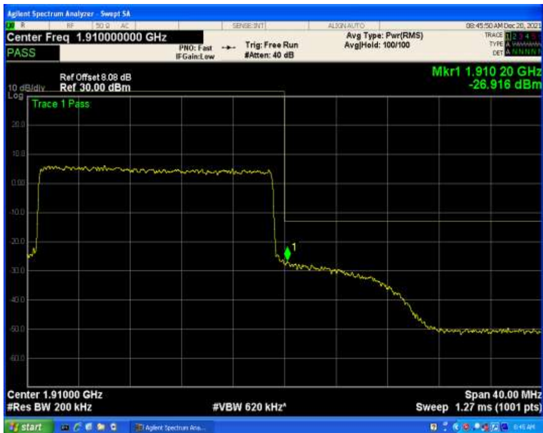
Band2 QAM16 BW=20MHz Channel=19100 RB Size=1 Position=#0
