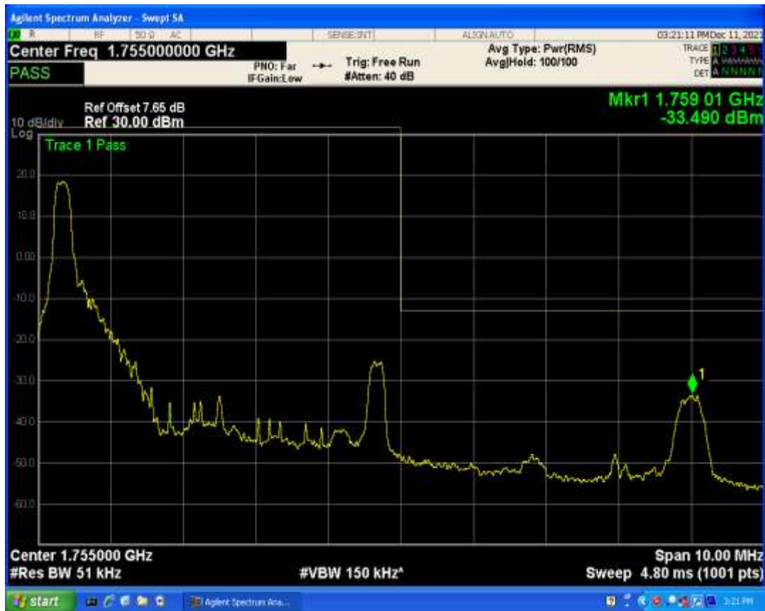
Band4 QAM16 BW=5MHz Channel=20375 RB Size=1 Position=#Max
