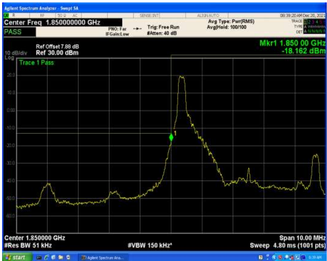
Band2 QPSK BW=5MHz Channel=18625 RB Size=1 Position=#Max
