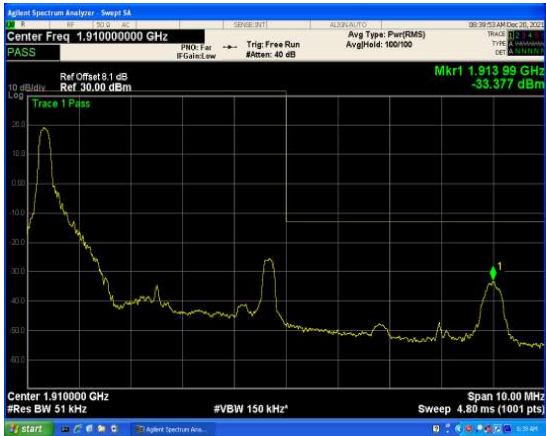
Band2 QAM16 BW=5MHz Channel=19175 RB Size=1 Position=#Max
