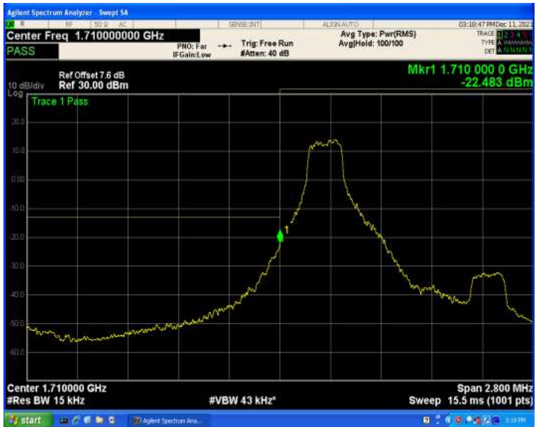
Band4 QAM16 BW=1.4MHz Channel=19957 RB Size=1 Position=#Max
