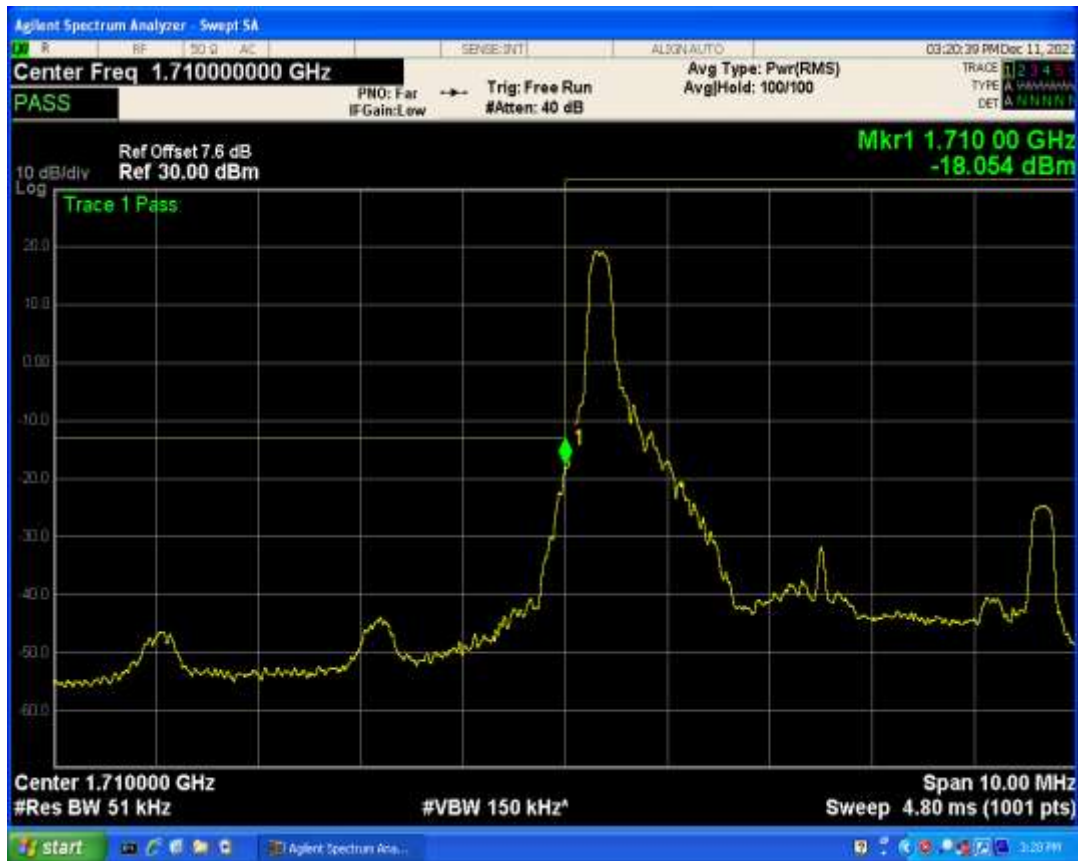
Band4 QPSK BW=5MHz Channel=19975 RB Size=25 Position=#0
