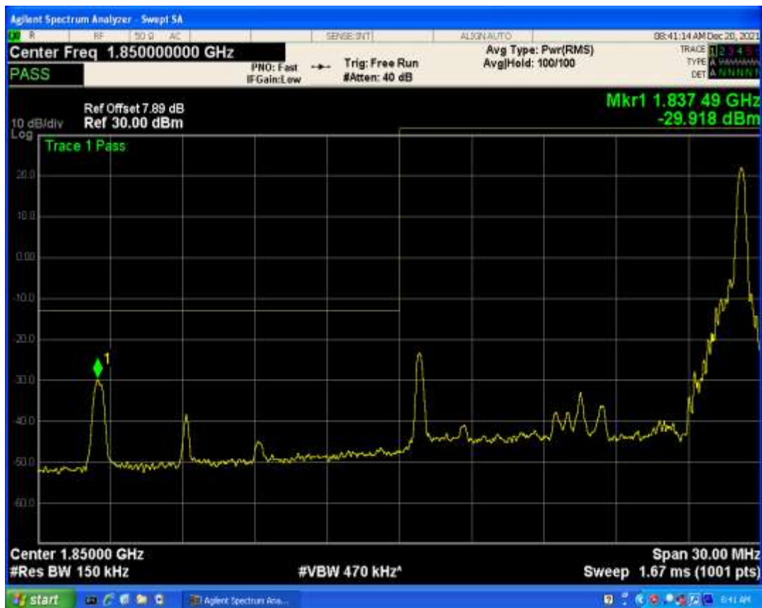
Band2 QAM16 BW=15MHz Channel=18675 RB Size=75 Position=#0
