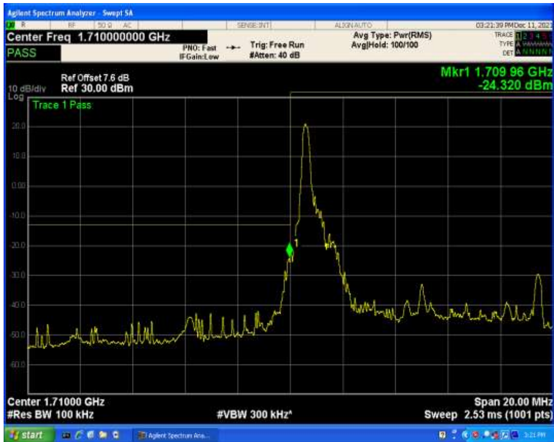
Band4 QAM16 BW=10MHz Channel=20000 RB Size=1 Position=#Max
