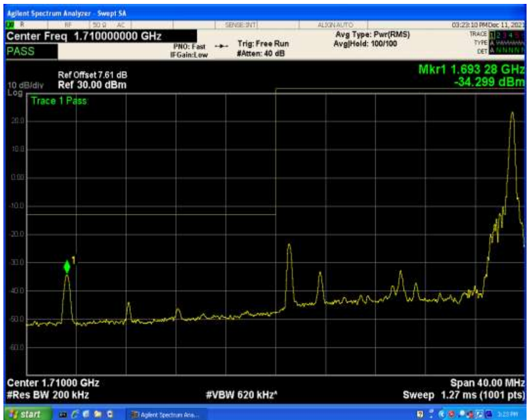
Band4 QPSK BW=20MHz Channel=20050 RB Size=1 Position=#0
