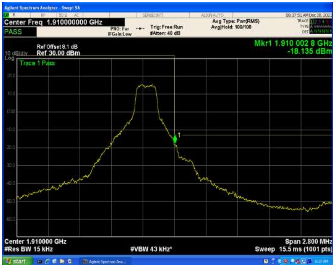
Band2 QPSK BW=1.4MHz Channel=19193 RB Size=6 Position=#0
