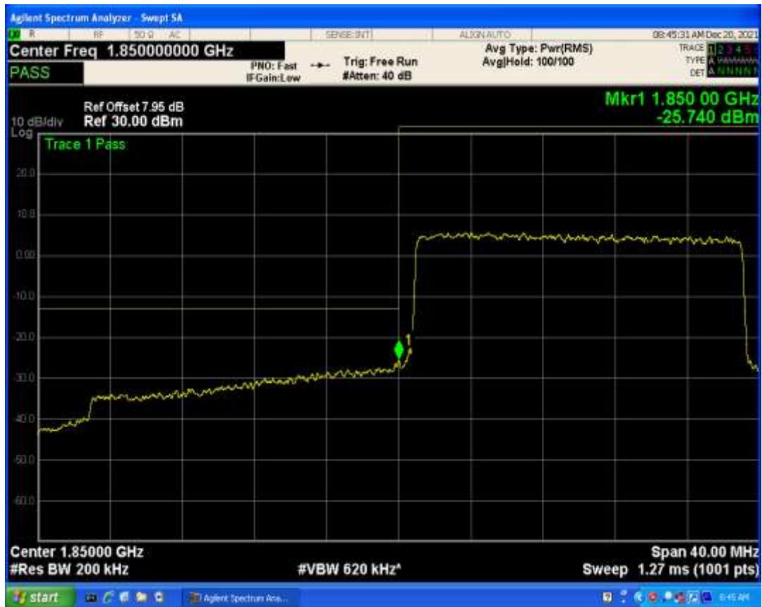
Band2 QAM16 BW=20MHz Channel=18700 RB Size=1 Position=#Max
