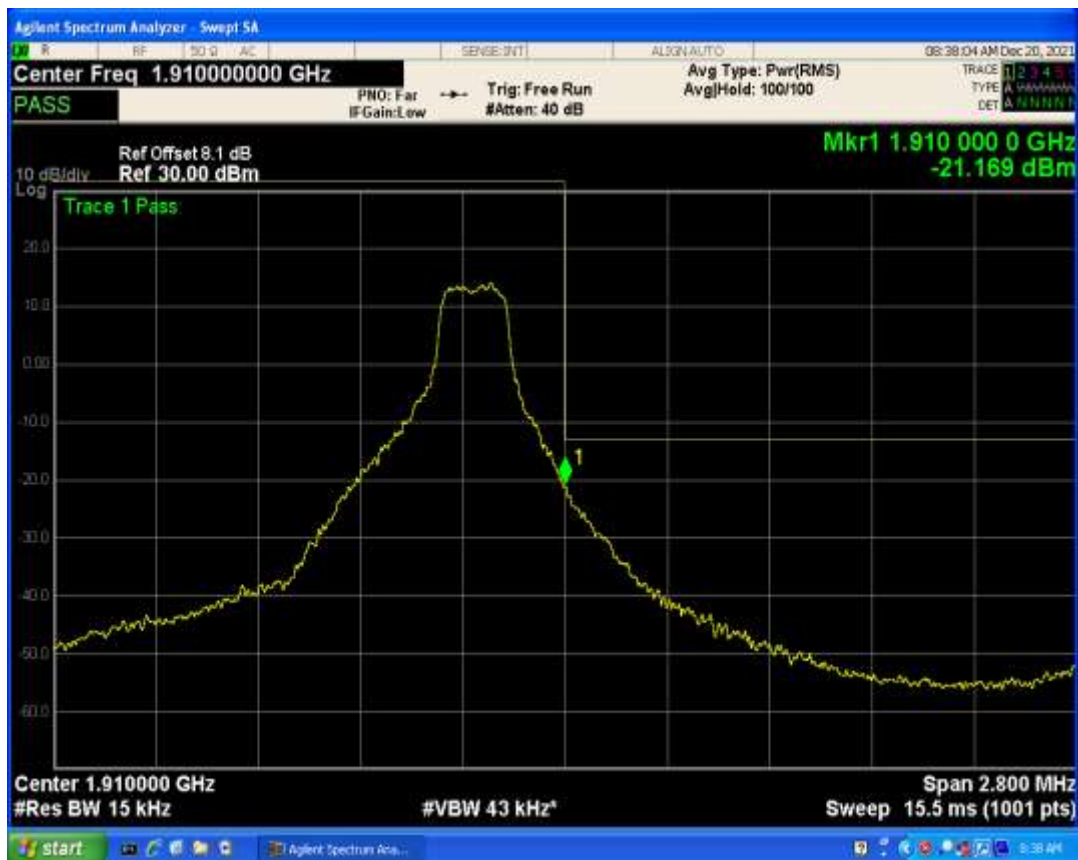
Band2 QPSK BW=3MHz Channel=18615 RB Size=1 Position=#0
