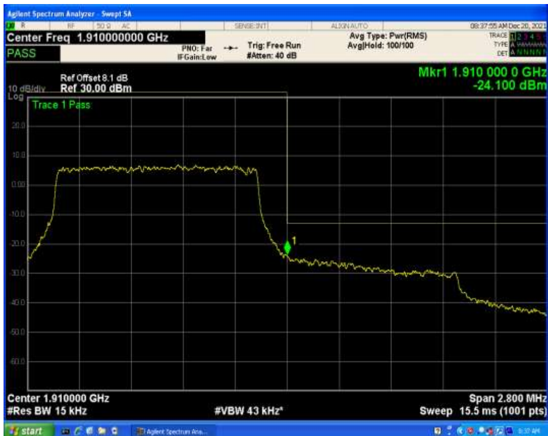
Band2 QAM16 BW=1.4MHz Channel=19193 RB Size=1 Position=#0
