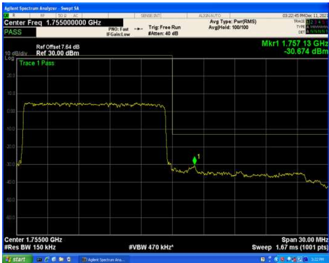
Band4 QAM16 BW=15MHz Channel=20325 RB Size=1 Position=#Max
