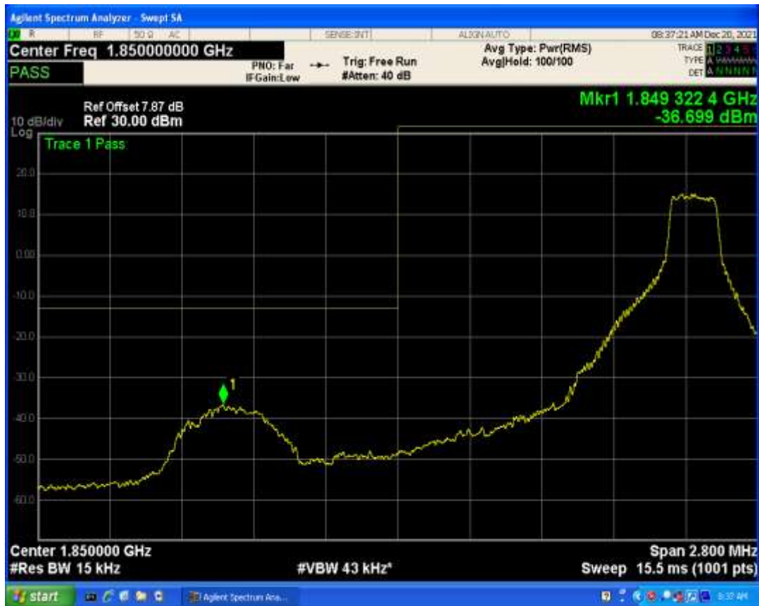
Band2 QAM16 BW=1.4MHz Channel=18607 RB Size=1 Position=#0
