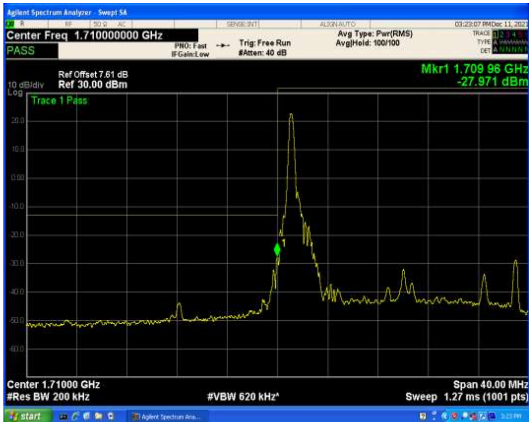
Band4 QPSK BW=20MHz Channel=20050 RB Size=100 Position=#0
