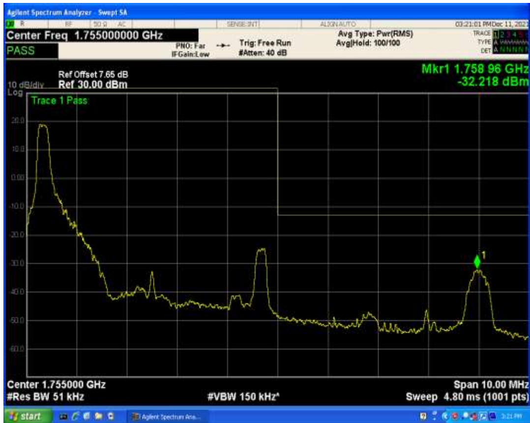
Band4 QAM16 BW=5MHz Channel=19975 RB Size=25 Position=#0
