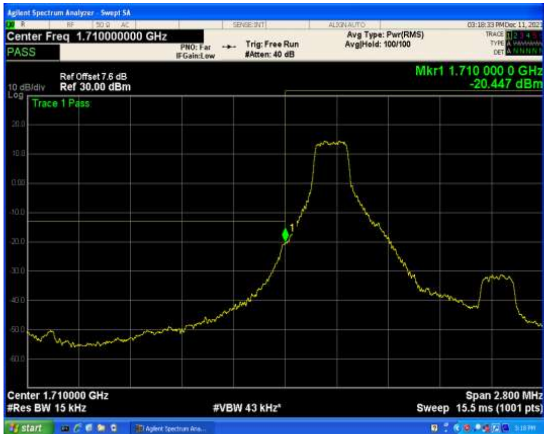
Band4 QPSK BW=1.4MHz Channel=19957 RB Size=6 Position=#0
