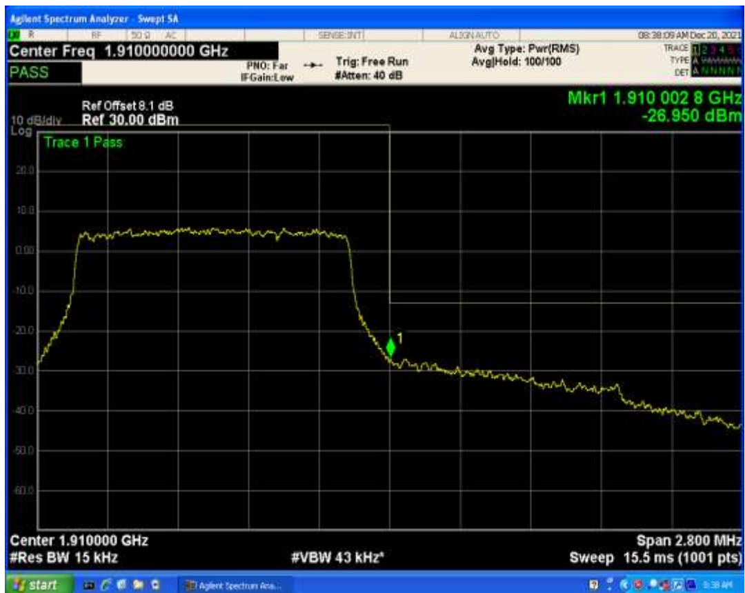
Band2 QPSK BW=3MHz Channel=18615 RB Size=1 Position=#Max
