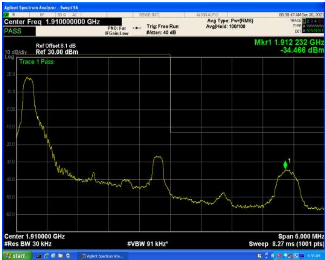
Band2 QAM16 BW=3MHz Channel=18615 RB Size=15 Position=#0
