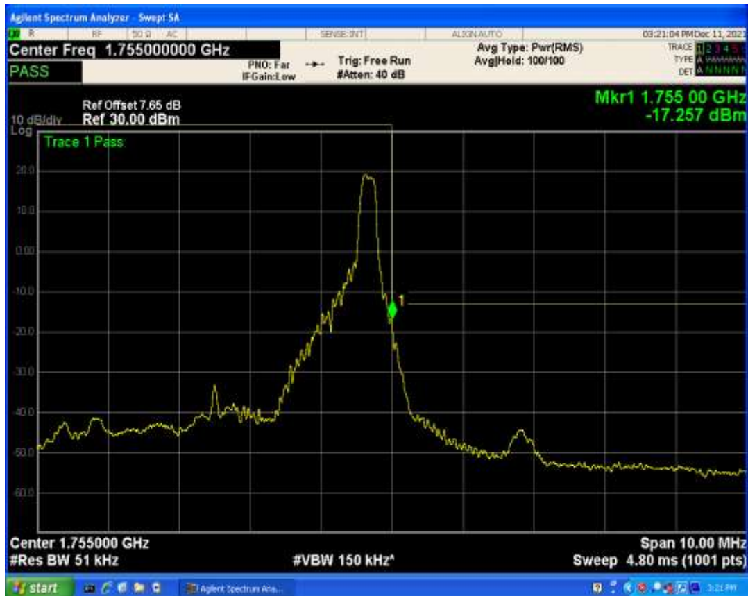
Band4 QPSK BW=5MHz Channel=20375 RB Size=25 Position=#0
