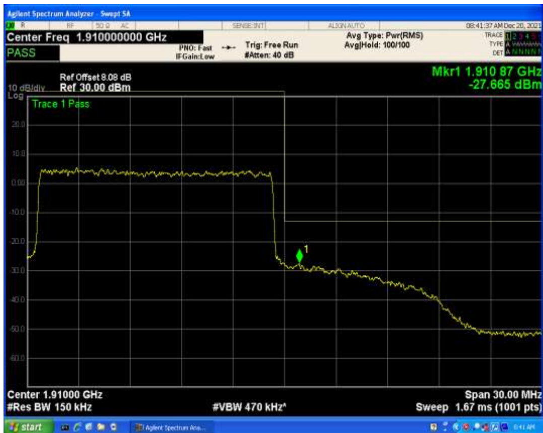
Band2 QPSK BW=20MHz Channel=18700 RB Size=1 Position=#Max
