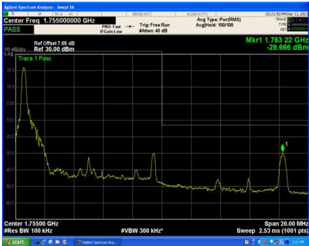
Band4 QAM16 BW=10MHz Channel=20000 RB Size=50 Position=#0
