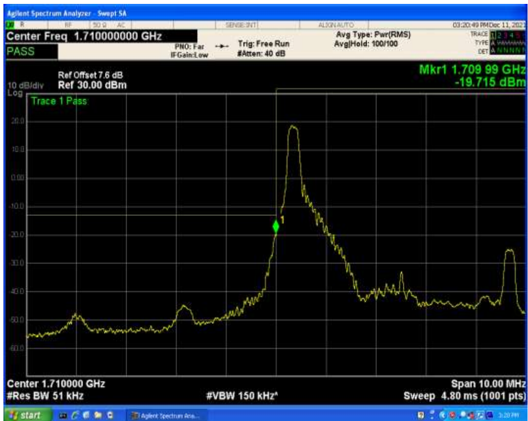
Band4 QPSK BW=5MHz Channel=20375 RB Size=1 Position=#0
