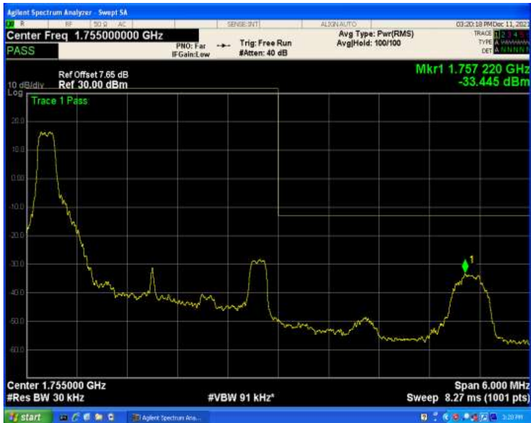
Band4 QAM16 BW=3MHz Channel=20385 RB Size=1 Position=#Max
