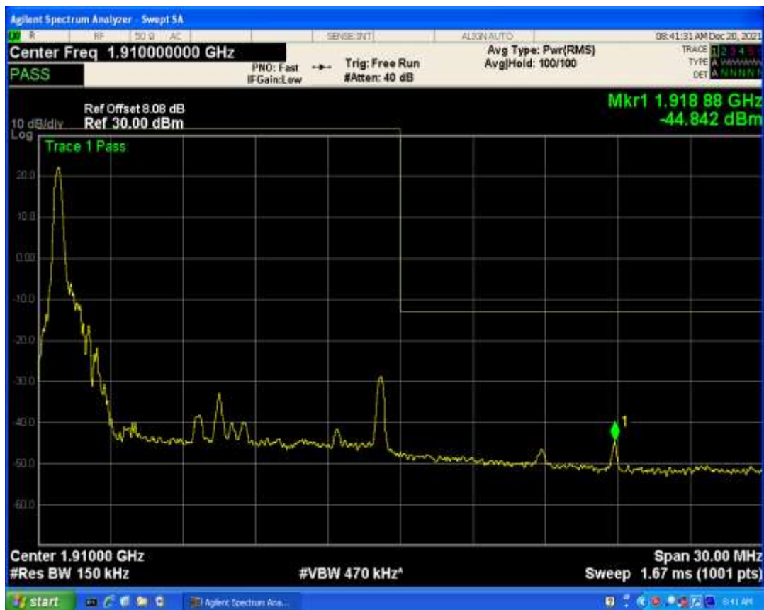
Band2 QPSK BW=15MHz Channel=19125 RB Size=75 Position=#0
