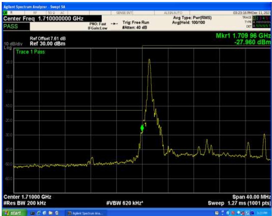
Band4 QAM16 BW=20MHz Channel=20050 RB Size=100 Position=#0
