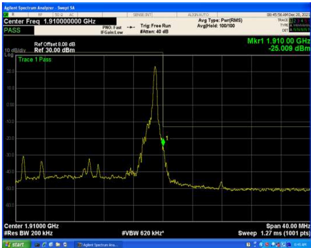
Band2 QAM16 BW=20MHz Channel=19100 RB Size=100 Position=#0
