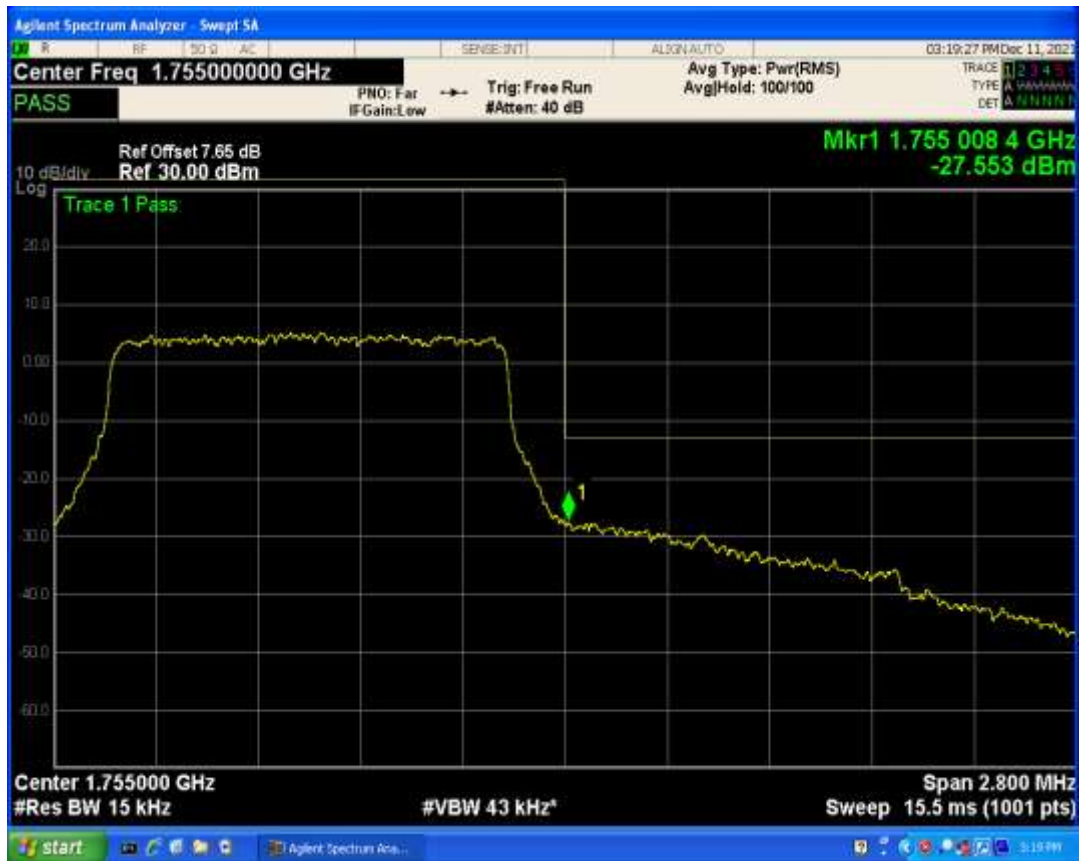
Band4 QPSK BW=3MHz Channel=19965 RB Size=1 Position=#Max
