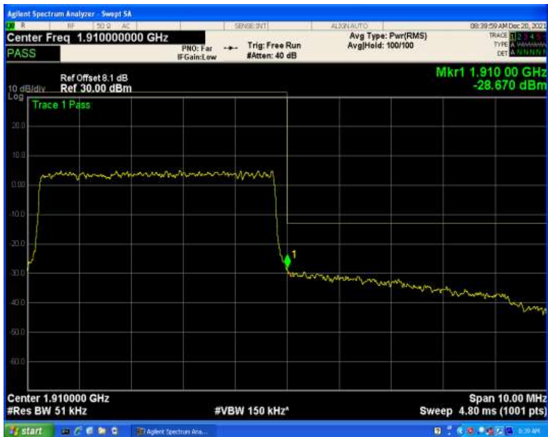
Band2 QPSK BW=10MHz Channel=18650 RB Size=1 Position=#Max
