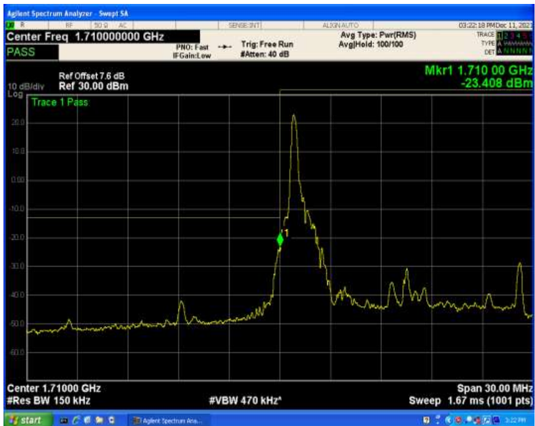
Band4 QPSK BW=15MHz Channel=20025 RB Size=1 Position=#Max
