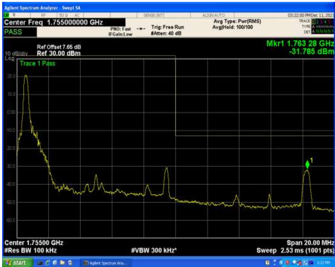
Band4 QAM16 BW=10MHz Channel=20350 RB Size=1 Position=#Max
