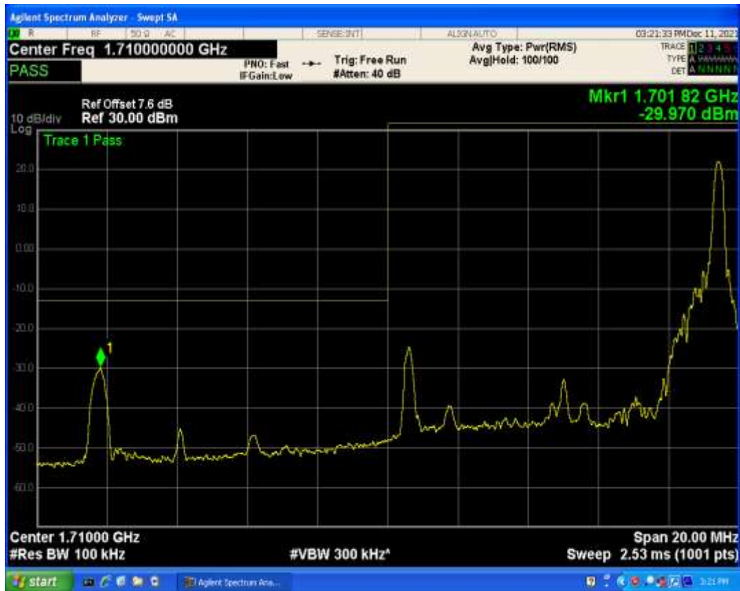
Band4 QPSK BW=10MHz Channel=20000 RB Size=50 Position=#0
