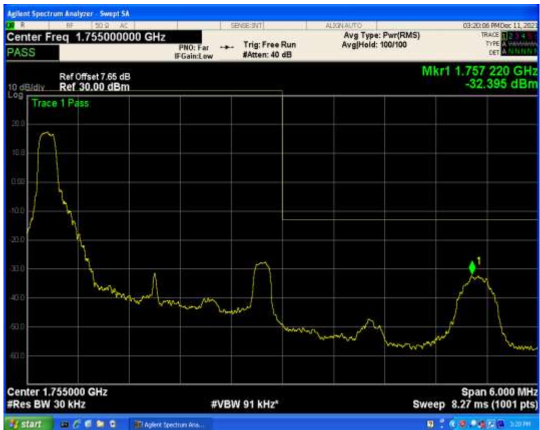
Band4 QPSK BW=3MHz Channel=20385 RB Size=1 Position=#Max
