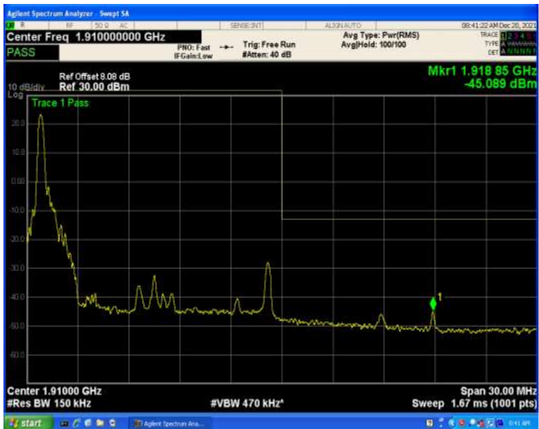
Band2 QPSK BW=15MHz Channel=19125 RB Size=1 Position=#Max
