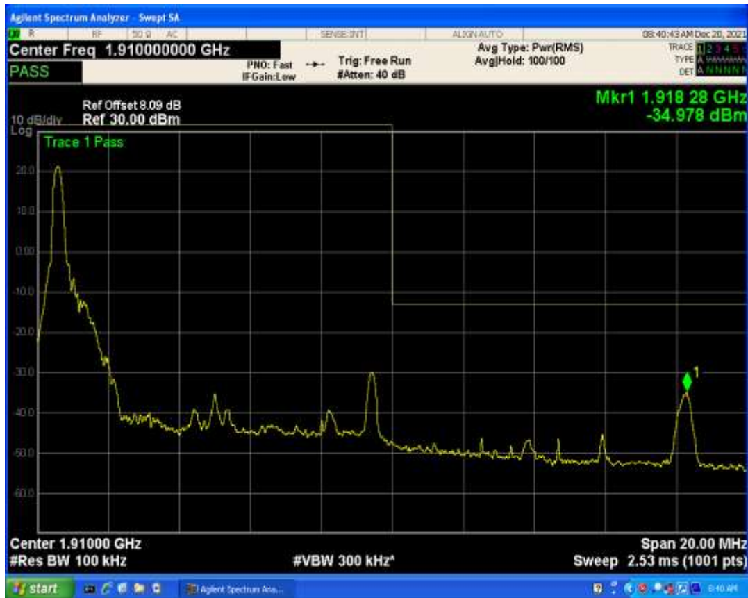
Band2 QAM16 BW=10MHz Channel=19150 RB Size=1 Position=#Max
