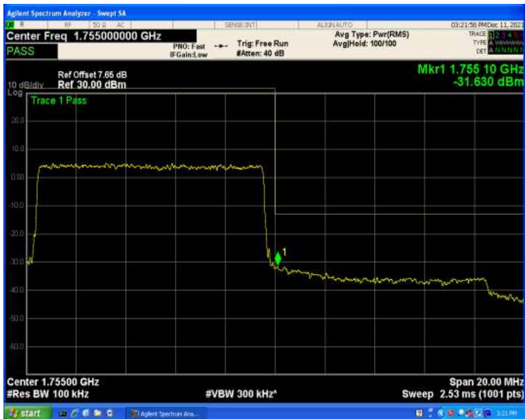
Band4 QAM16 BW=10MHz Channel=20350 RB Size=1 Position=#0
