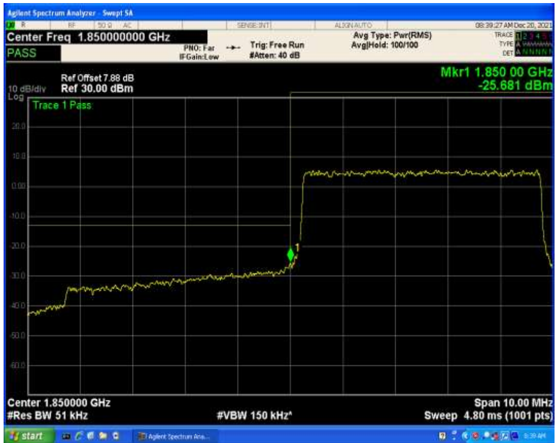
Band2 QAM16 BW=5MHz Channel=18625 RB Size=1 Position=#Max
