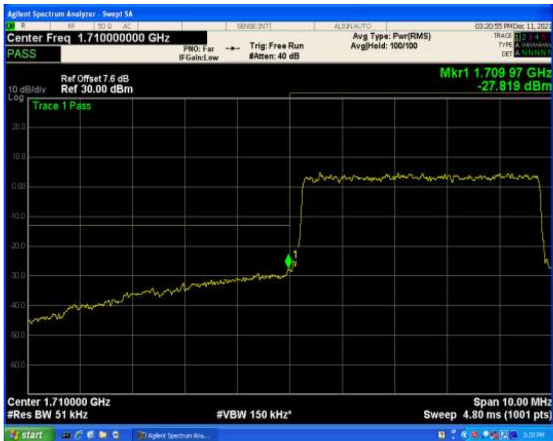
Band4 QPSK BW=5MHz Channel=20375 RB Size=1 Position=#Max
