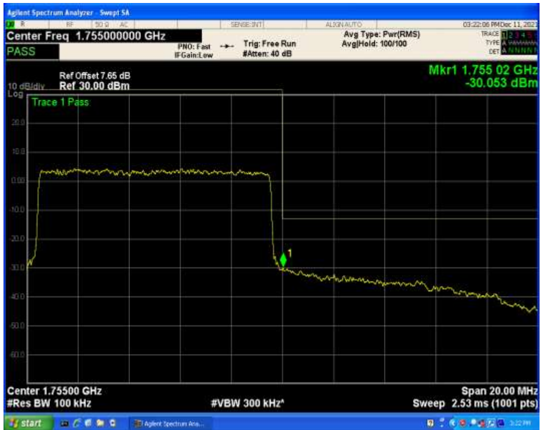
Band4 QPSK BW=15MHz Channel=20025 RB Size=1 Position=#0
