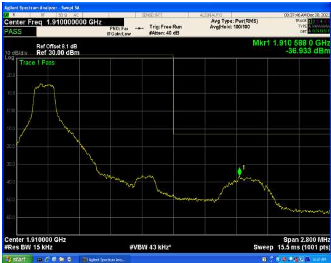
Band2 QAM16 BW=1.4MHz Channel=18607 RB Size=6 Position=#0
