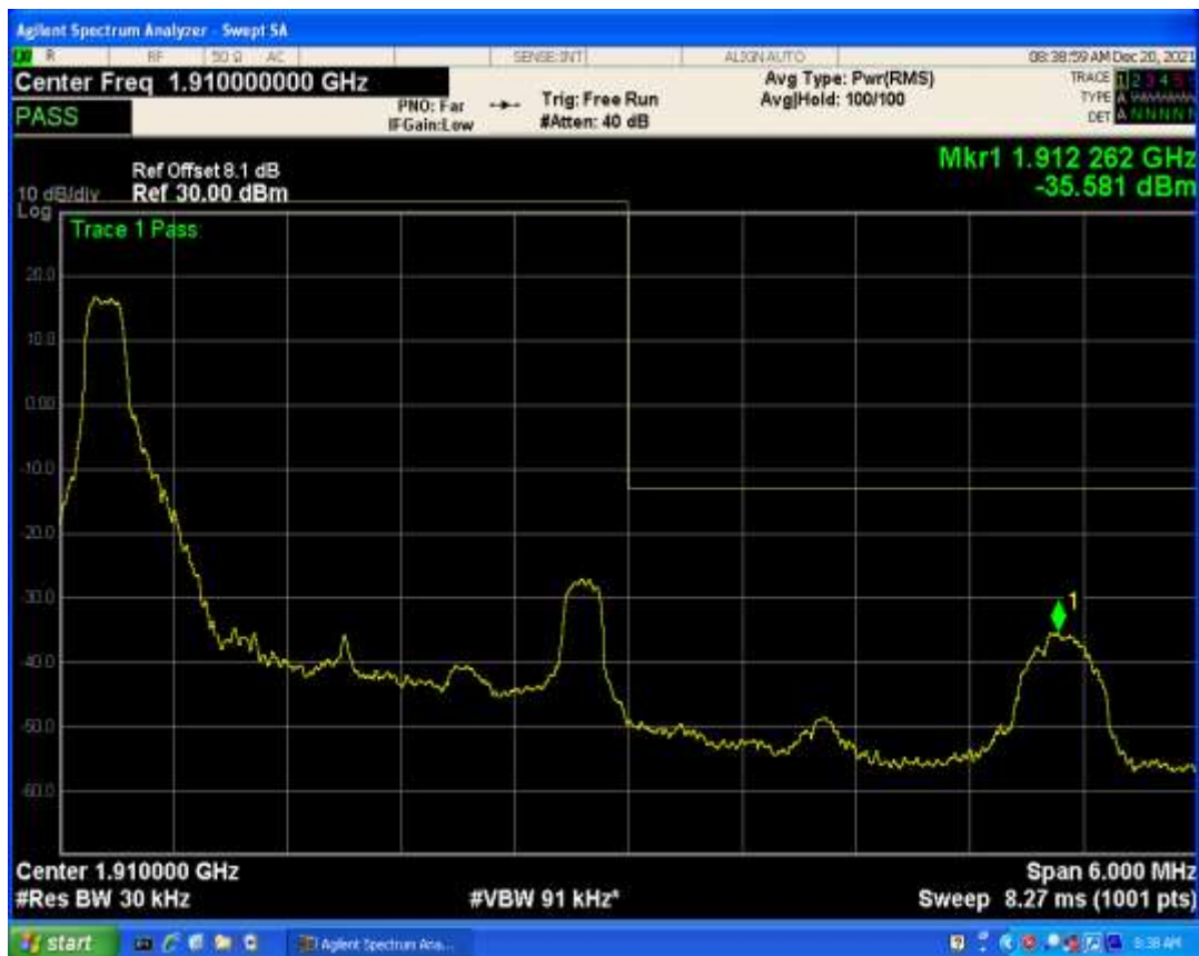
Band2 QPSK BW=3MHz Channel=19185 RB Size=15 Position=#0
