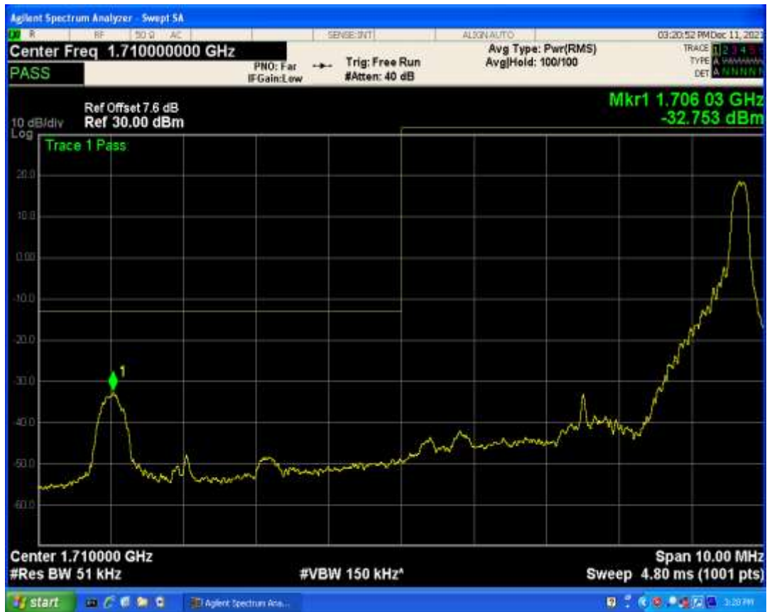
Band4 QAM16 BW=5MHz Channel=19975 RB Size=1 Position=#0
