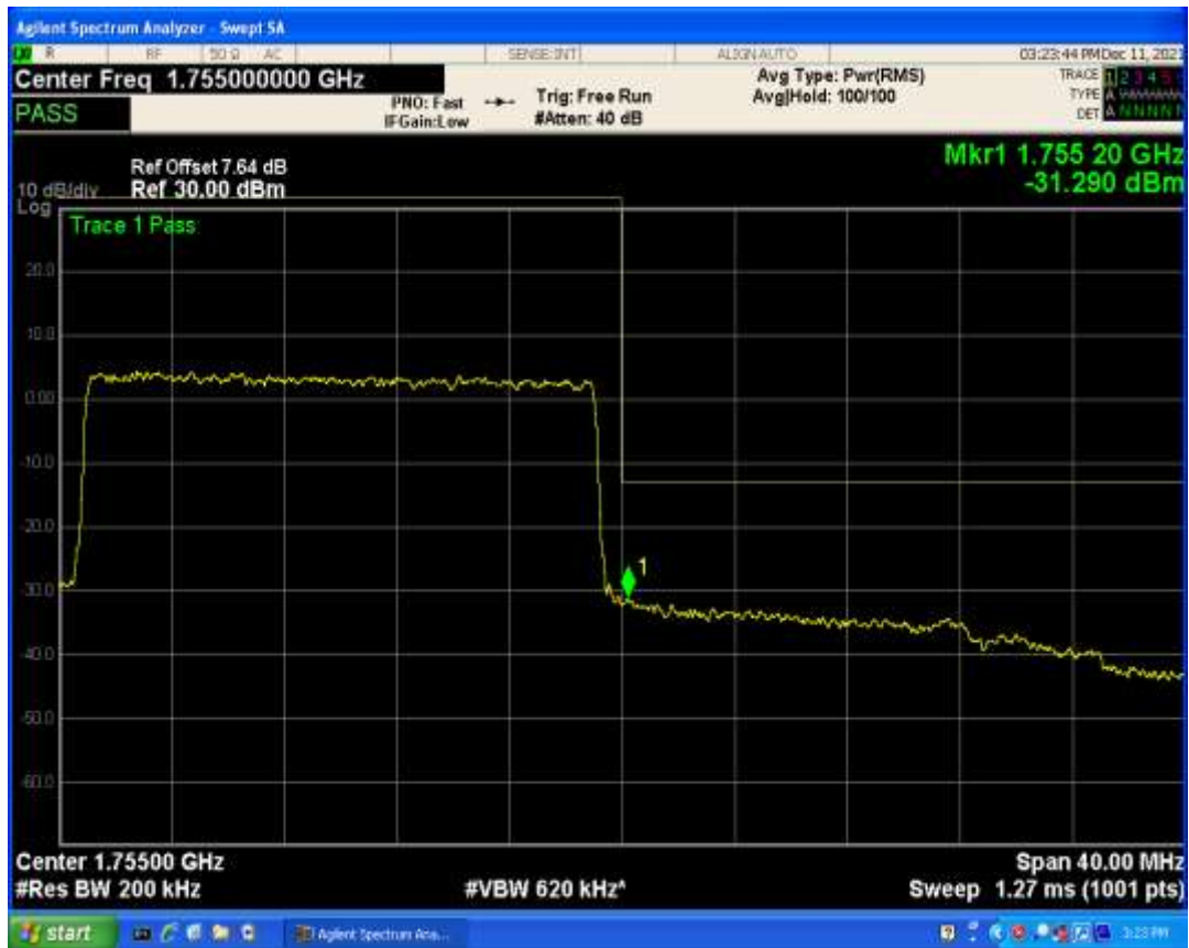
Band5 QPSK BW=1.4MHz Channel=20407 RB Size=1 Position=#Max
