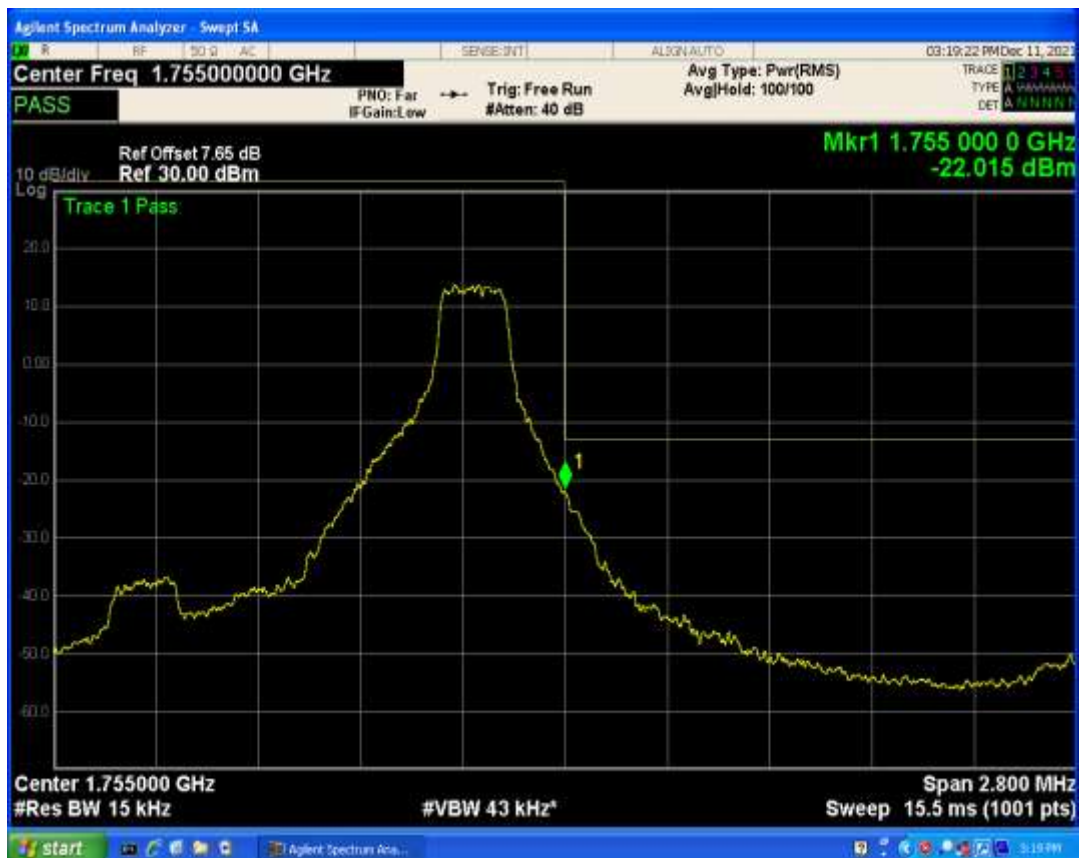
Band4 QAM16 BW=1.4MHz Channel=20393 RB Size=6 Position=#0
