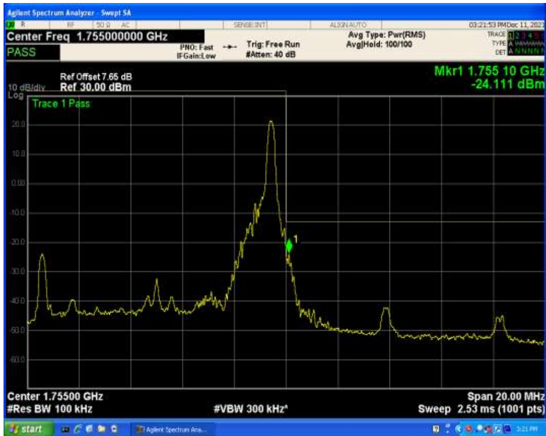
Band4 QPSK BW=10MHz Channel=20350 RB Size=50 Position=#0
