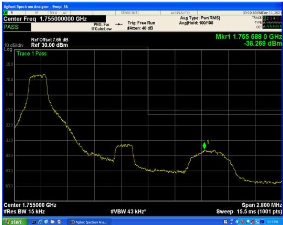
Band4 QAM16 BW=1.4MHz Channel=20393 RB Size=1 Position=#Max
