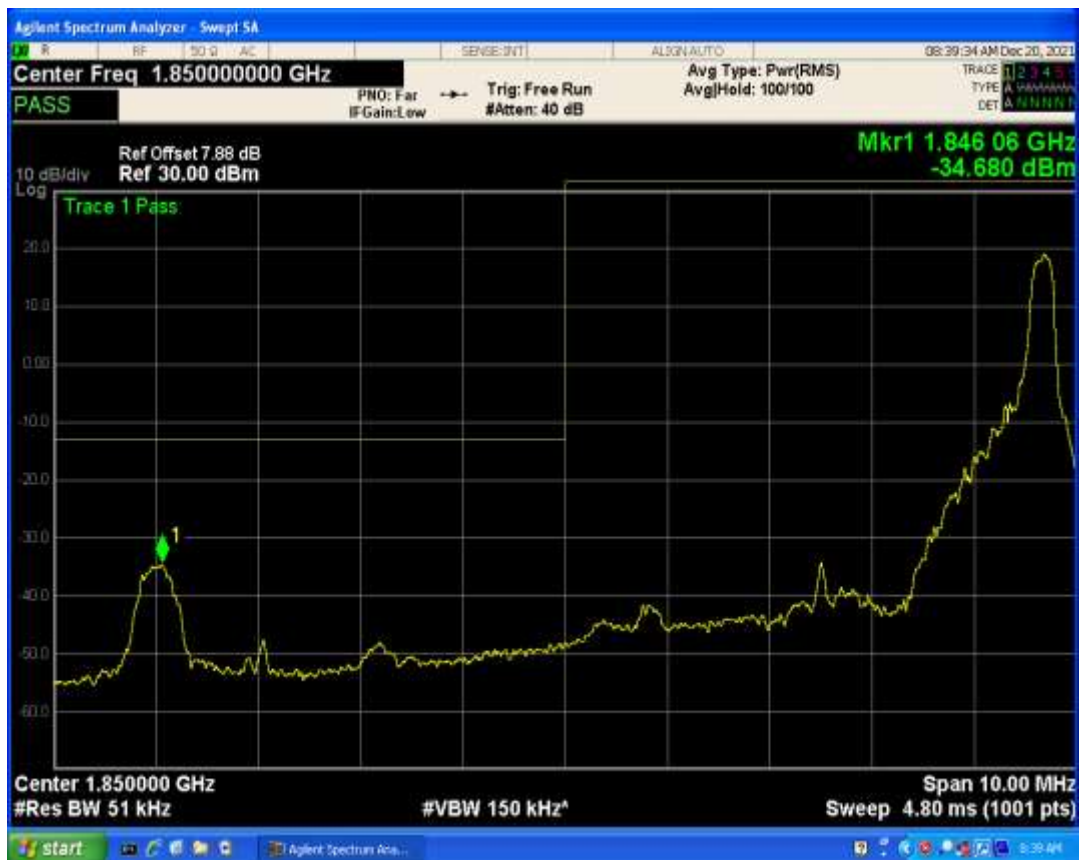
Band2 QAM16 BW=5MHz Channel=18625 RB Size=25 Position=#0
