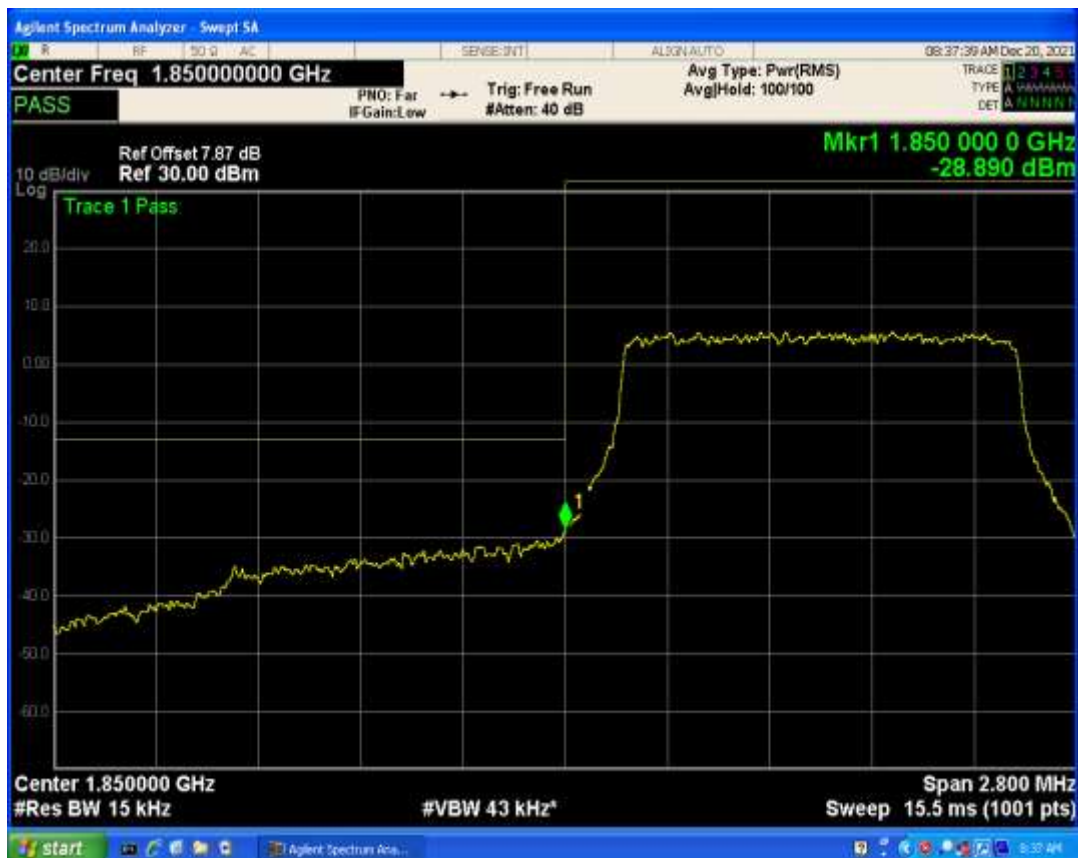
Band2 QPSK BW=1.4MHz Channel=19193 RB Size=1 Position=#Max
