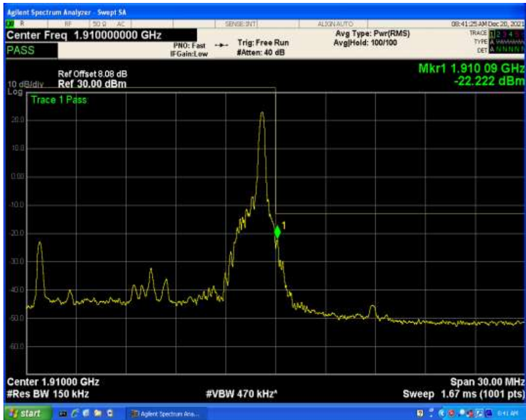
Band2 QAM16 BW=15MHz Channel=19125 RB Size=1 Position=#0
