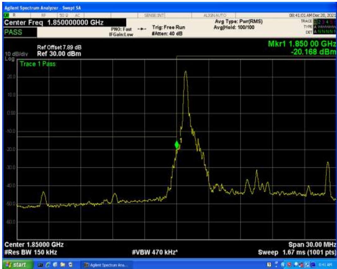
Band2 QAM16 BW=10MHz Channel=19150 RB Size=50 Position=#0
