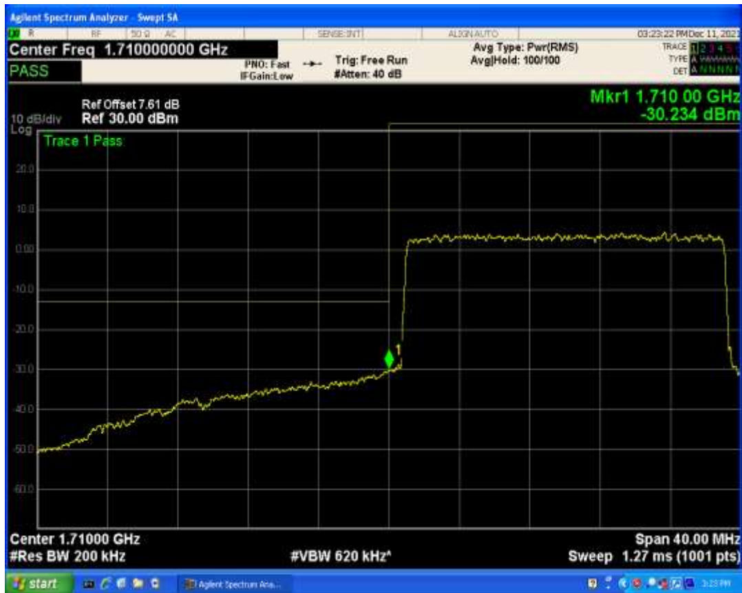
Band4 QPSK BW=20MHz Channel=20300 RB Size=1 Position=#0
