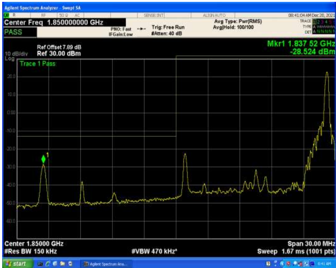
Band2 QAM16 BW=15MHz Channel=18675 RB Size=1 Position=#0
