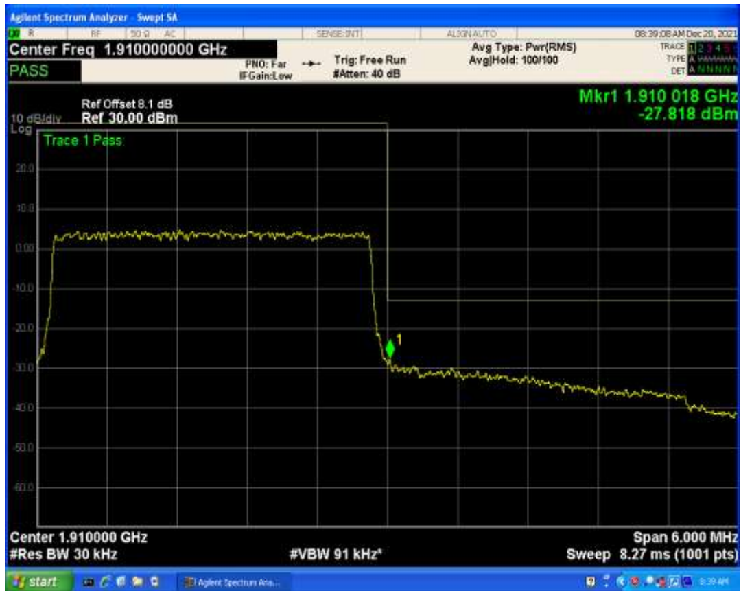
Band2 QPSK BW=5MHz Channel=18625 RB Size=1 Position=#0
