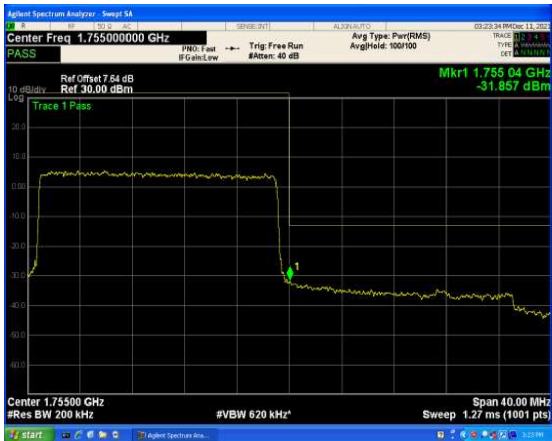
Band4 QAM16 BW=20MHz Channel=20300 RB Size=1 Position=#0
