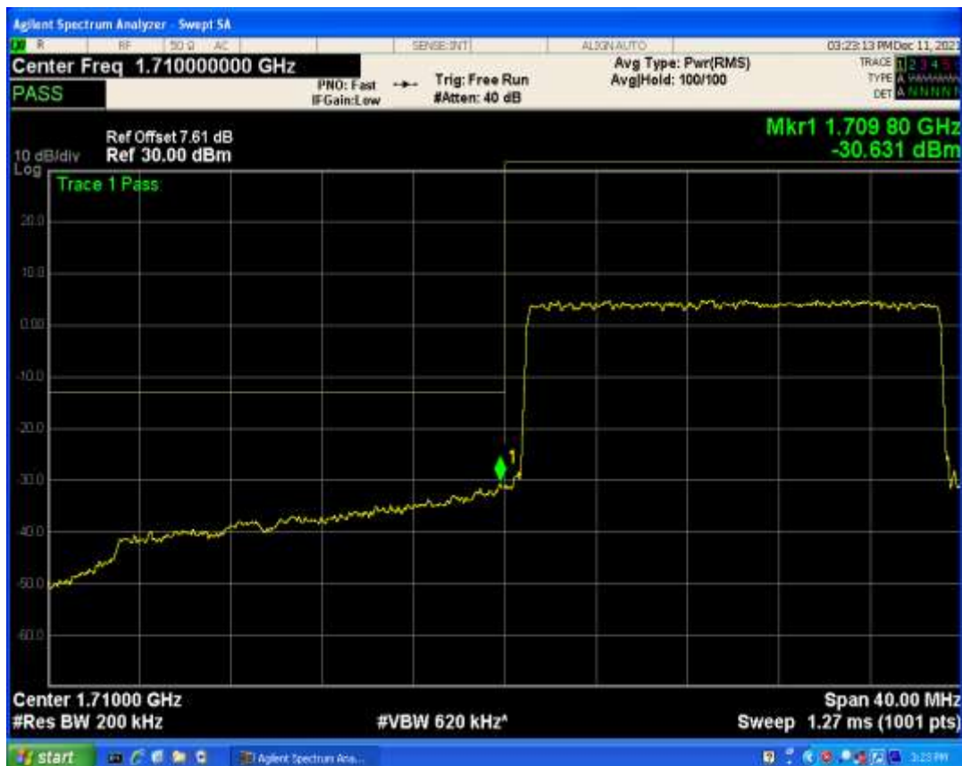
Band4 QAM16 BW=20MHz Channel=20050 RB Size=1 Position=#Max
