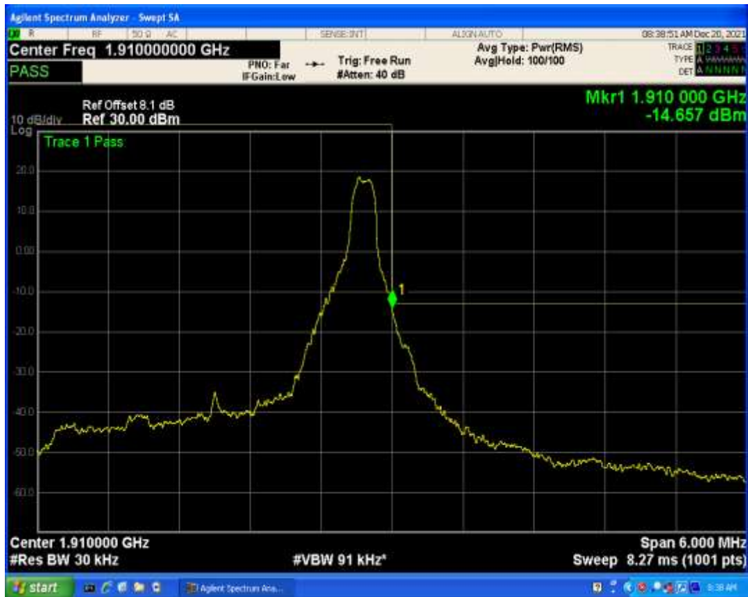
Band2 QAM16 BW=3MHz Channel=19185 RB Size=1 Position=#0
