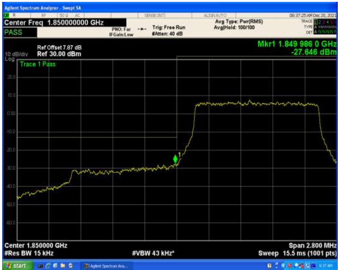
Band2 QAM16 BW=1.4MHz Channel=18607 RB Size=1 Position=#Max
