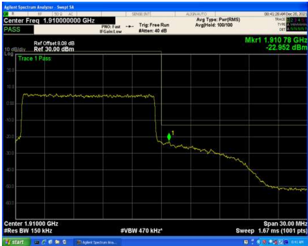
Band2 QAM16 BW=15MHz Channel=19125 RB Size=1 Position=#Max
