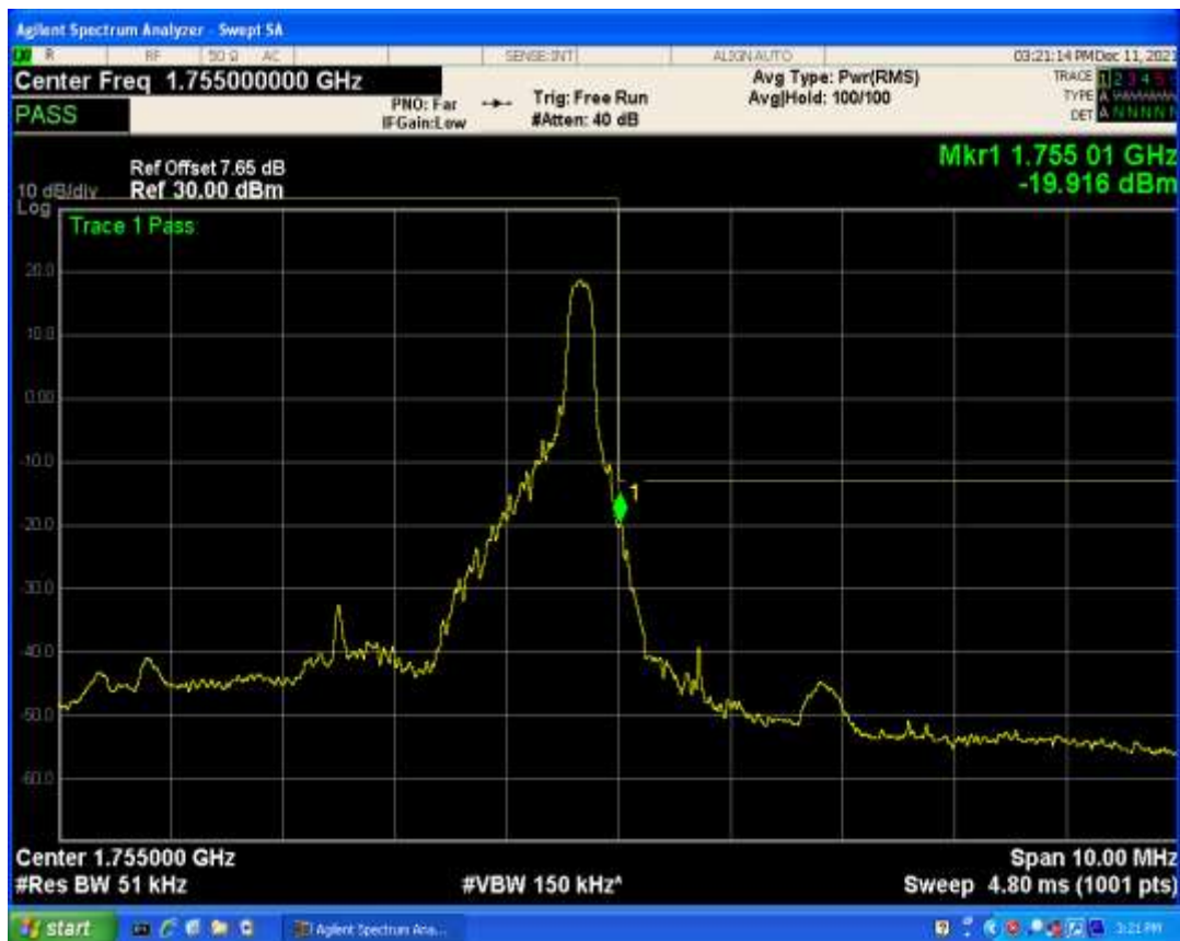
Band4 QPSK BW=10MHz Channel=20000 RB Size=1 Position=#0
