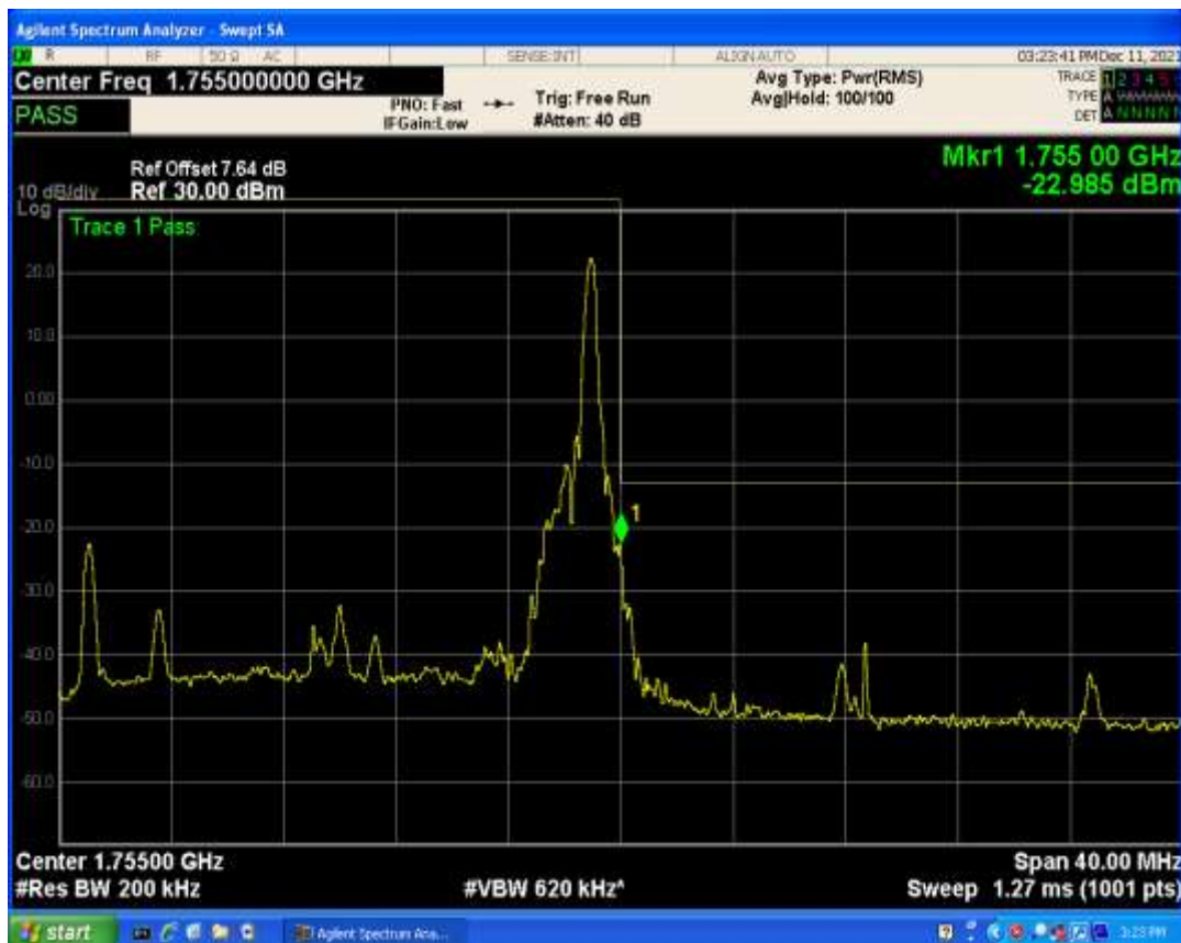
Band4 QAM16 BW=20MHz Channel=20300 RB Size=100 Position=#0
