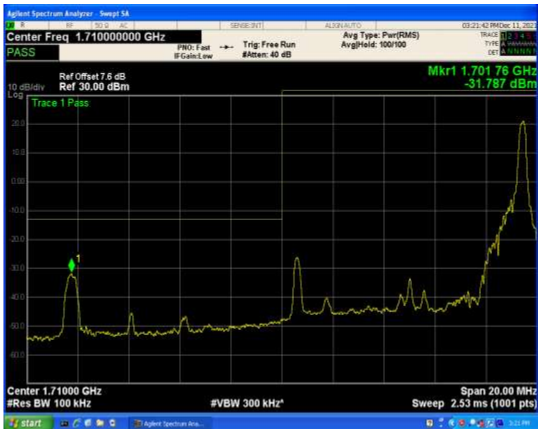
Band4 QPSK BW=10MHz Channel=20350 RB Size=1 Position=#0
