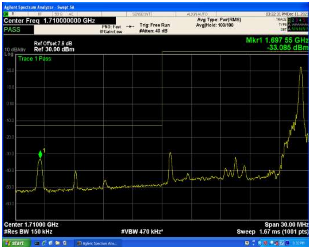
Band4 QAM16 BW=15MHz Channel=20025 RB Size=1 Position=#0
