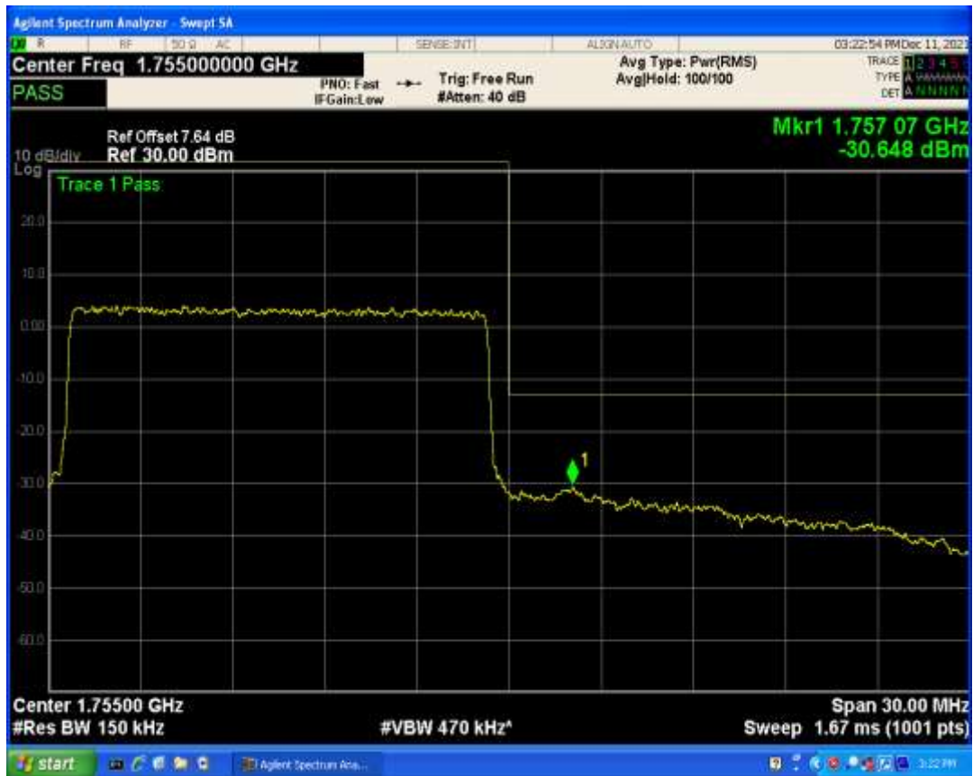
Band4 QPSK BW=20MHz Channel=20050 RB Size=1 Position=#Max
