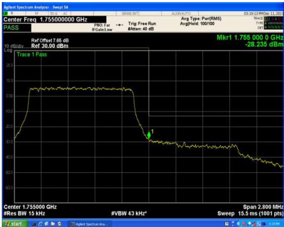
Band4 QAM16 BW=1.4MHz Channel=20393 RB Size=1 Position=#0
