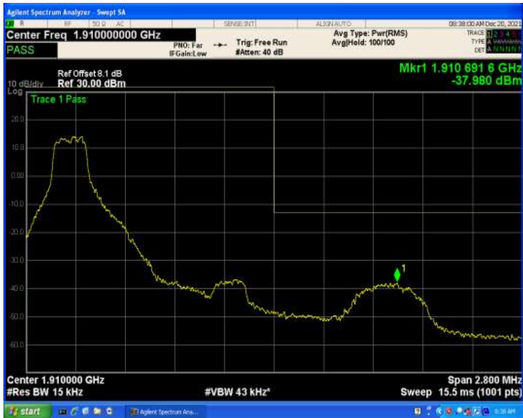
Band2 QAM16 BW=1.4MHz Channel=19193 RB Size=1 Position=#Max
