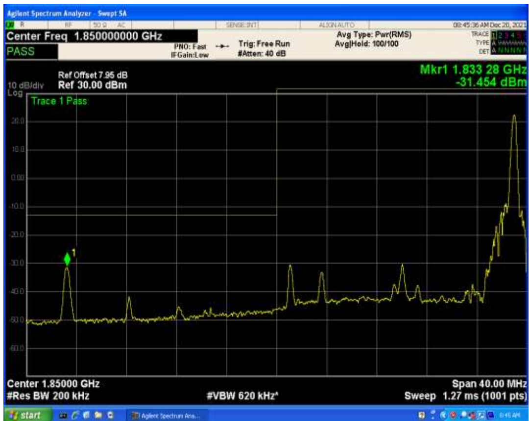
Band2 QPSK BW=20MHz Channel=19100 RB Size=1 Position=#0
