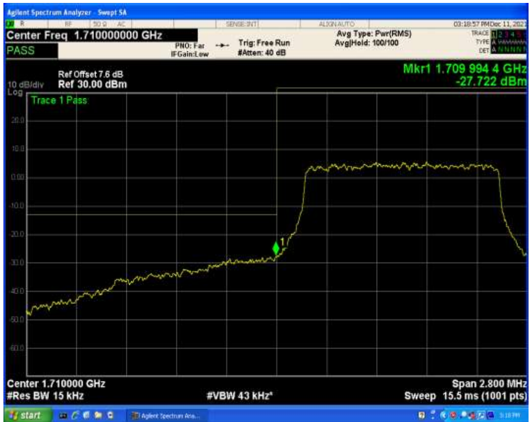
Band4 QPSK BW=1.4MHz Channel=20393 RB Size=1 Position=#0
