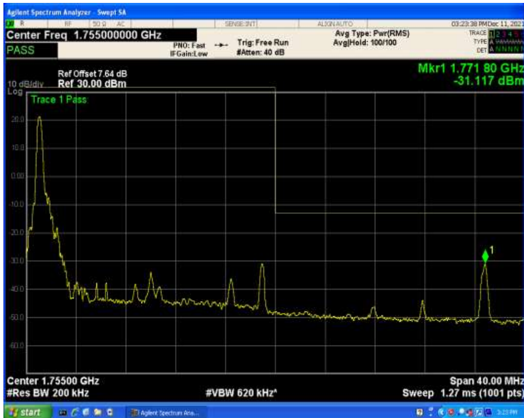
Band4 QAM16 BW=20MHz Channel=20300 RB Size=1 Position=#Max
