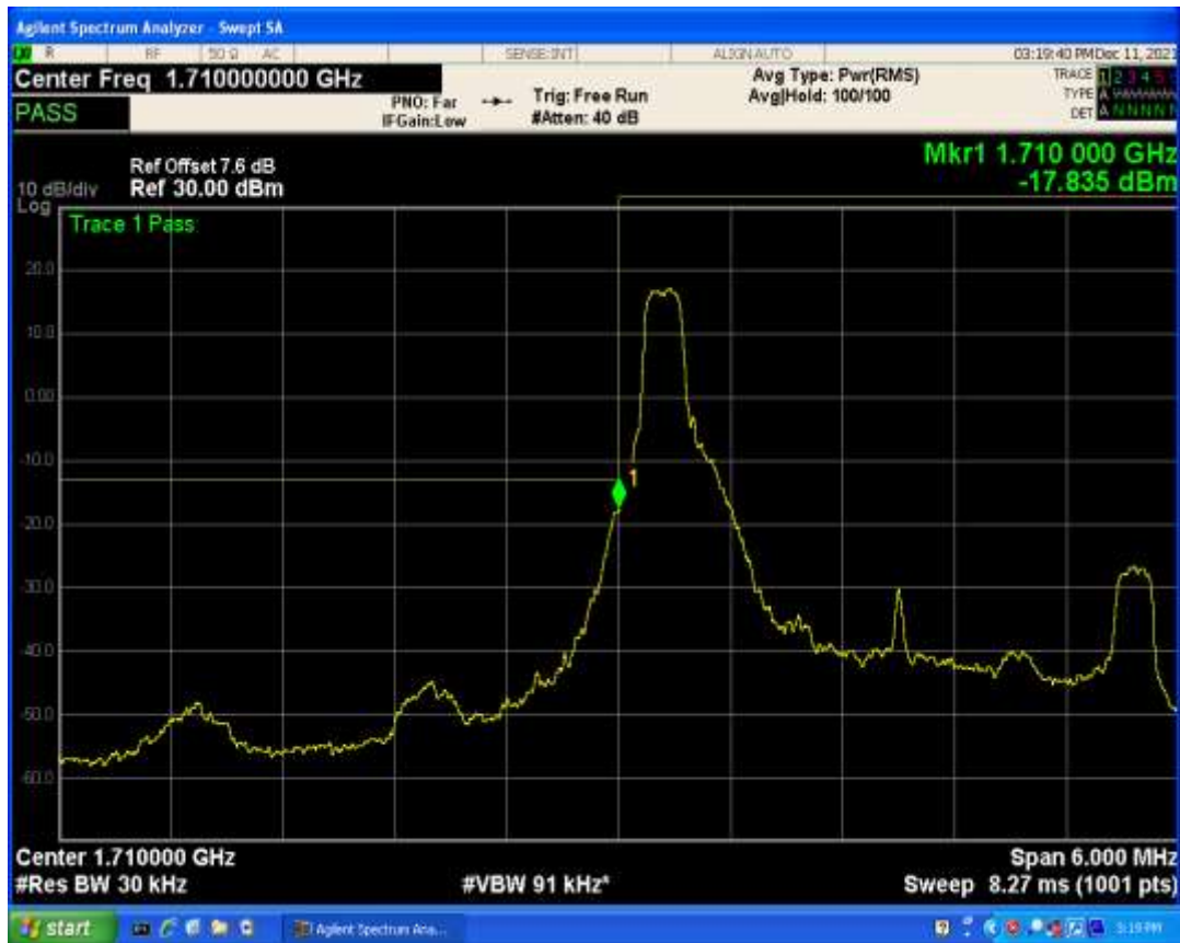
Band4 QPSK BW=3MHz Channel=19965 RB Size=15 Position=#0
