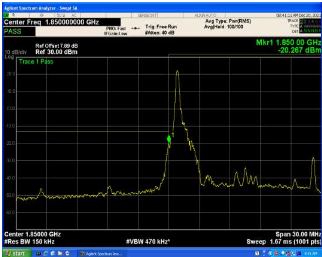
Band2 QPSK BW=15MHz Channel=18675 RB Size=75 Position=#0
