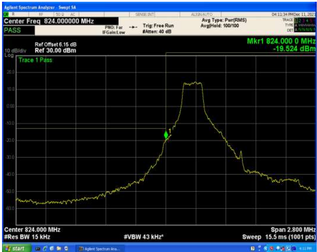
Band5 QPSK BW=1.4MHz Channel=20407 RB Size=6 Position=#0
