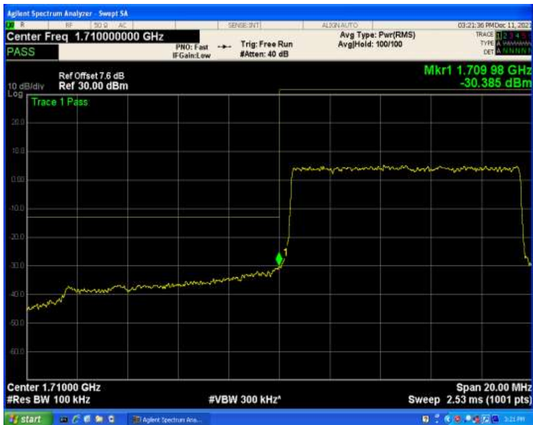
Band4 QAM16 BW=10MHz Channel=20000 RB Size=1 Position=#0
