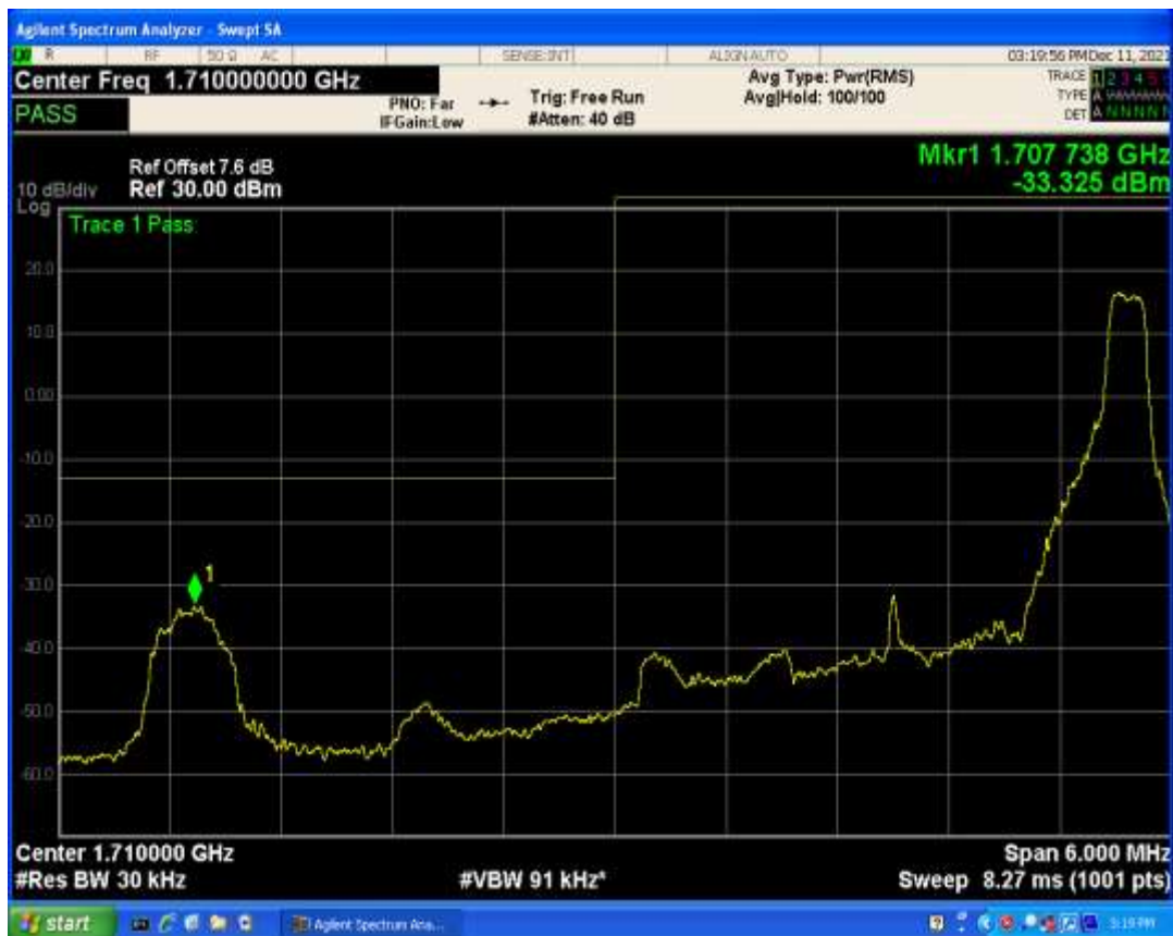
Band4 QAM16 BW=3MHz Channel=19965 RB Size=15 Position=#0
