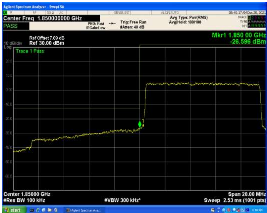
Band2 QAM16 BW=10MHz Channel=18650 RB Size=1 Position=#0
