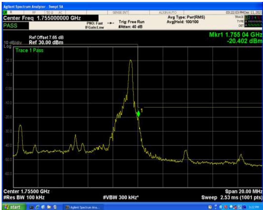
Band4 QAM16 BW=10MHz Channel=20350 RB Size=50 Position=#0
