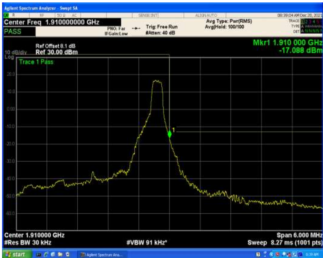
Band2 QAM16 BW=3MHz Channel=19185 RB Size=15 Position=#0
