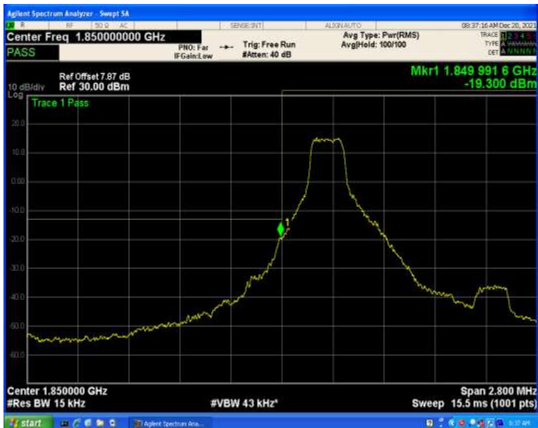
Band2 QPSK BW=1.4MHz Channel=18607 RB Size=1 Position=#Max
