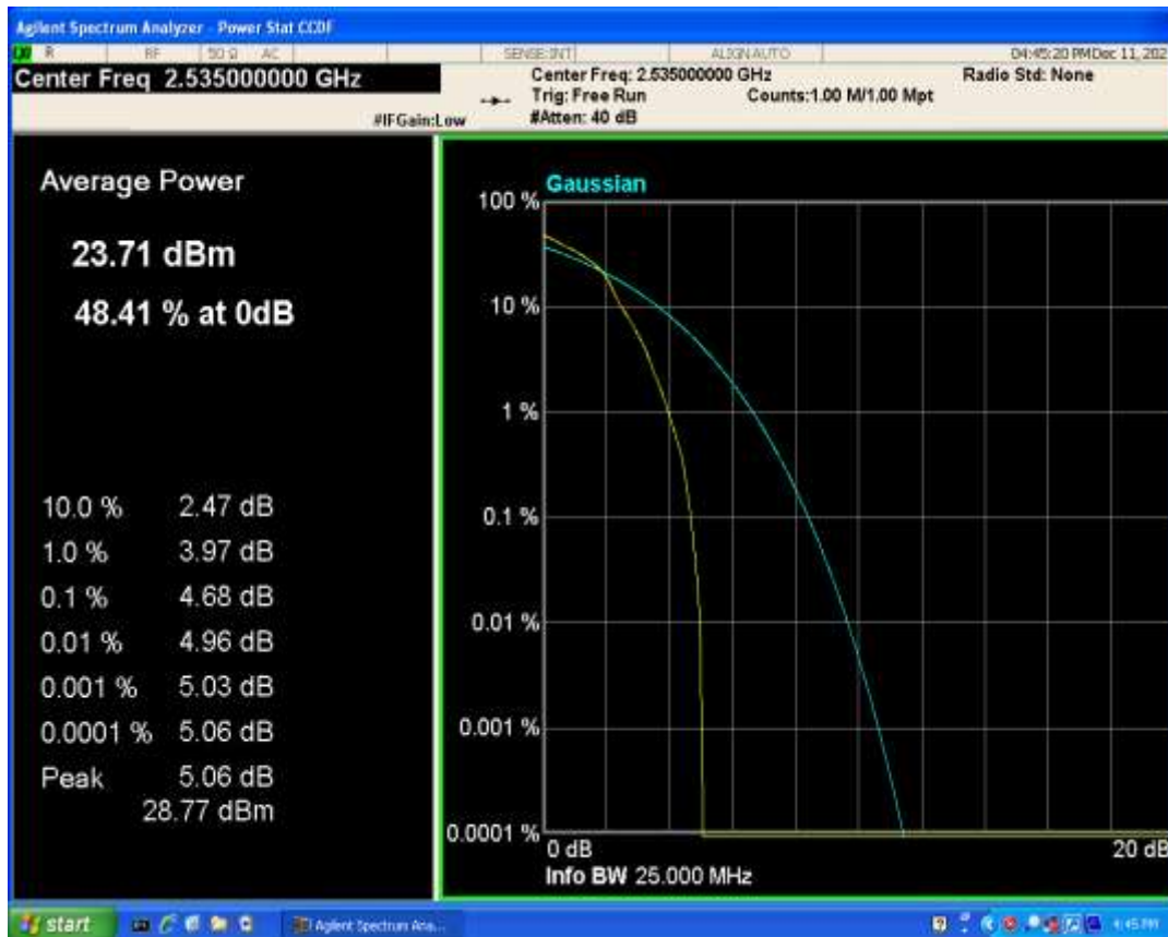
Band7 QPSK BW=10MHz Channel=21100 RB Size=1 Position=#0
