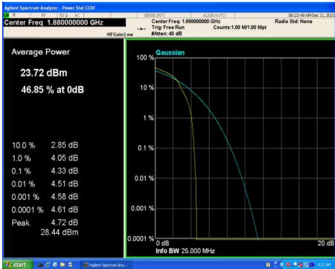
Band2 QPSK BW=20MHz Channel=18900 RB Size=1 Position=#0
