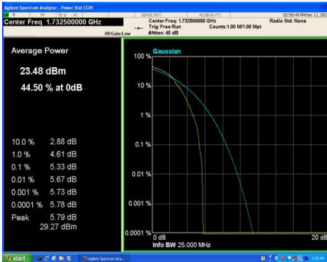
Band4 QPSK BW=10MHz Channel=20175 RB Size=1 Position=#0
