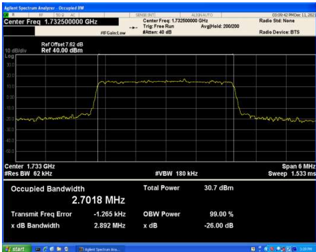
Band4 QPSK BW=3MHz Channel=20175 RB Size=15 Position=#0
