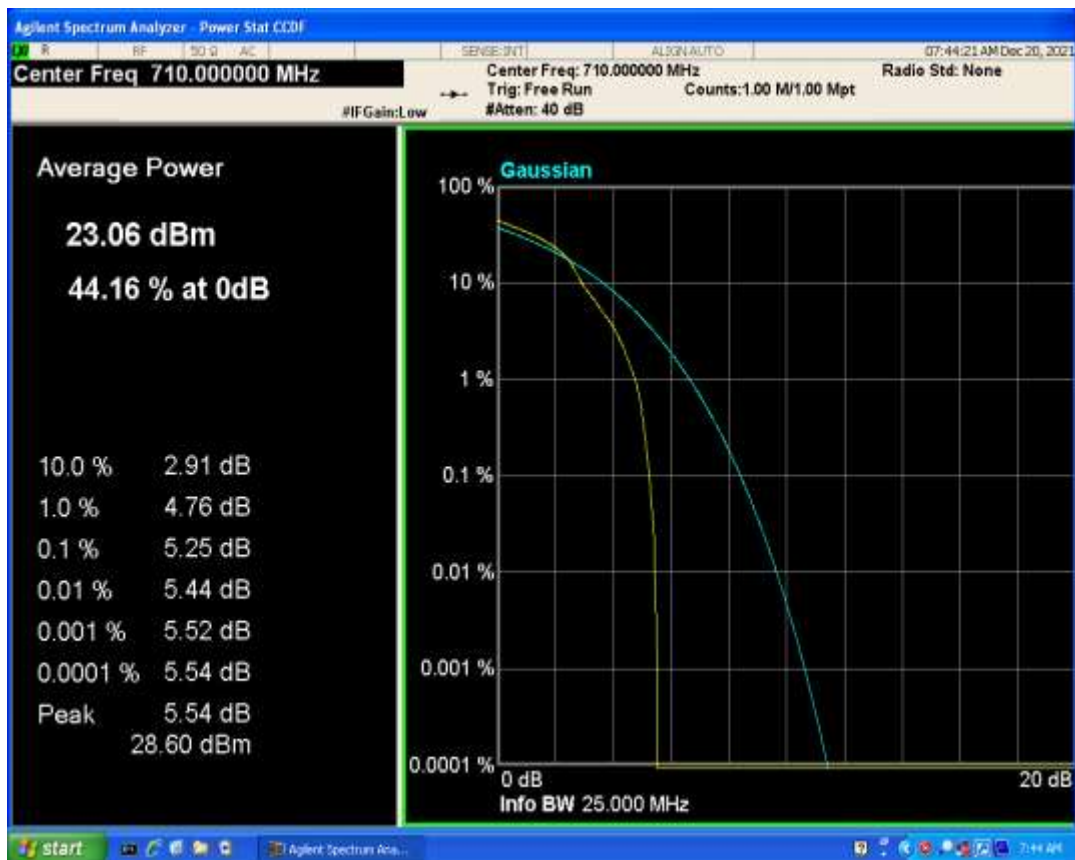
Band17 QPSK BW=10MHz Channel=23790 RB Size=1 Position=#0
