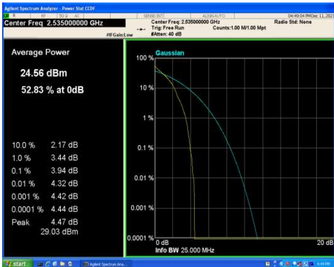
Band7 QAM16 BW=15MHz Channel=21100 RB Size=1 Position=#0
