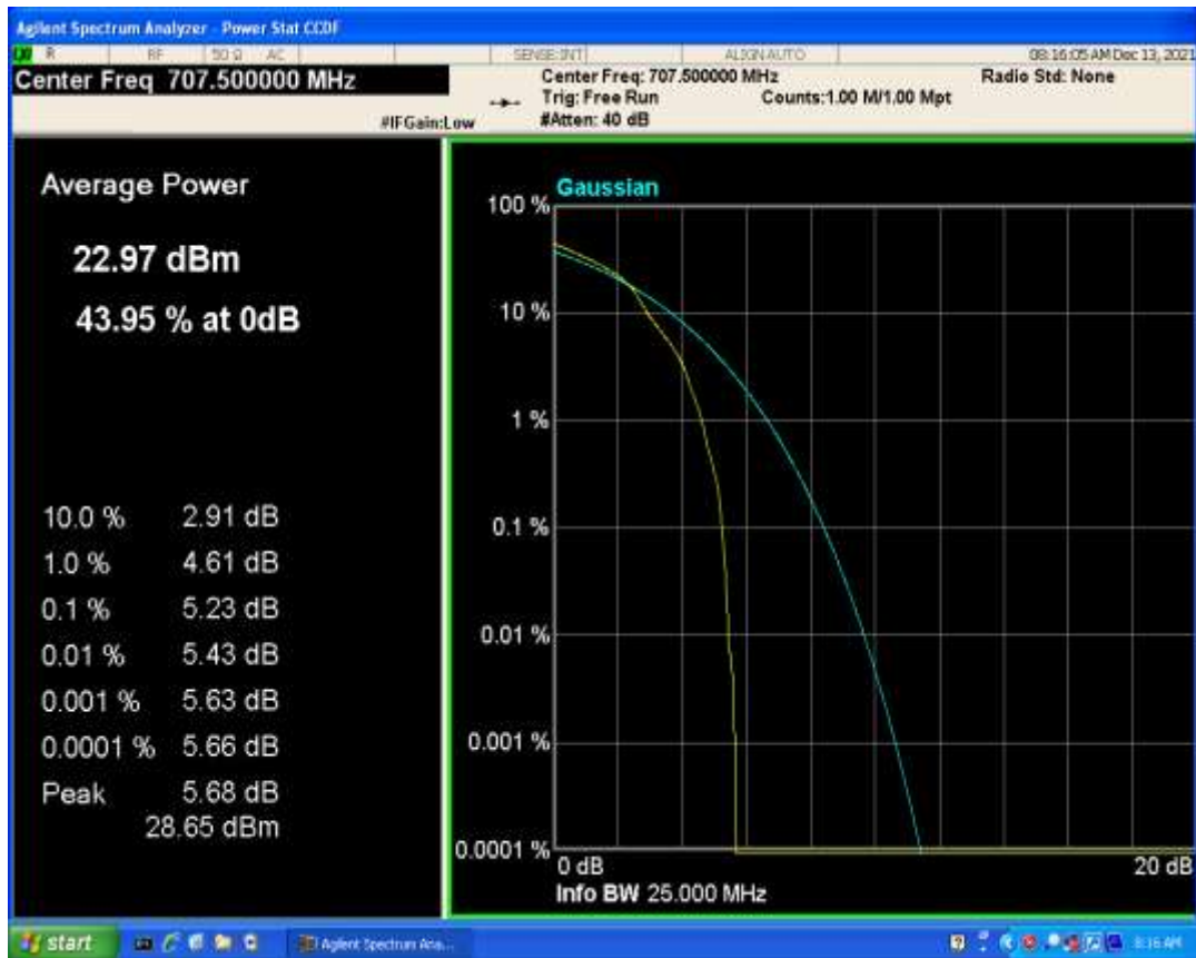
Band12 QPSK BW=10MHz Channel=23095 RB Size=1 Position=#0
