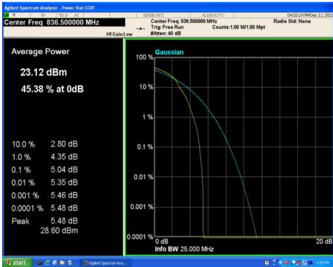
Band5 QPSK BW=10MHz Channel=20525 RB Size=1 Position=#0
