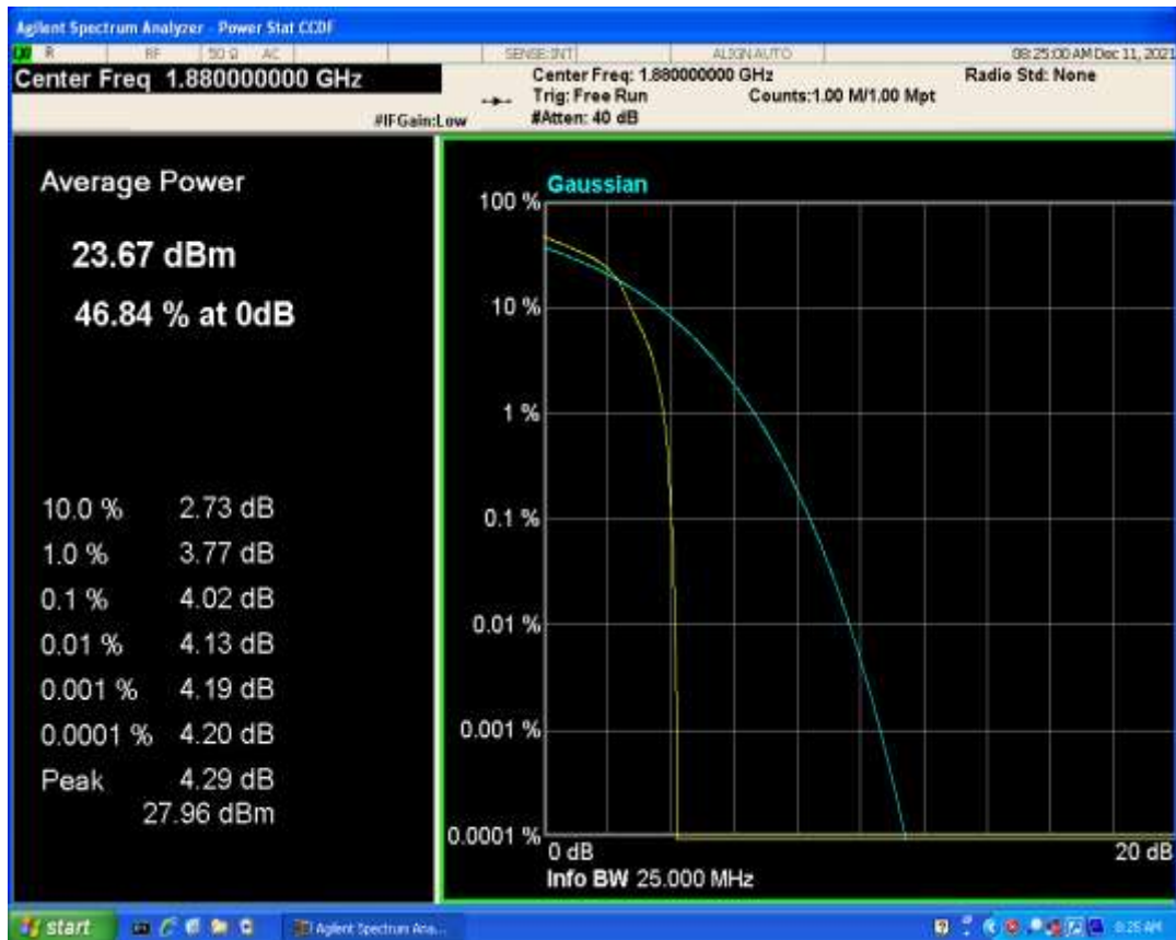
Band4 QPSK BW=1.4MHz Channel=20175 RB Size=1 Position=#0
