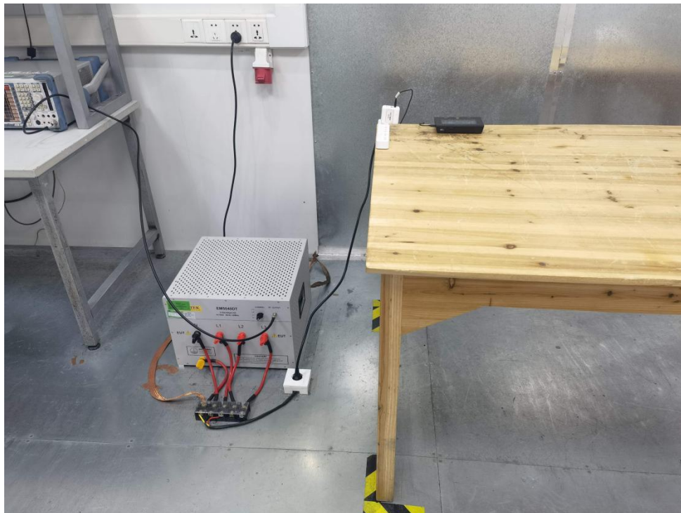
Photo of Conducted Emission Measurement
