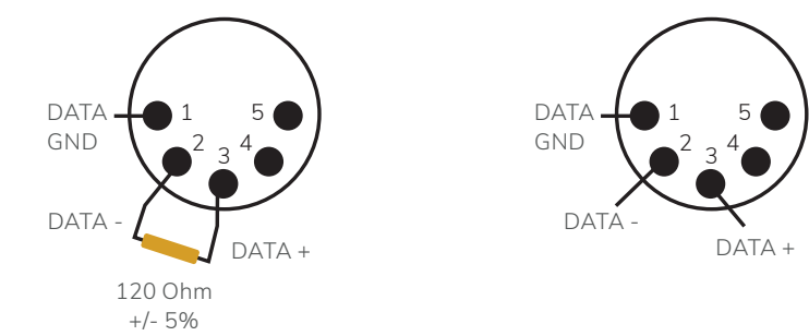
DMX Termination on last fixture DMX out
