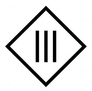
\*To identify equipment meeting the safety requirements specified for <u>claSS III</u> according to IEC 61140.
