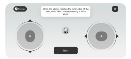
c. Click the {Next} button to save the connection line and enter the process of establishing a work zone.
