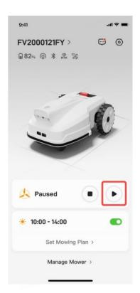
During the mowing process, if the battery is too low (below 20%), the robotic lawn mower will automatically stop mowing and return to recharge. Once the battery level reaches the resumed mowing threshold (default 80%), the robotic lawn mower will automatically return to the last mowing point and resume mowing operations.
