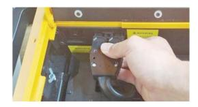
3. Plug the connector 1 (the one farther away from the connector 3) of the power adapter into the housing of the power station.
