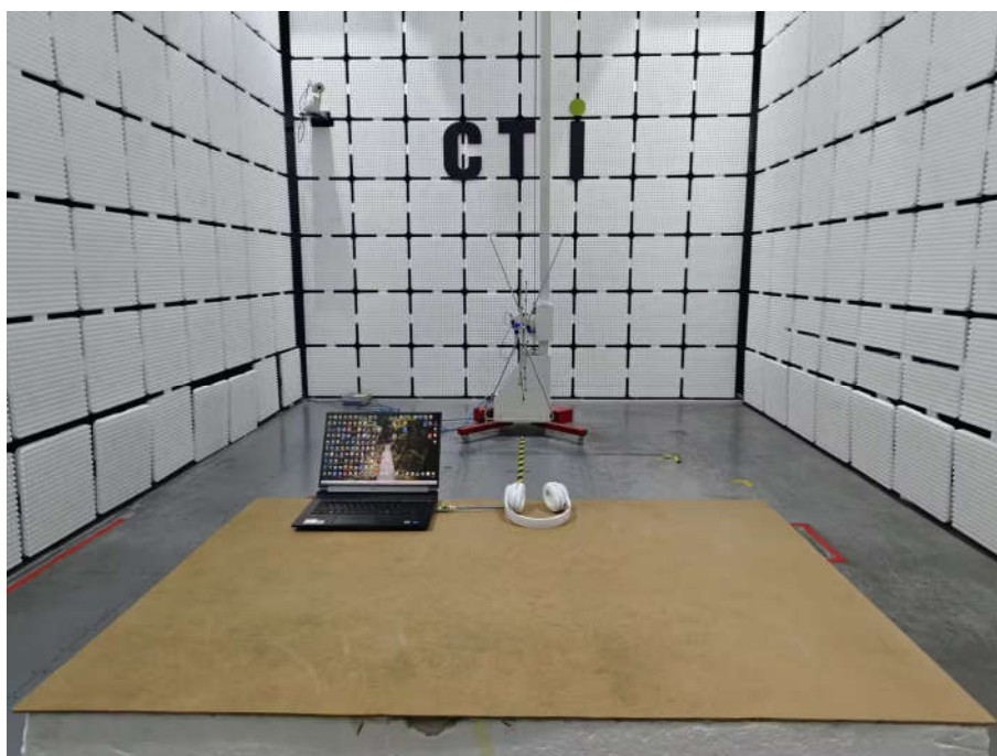
Radiated spurious emission Test Setup-1(Below 1GHz)
