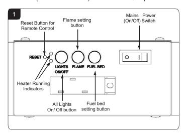
Note: The remote control will lose the memory for all function settings when the switch is set to the Off Position.
