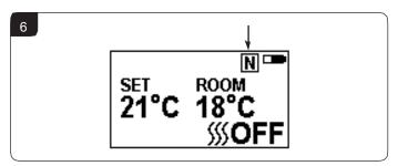
2b.12 Press the '+' or '-' button to adjust the setting temperature from 17 °C to 25°C.
