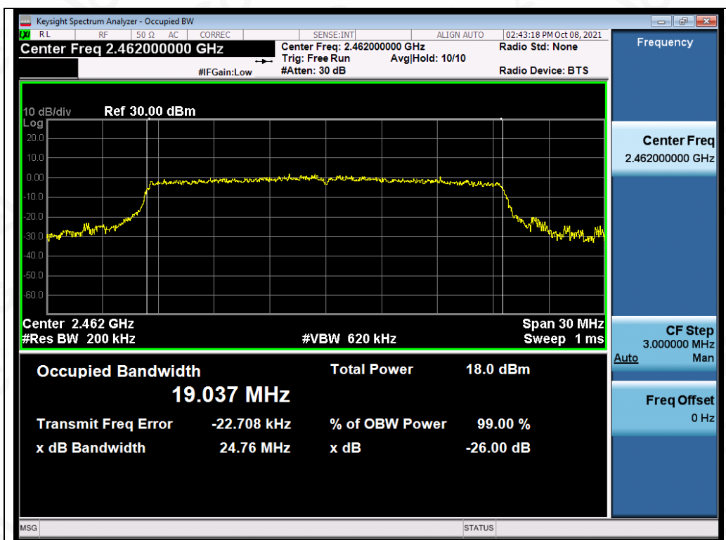
Test_Graph_802.11ax20_ANT1_2462_MCS0_OBW
