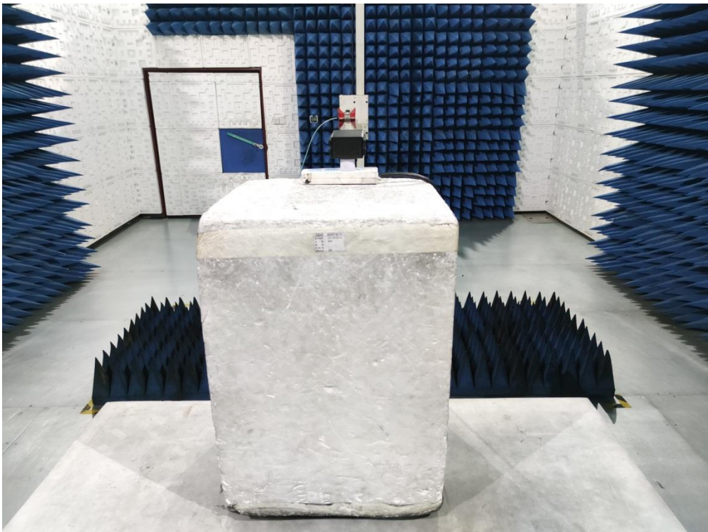
FCC RADIATED EMISSION TEST SETUP ABOVE 1GHZ
