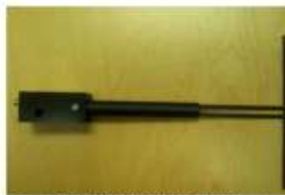
Figure 1 – MVG COMOSAR Validation Dipole
