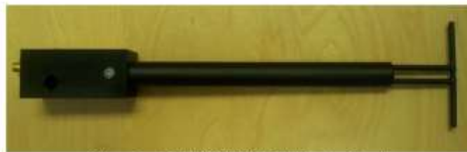
Figure 1 – MVG COMOSAR Validation Dipole
