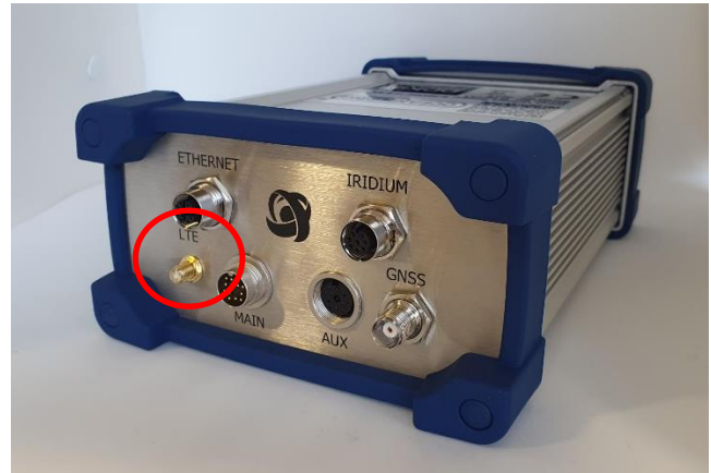
Figure 2 – Exterior of the unit showing LTE SMA bulkhead connector
