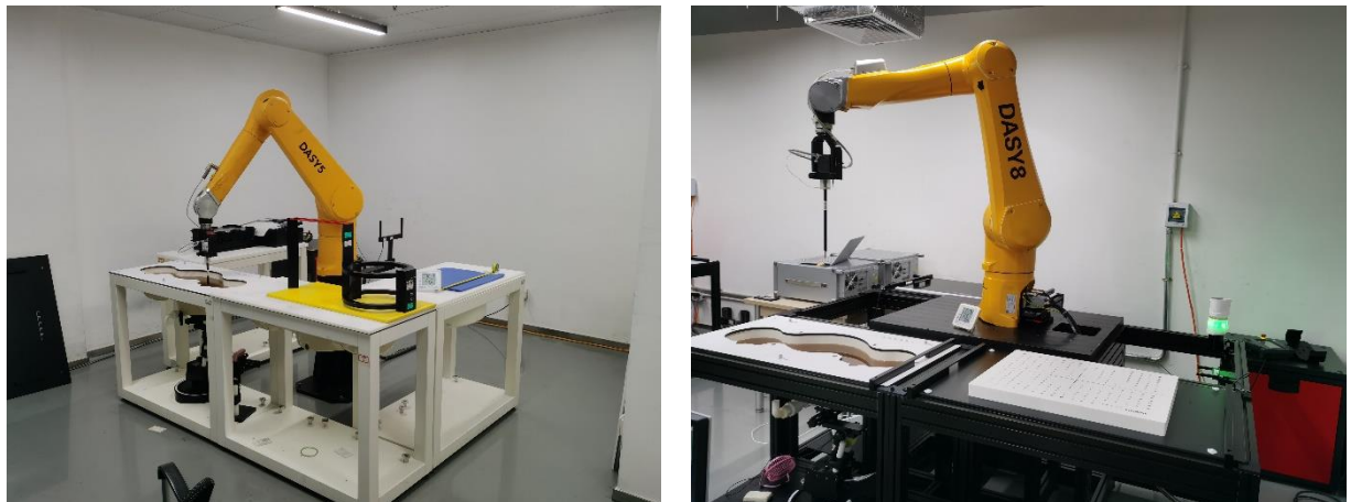
Picture D.6 Specific Absorption Rate Test Layout
